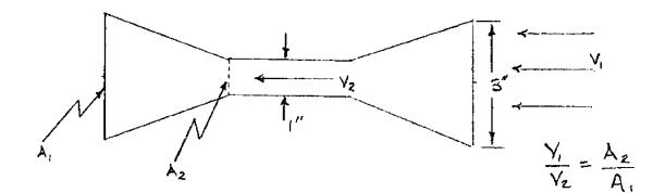
The velocity in the small tube varies as the inverse of the ratio of cross sectional areas, large (3" diameter) to small (1" diameter). This should make the unit very sensitive to changes in velocity of the surrounding medium.
