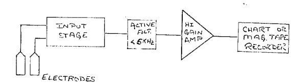
Figure 2: Block Diagram of the Amplifier Section
