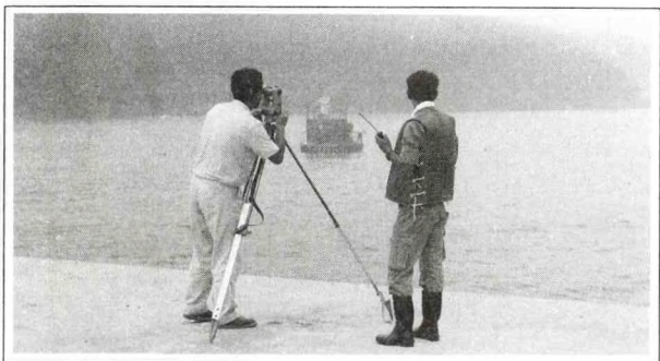
Figure 17. Measurement of anchors and artificial seafloor position.
