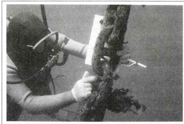
Figure 14. Measurement of chain diameter.
