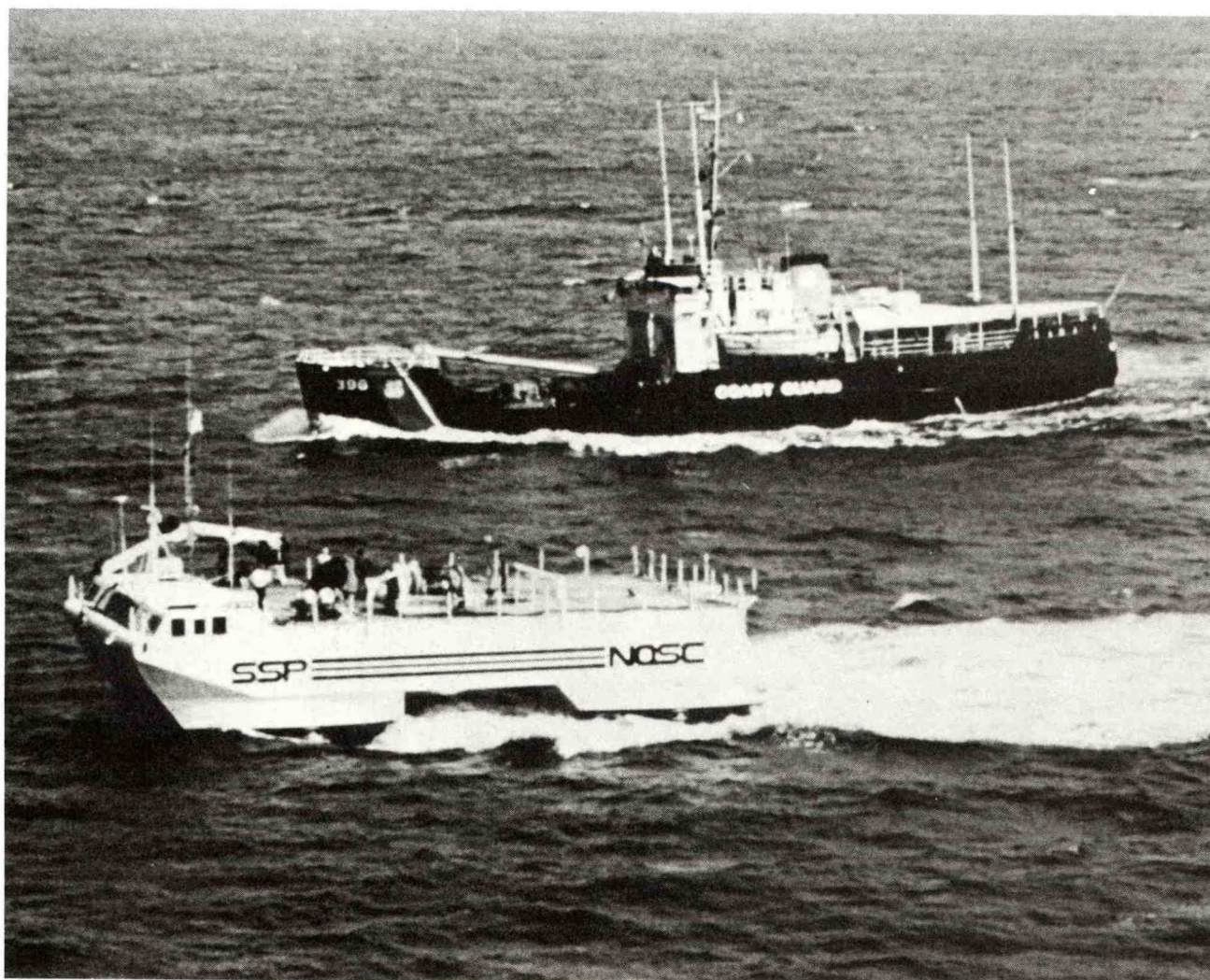
SIDE-BY-SIDE TRIALS OF SWATH KAIMALINO AND COAST GUARD BUOY TENDER.
