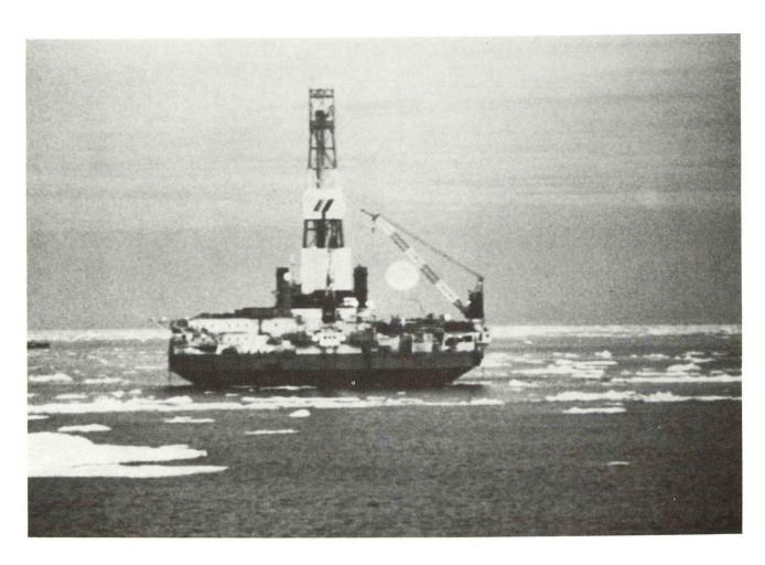
Figure 15. Beaudril Conical Drilling Unit (Kullur) at Amoco's Belcher wellsite.
