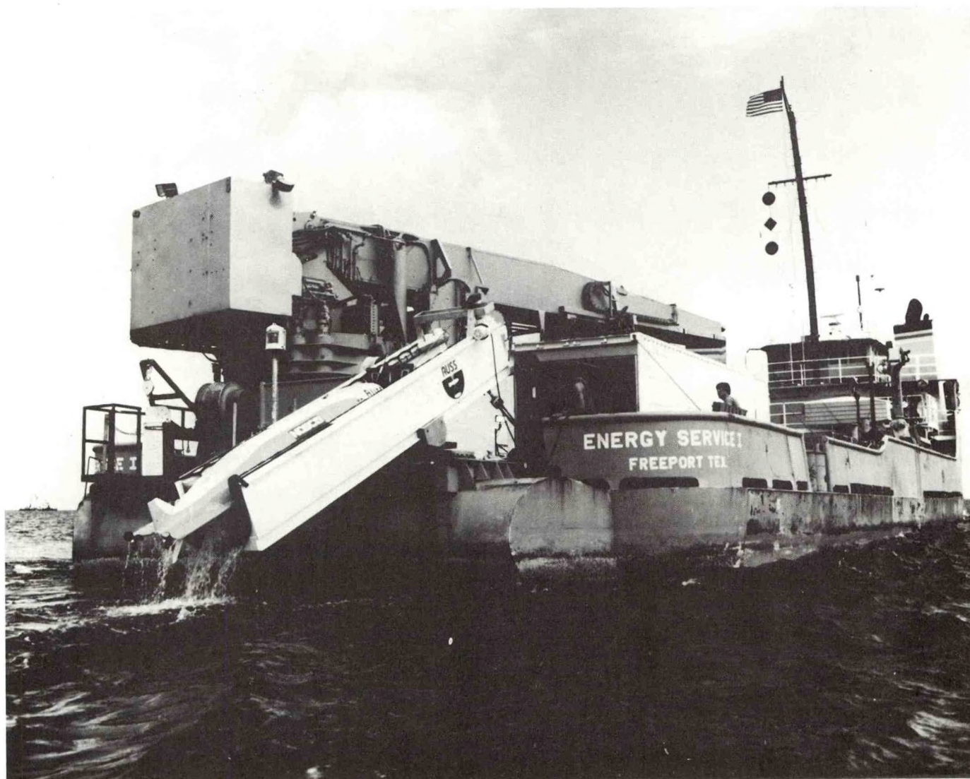
Figure 3. Retrieval of AUSS vehicle showing use of tiltable ramp
