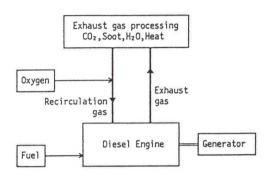
Fig.4-2 Principle of the CCDE
