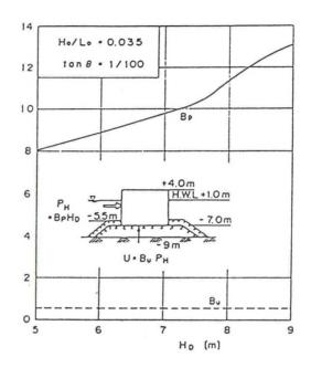
Fig. 3 Transfer coefficients of wave forces
