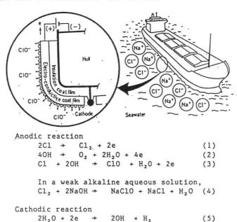
Fig. 1 Principle of marine growth prevention system by electro-conductive coating
