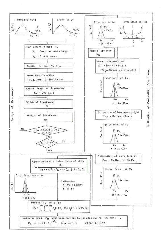
Fig. 5 Computation flow of probability of sliding failure of breakwater
