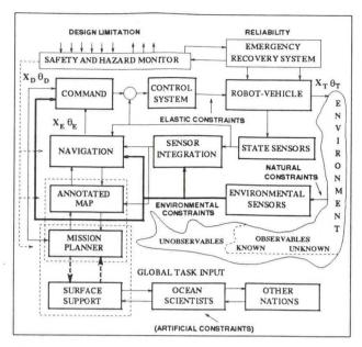
Figure 2: A possible black box wiring diagram showing the inter-connection of sub-systems for an underwater robot-submarine. The topology of these interconnections is only partially complete and accurate. For example, in other robot-system implementations the navigation subsystem is used to provide environmental sensors with positional information. This is done because when sensors make measurements the global location of the vehicle is used to "coordinate" them.
