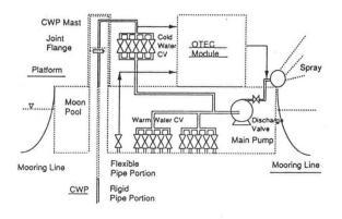
Fig.1 Concept of Experimental Facility
