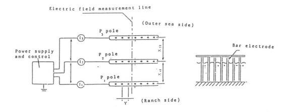
Fig. 4 "3 pole-2 potential method" electrical screen basic structure
