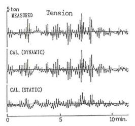
Fig.16 Time series of measured and simulated tensions
