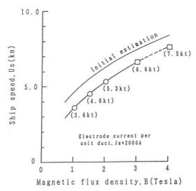
Fig. 11 Ship speed estimation
