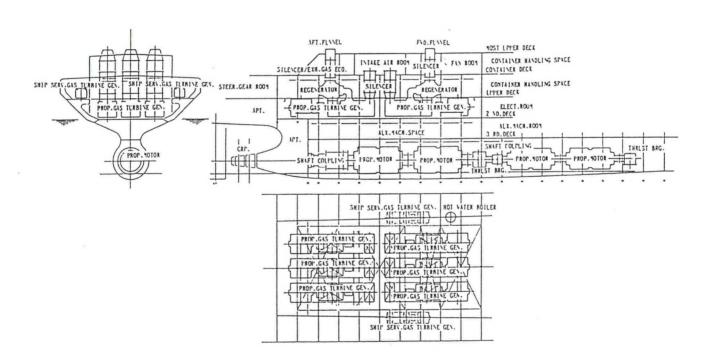
Fig. 10 Arrangement diagram of engine room
