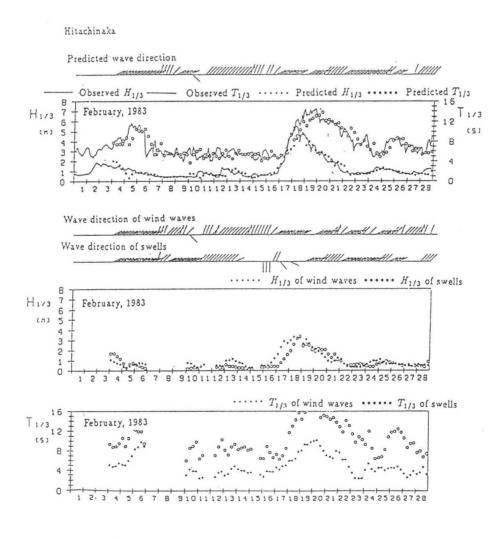
Figure 7 After 12 Hours Wave Forecasting Results at Port of Hitachinaka (Model B)
