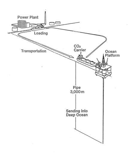
Fig. 2 Conceptual general view of transfer system of liquefied CO<sub>2</sub> into deep ocean
