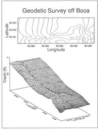
Figure 9: Geodetic survey off of Boca Raton Florida taken during March 1992. Location of each data point supplied from a Magnavox MX-200 GPS unit. Depths taken from output of the high resolution Chirp Sonar system. The distance between samples is 60 feet.
