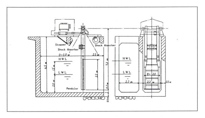
FIGURE 2. Pendulor System - 5 kW (hydraulic) prototype at Muroran Port.
