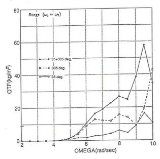
Fig. 6 Diagonal components of quadratic transfer function of surge mode
