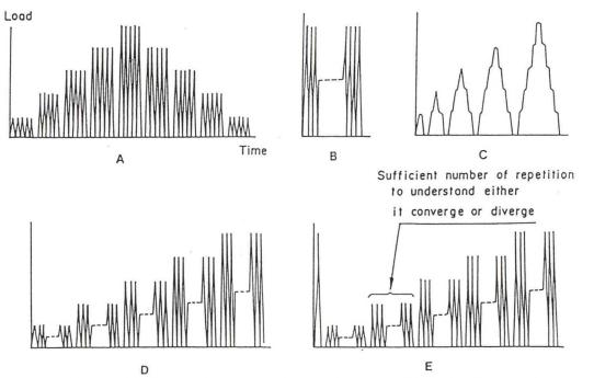
Fig. 5 Loading Patterns in Repeated Lateral Loading Experiments
