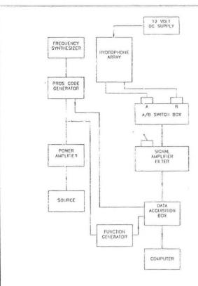
FIG. 1. P\*2S-tomography instrumentation system diagram.
