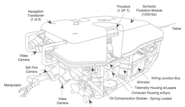
Figure 1. The Jason ROV performs scientific survey and sampling to depths of 6000 meters
