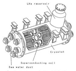
Fig. 3 Openview of the MHD thruster Fig. 4 Outside view of the right thruster
