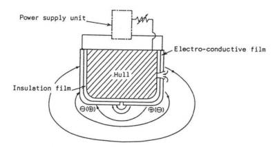
Fig. 7 Antifouling and anticorrosion system for ship's hull by electro-conductive coating
