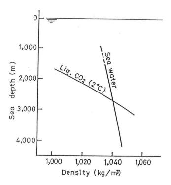
Fig. 7 Comparison of density between liquiefied  ${\rm CO_2}$  and seawater
