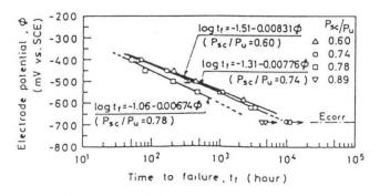
Fig. 11 Effect of electrode potential on time to failure [7]
