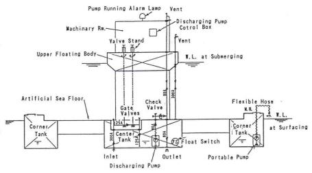
Fig. 5 Piping Diagram of the Ballasting System
