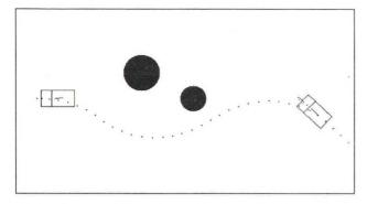
Figure 5: A fuzzy "style" algorithm that takes as its input the robot-vehicle's current position and heading and a goal position and heading and then "maps" the "difference" between them directly into actions for the controllers of motion and heading to act on. Unmapped objects are also avoided.
