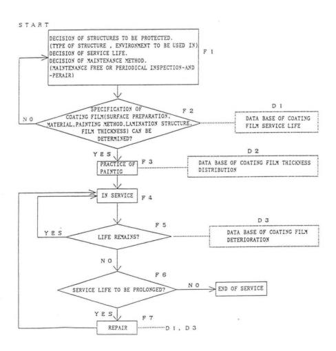
Fig. 7 Composition of corrosion preventing system of paint coating [5]
