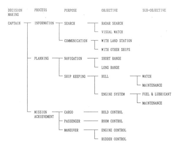
Fig. 1 An Example of Functional Hierarchy of Ship System
