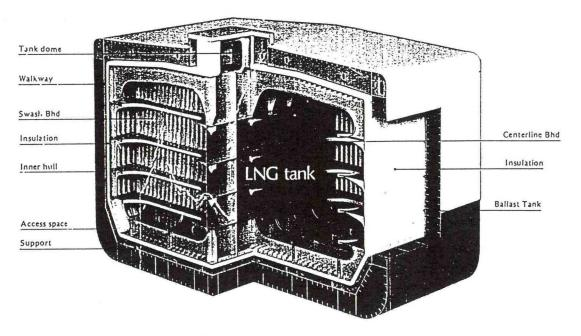
Fig.3 Structure of SPB Tank
