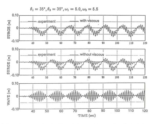
Fig.9 Comparison of time histories of surge in bi-chromatic waves ( $\theta 1=35^{\circ}$ ,  $\theta 2=35^{\circ}$ )
