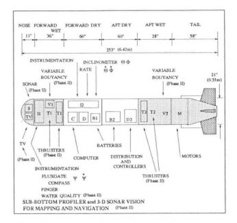
Figure 1: Schematic of FAU vehicle the Ocean Voyager.
