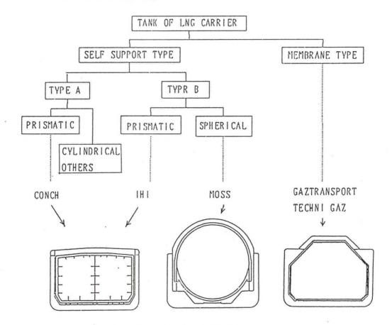
Fig. 2 Types of LNG Tank
