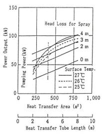
Fig.5 Self-sustaining Condition of Ocean-based Mariculture System "Houyou"
