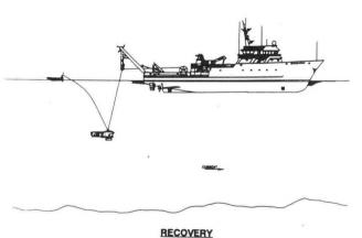
Submersible can now be winched to the surface. Buoy line slack is taken up by small book Figure 6
