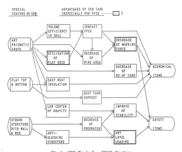
Fig.4 SPB Tank for FPSO System
