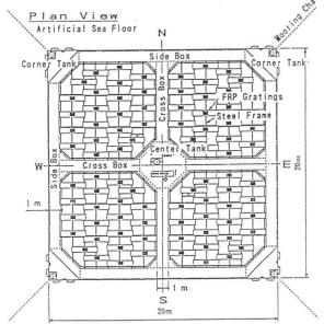
Fig. 2 General Arrangement of the Facility
