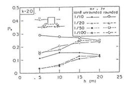
Fig. 13 Encounter probability of sliding failure of vertical breakwater
