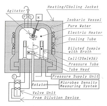
Fig. 4. Schematic Diagram of Isolation Device.
