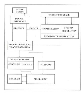
Figure 10: Organisation of a sonar interpreter for underwater robots.
