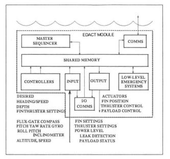
Figure 6: Communications layout for subsurface vehicle.
