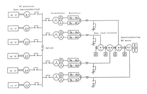
Fig. 8 Wiring diagrams of electric propulsion systems
