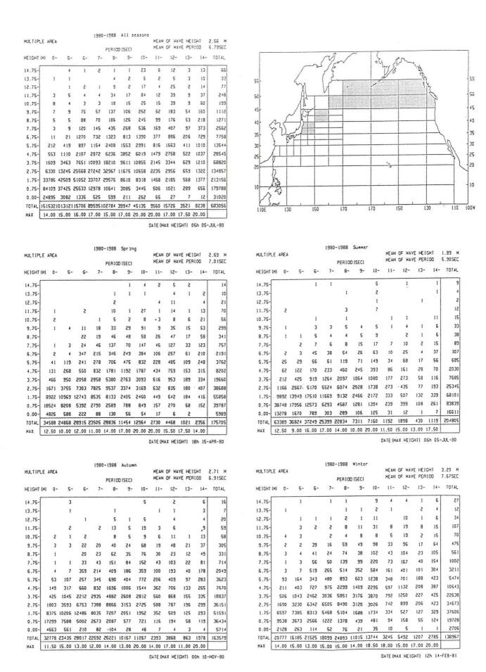
Fig.10 Scatter diagram of Wave Height and Period along Higher Latitude route
