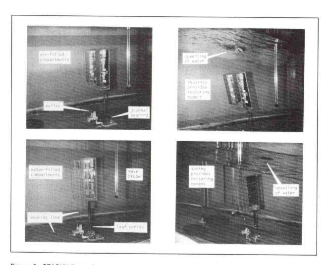
FIGURE 3. SEASUN Power Systems' wave energy absorber model in still water (left photos) and deflected seaward under a regular wave (right photos). Top photos are of Model 1, bottom photos of Model 2.
