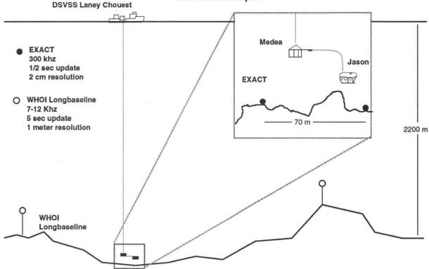
Figure 2. The precision survey required coordination of the dynamically positioned ship, the *Medea* vehicle and *Jason*. All vehicles were tracked with conventional long baseline navigation.
