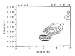
Figure 5 Example of the Observed Wave Directional Spectrum at the Iwaki Oki Station
