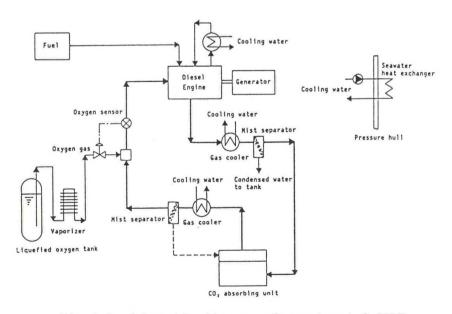
Fig.4-3 Schematic diagram of constructed CCDE
