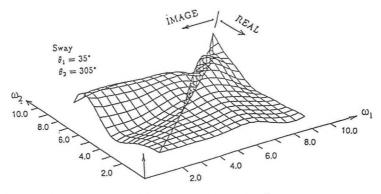
Fig.5 Quadratic transfer function of sway mode  $(\theta_1=35^\circ, \theta_2=305^\circ)$
