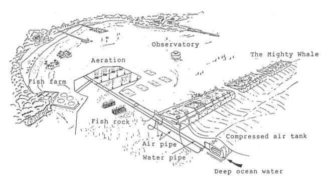
Fig. 5 A Future Plan of the Mighty Whale for the Offshore Utilization
