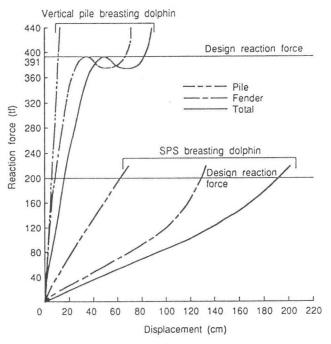
Fig. 3 Relationship between displacement and reaction force of the fender of vertical-pile and SPS breasting dolphins
