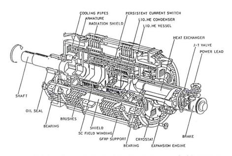
Fig.5 A bird's eye view of the 480kw superconducting motor
