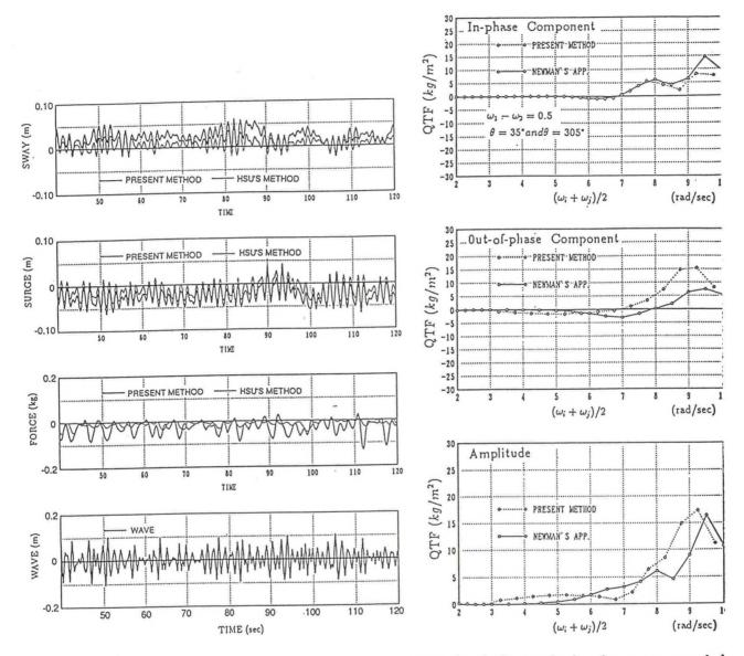
Fig.2 Comparison of time history of present method and Hsu's method
