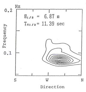
Fig.6 Directional wave spectrum
