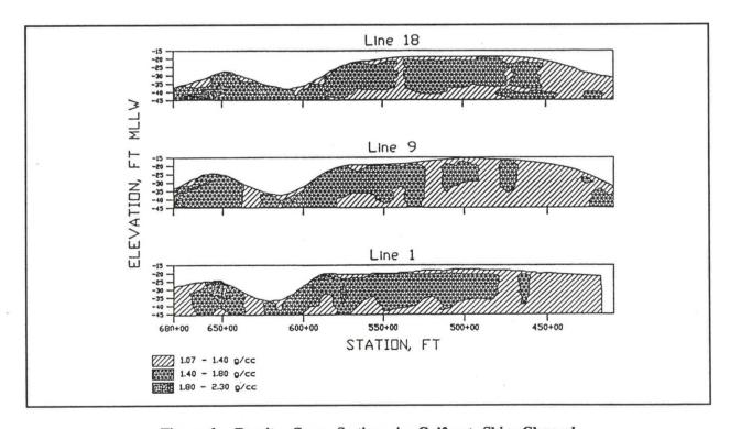
Figure 6. Density Cross Sections in Gulfport Ship Channel
