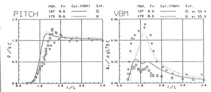
Fig. 4 Comparison with the conventional high speed vessel about pitch and vertical bending moment at high speed (F=0.60)
