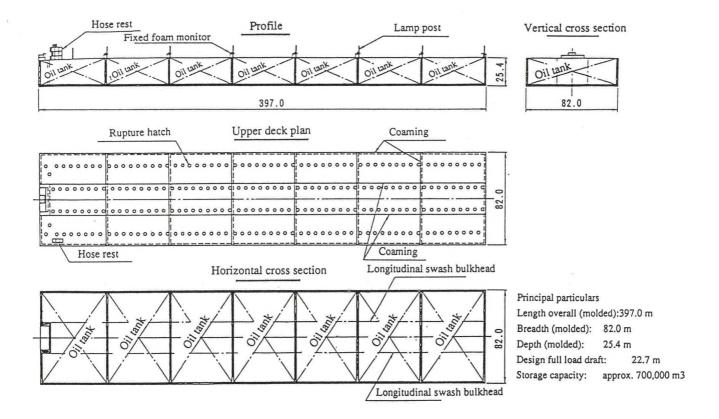
FIG.3 GENERAL ARRANGEMENT OF STOCKPILING VESSEL
