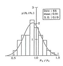
Fig. 8 Estimation error distribution of wave force on vertical breakwater
