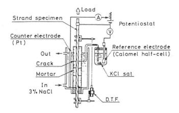
Fig. 10 Sketch of testing paratus of strand [7]
