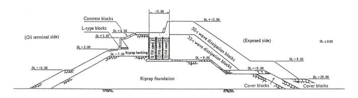
FIG. 6 PROFILE OF NORTH BREAKWATER
