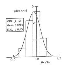
Fig. 7 Estimation error distribution of mild slope equation
