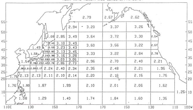
Fig.8 Mean Wave Height by Zones from Hindcast Data
