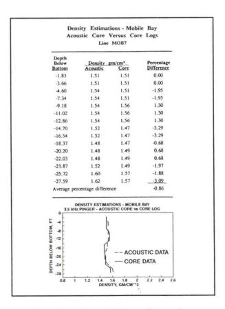
Figure 2. Ground Truth Comparison for Consolidated Sediments
