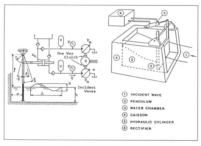
FIGURE 1. Pendulor System - concept and schematic diagram of rectifier.
