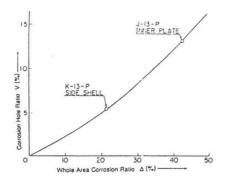
Fig. 1 Relation between whole area corrosion ratio  $\Delta$  and corrosion hole ratio [1]
