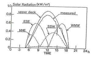
Fig.21 Total solar radiation for each surface wall
