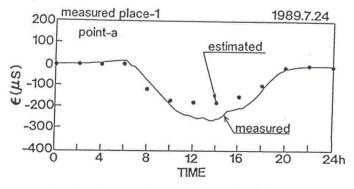
Fig.23 Comparison of strain between estimated and measured
