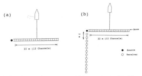
Fig. 1 (a) Schematic diagram of Kite system, (b) Kite system and conventional method ware performed to compare the results.
