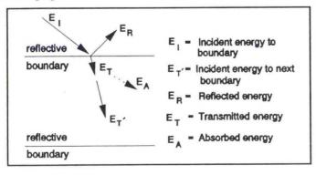
Figure 1. Energy Path Schematic
