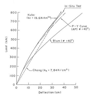
Fig. 4 Relationship between Load and Pile-Head Displacement (Lateral loading experiments of mock-up piles in hard sandy soil)
