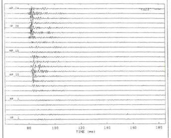
FIG. 2. Common source gather: source 22 m below surface in well-20, phone-1 at 49 m below surface, 24 at 3m in well-15, crosswell distance 122 m.
