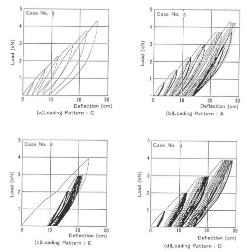
Fig. 6 Relationship Between Lateral Load and Pile-Head Displacement in Repeated Lateral Loading Experiments
