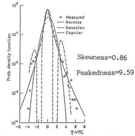
Fig.18 Instantaneous distribution of measured tensions
