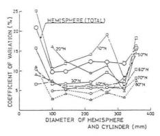
Fig. 5 Relation between diameter D and coefficient of variation  $\sigma/t_m$  for hemisphere [4]
