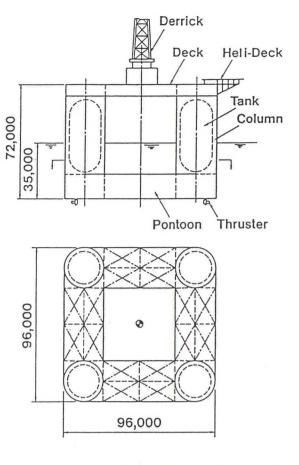
Fig. 5 Rough arrangement of ocean platform of semisubmersible type
