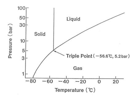
Fig. 3 CO<sub>2</sub> phase diagram
