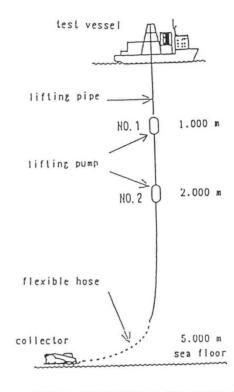
Fig. 1 GENERAL ARRANGEMENT OF THE MINING SYSTEM
