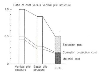
Fig. 2 Comparison of construction costs for a breasting dolphin
