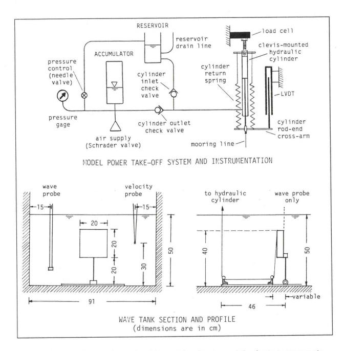
FIGURE 4. SEASUN Power Systems' model power take-off system and absorber test arrangements.
