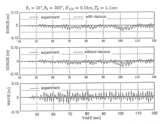
Fig.10 Comparison of time histories of surge in bi-directional waves ( $\theta$ 1=35°,  $\theta$ 2=305°)
