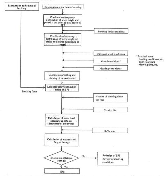
Fig. 7 Flowchart for examination of fatigue strength
