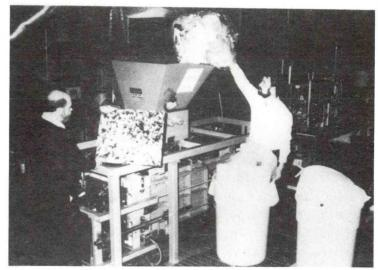
Figure 2. Prototype shipboard plastic waste processor.
