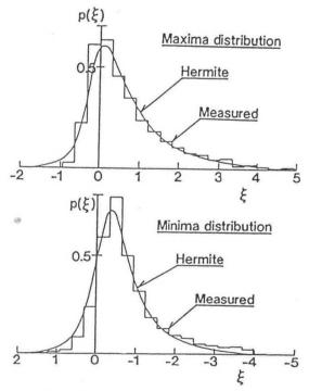
Fig.19 Minima and maxima distribution of measured tensions
