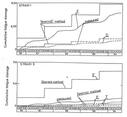
Fig.15 Cumulative fatigue damage in during field test
