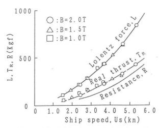
Fig. 10 Result of speed trials (2)
