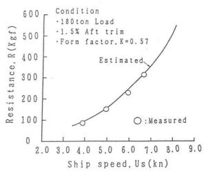
Fig. 9 Measured resistance of YAMATO-1
