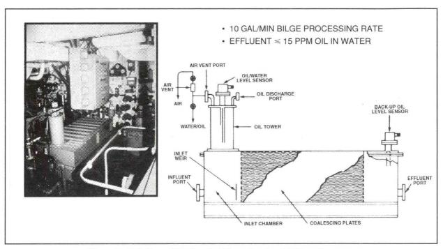
Figure 7. U.S. Navy 10NP Parallel Plate, Gravity, Oil/Water Separator
