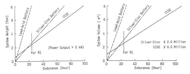
Fig.4-1 Comparison of Batteries and the CCDE
