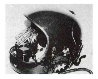
Figure 8. TOPS CVM Helmet Mounted Display.
