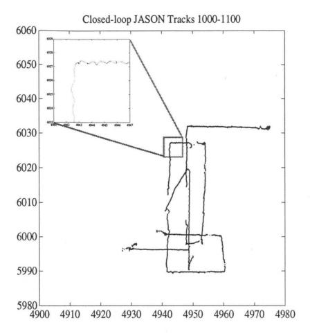
Figure 3. This plot shows *Jason* tracklines over a one hour period. The inset shows the control precision.
