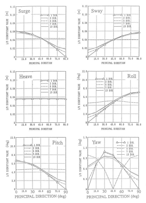
Fig.12 Significant values of motions for various principal directions and parameters of directional distribution function
