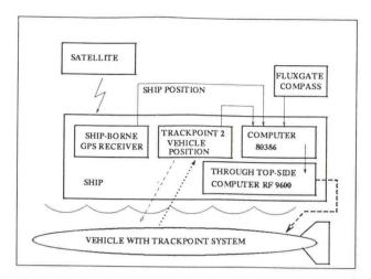
Figure 4: Development of Global Positioning System and Trackpoint to determine vehicle position.
