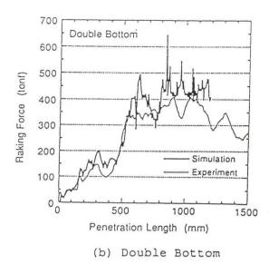
Fig.6 Raking Force vs. Penetration Length
