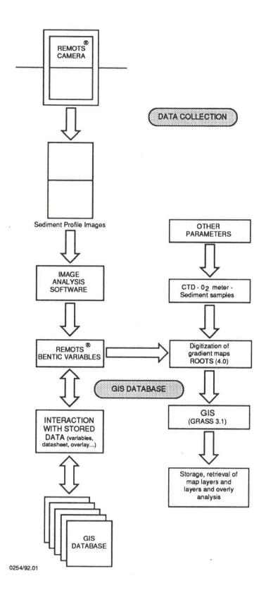
Figure 3. Protocol for pollution impact assessment: Integration of Image Analysis (REMOTS <sup>®</sup> technology) and GIS. Computer storage of REMOTS <sup>®</sup> benthic variables and GIS map layer allows the user to interactively retrieve and display information of interest.
