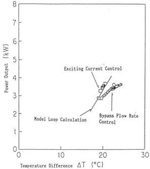
Fig.4 Characteristics of OTEC Power Output due to Two Types of Turbine Rotation Control Methods
