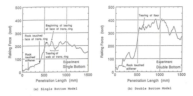
Fig.3 Raking Force vs. Penetration Length by the Experiments
