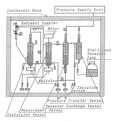
Fig. 3. Schematic Diagram of Dilution Device.
