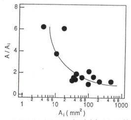
Fig. 9 Relation between visual defect area Ai of coating and real defect area A [6]
