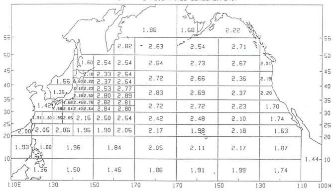
Fig.7 Mean Wave Height by Zones from Ship Data
