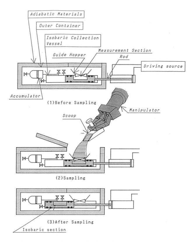
Fig. 2. Schematic Diagram of Sediment Sampling.
