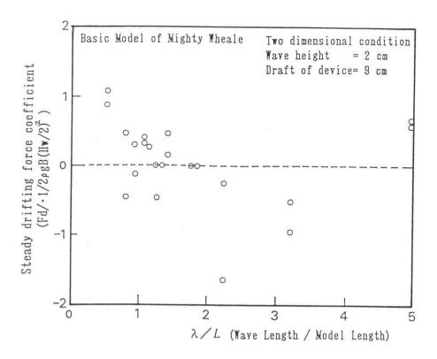
Fig.4 Experimental Results of Drifting Force
