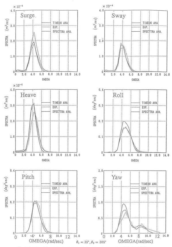
Fig.4 Spectra of first order motions in bi-directional waves ( $\theta1=35^{\circ}$ ,  $\theta2=305^{\circ}$ )
