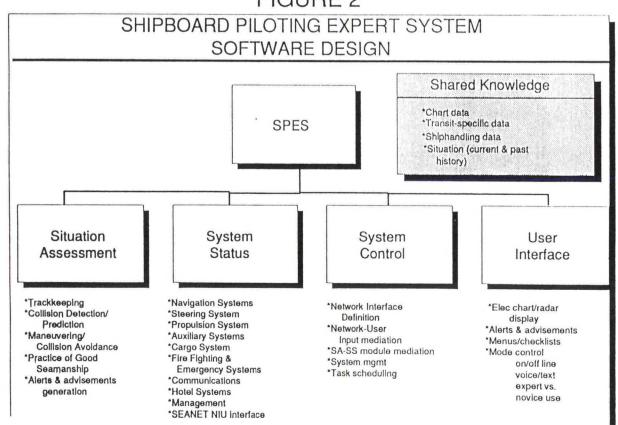
Situation Assessment Module - The Situation Assessment module houses the "expert" of the SPES. This module evaluates the piloting situation of your ship, assessing collision and grounding situations, required maneuvers, and generating action plans to resolve detected problems. This module uses chart knowledgebases as well as the maneuvering knowledgebase as part of the reasoning process.
