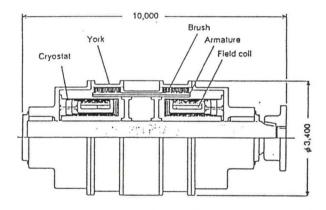
Fig.7 Superconducting D.C. homo-polar motor (21,000kw/120rpm)
