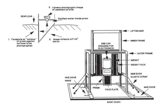
Figure 1(b). Principal elements of the REMOTS system.
