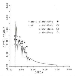
Fig.6 Comparison between Experiment(solid line) and Calculation(marks) of Pitch Transfer Function of the Platform
