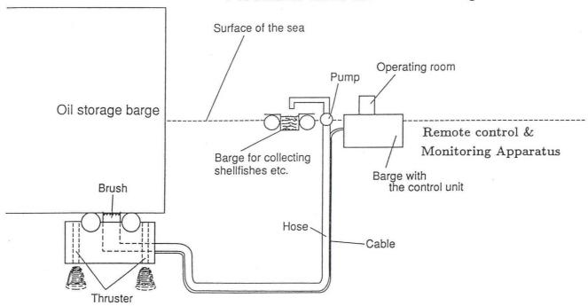
Figure 13 ROV and its Items under developing
