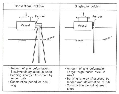
Fig. 1 Comparison of conventional dolphin with single-pile dolphin
