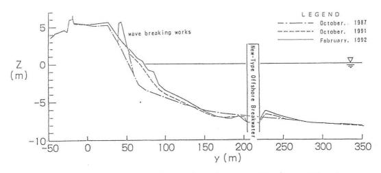
Fig. 6. Advance of shoreline due to the installation of slit-type offshore breakwater
