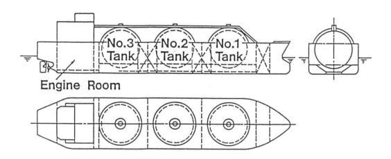
Fig. 4 Rough arrangement of CO<sub>2</sub> carrier
