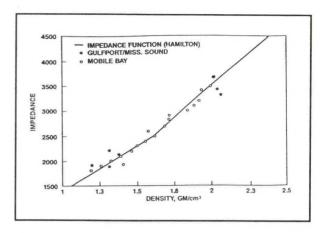
Figure 4. Computed Impedance Versus In-Situ Density Compared to Hamilton (1972)
