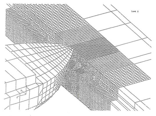
Fig.4 An Example of Simulation Model of the Ship Collision
