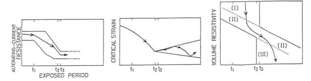
Fig. 3 Schematic view of deterioration phenomena of epoxy coating in an early stage [2]
