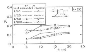
larger than those for the estimated Fig. 15 Encounter probability of sliding failure values by about 0.1. The probabilities of vertical slit caisson
