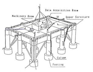
Fig. 3 Structure of POSEIDON
