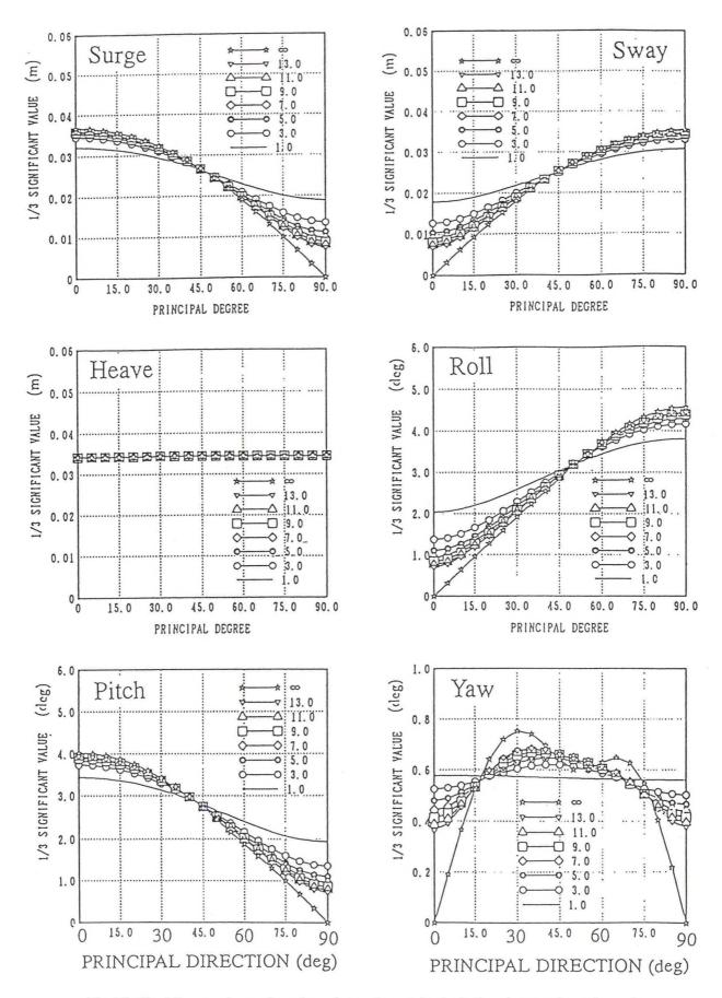
Fig.13 Significant values of motions for various principal directions and number of discrete wave directions
