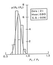
Fig. 9 Estimation error distribution of wave force on caisson covered with concrete blocks
