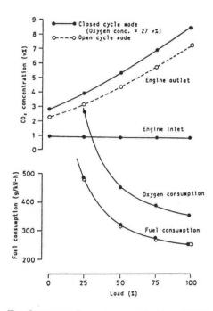
Fig.4-6 Engine performance of the CCDE
