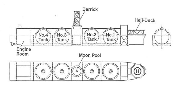
Fig. 6 Rough arrangement of ocean platform of ship type
