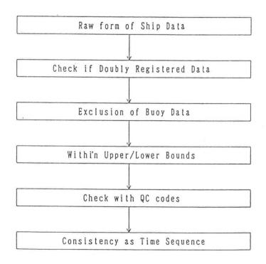
Fig.5 Checking Process of the Ship Data
