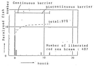
Fig. 8 interception performance by discontinuous barrier
