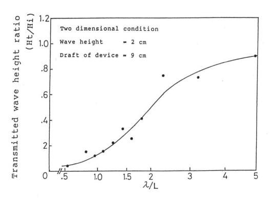
Fig.3 Performance of Dissipation of Incident Wave
