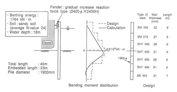
Fig. 8 Example of breasting dolphin design using SPS for 100,000 dwt tankers
