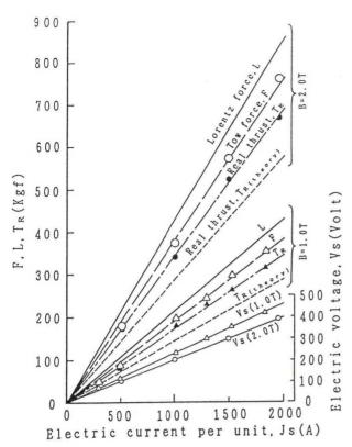
Fig. 6 Result of the bollard pull test
