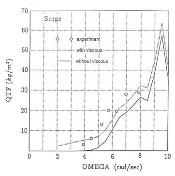
Fig.8 Quadratic transfer function of second order wave exciting force of surge mode ( $\theta$ =35°)
