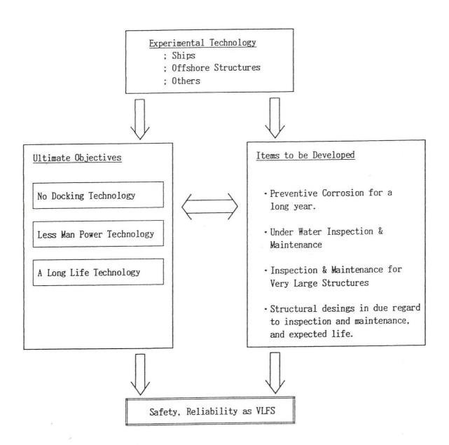
Figure 16 Concept for Inspection and Maintenance.
