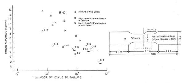
Fig. 2 Fatigue life diagram expressed by stress at section with minimum sectional area [1]
