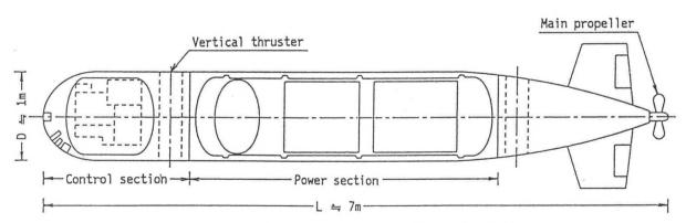
Fig.3-1 Conceptual drawing of the R1 robot
