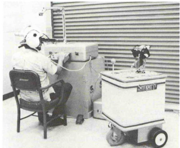
Figure 1. The Teleoperated Demonstration Device (TODD) vehicle shown to the right of the operator seated at the suitcase controller.
