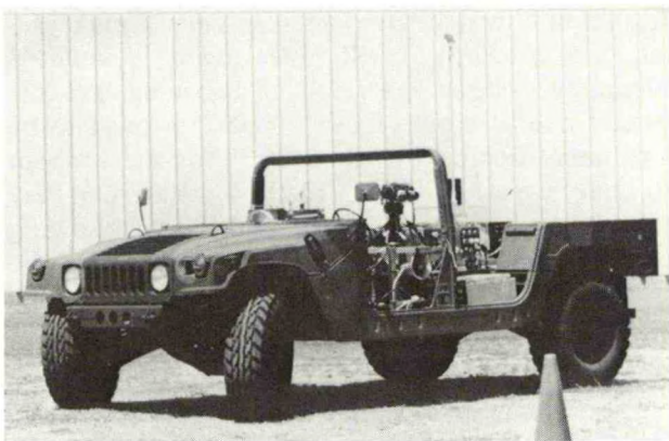
Figure 2. High-Mobility, Multi-Purpose Wheeled Vehicle (HMMWV) with the telepresence system installed.
