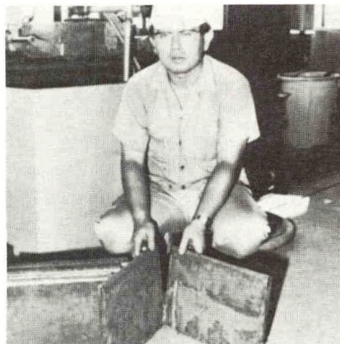
Underwater Cutting of 300 mm (11.8 inch) Thick Stainless-Clad Steel
