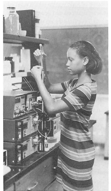
A graduate student separates chemical metabolites from marine organisms using high-performance liquid chromatography. Photo: Delaware Sea Grant
