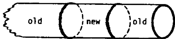
f. REPLACING A SECTION OF A PIPE
