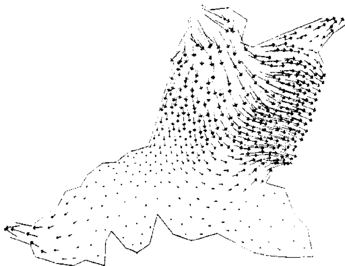
Fig. 4: Computed tidal current vectors for existing bathymetry (NOS hydrographic chart No. 12327, 70th Ed., July 1977) for maximum ebb at Sandy Hook. After Wong and Wilson (1979).
