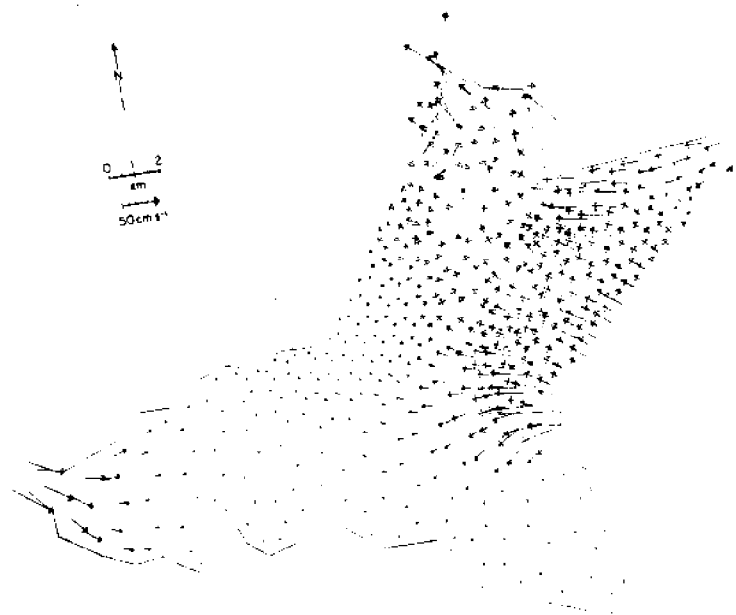
Fig. 5: Computed tidal current vectors for existing bathymetry (NOS hydrographic chart No. 12327, 70th Ed., July 1977) for maximum flood at Sandy Hook. After Wong and Wilson (1979).
