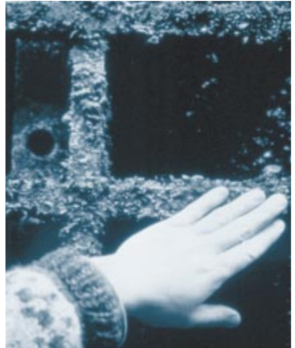
Zebra mussels have become a foulant for inland navigation by settling in towboat sea chests and keel coolers.
