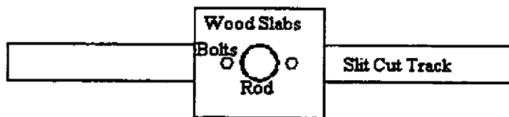
Figure 5-7b. Side view of mounts used to keep steel rods in place.
