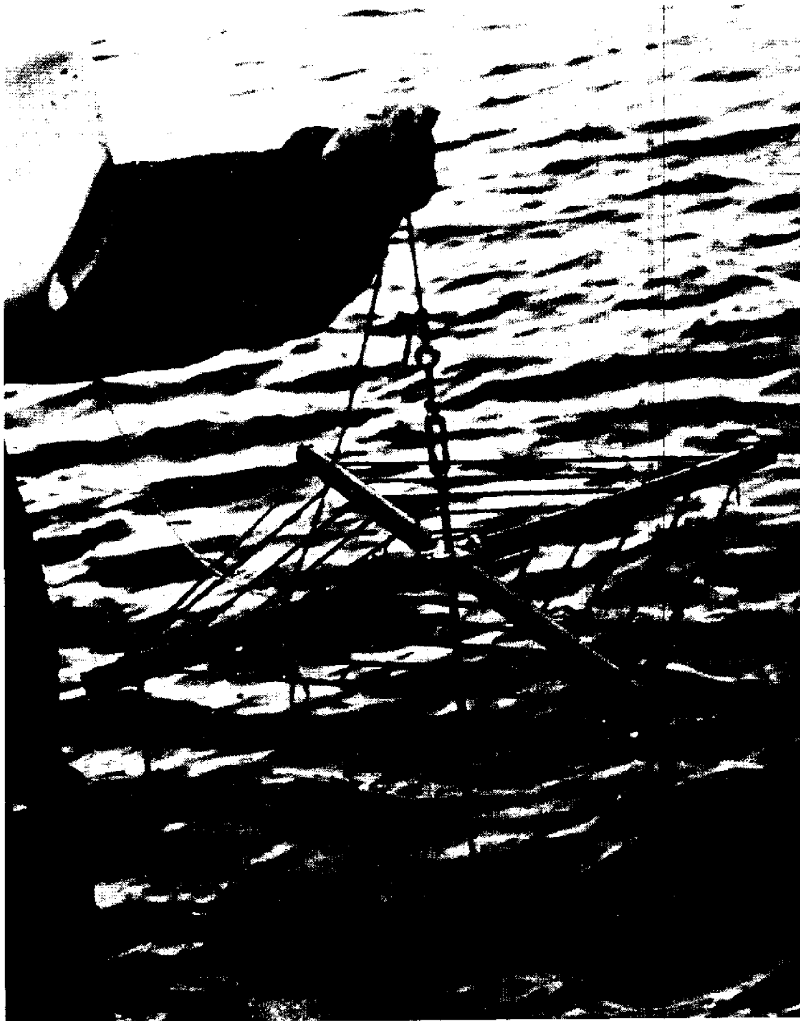
FIGURE 2.5 X-Shaped Plastic Pipe Frame Strung with Spore-Seeded Line for Growth and Yield Studies (The frame was suspended from a stiff rod supported by a surface buoy; a counterweight was used at the bottom of the rod to maintain the frame in a horizontal position in the water. A flexible anchor line tethered the unit to a bottom anchor. This design minimizes the surface area of rigging available for colonization by fouling organisms. The frame is approximately 0.5 x 0.5 m in surface area.)
