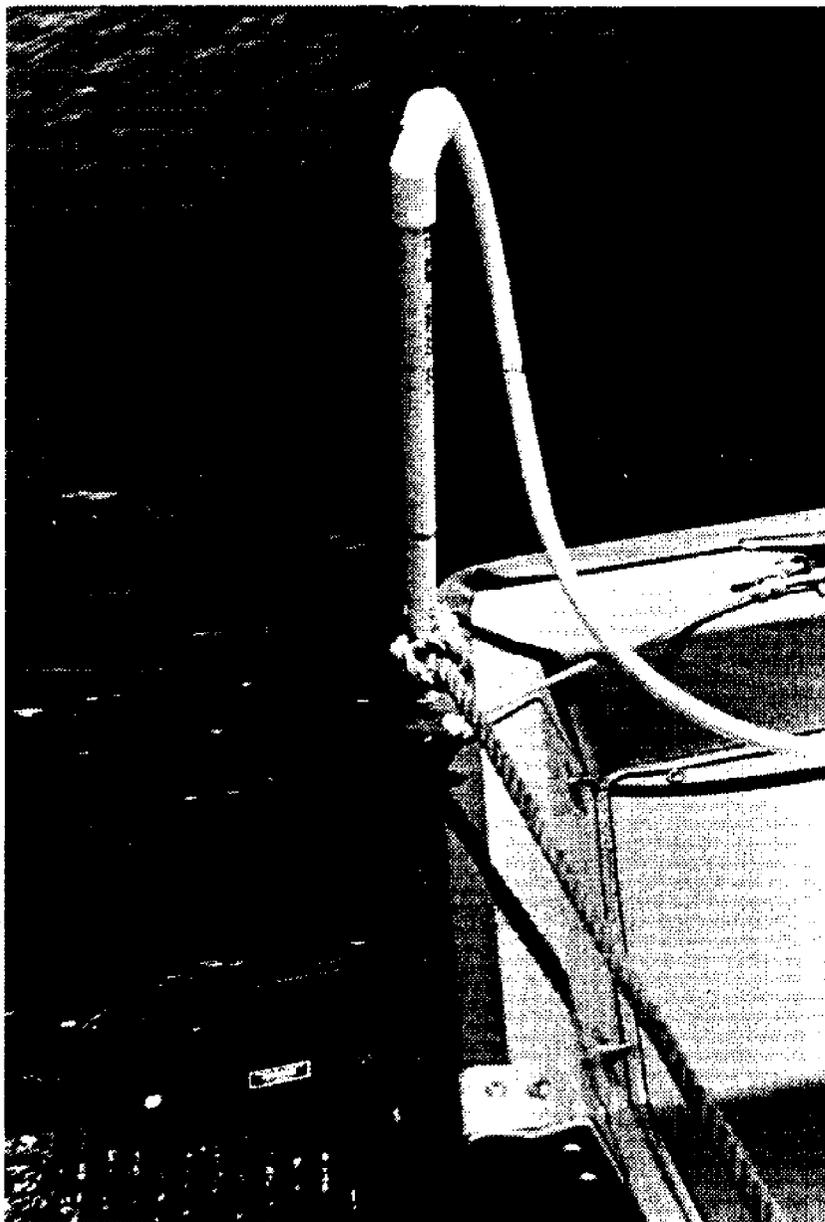
Figure 12.8 - Use of Short Length of PVC Pipe for Sampling Water-Tracing Dye From Moving Boat at 3 ft depth.
