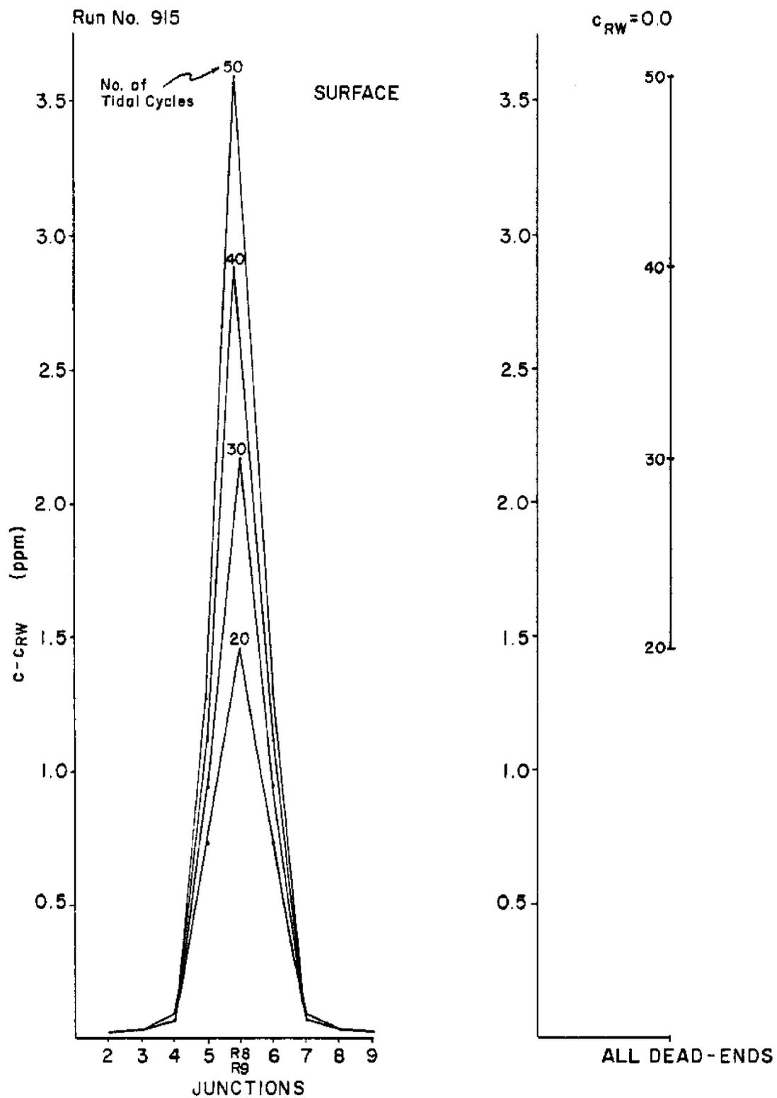
Figure 13.25a - Values of Surface Concentrations for No Wind at Junctions and Dead-ends at High Tide After Fifty Tidal Cycles, System D.
