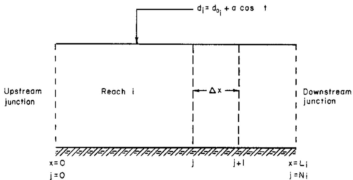
Figure 3.8 - Schematic Drawing of Horizontal Water Surface Assumption.
