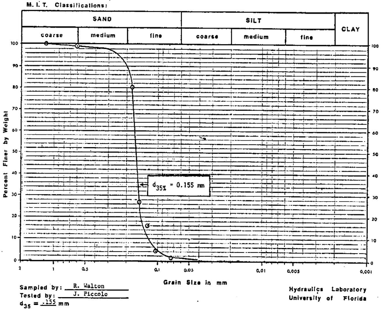
Figure 13.4 - Measured Bed Grain-size Distribution Curve for Sample From Station B, 57 Acres Canal System.
