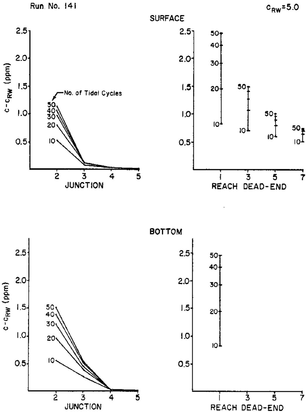
Figure 13.13 - Values of Surface and Bottom Concentration for West Wind, at Junctions and Dead-ends at High Tide After Fifty Tidal Cycles, System A.
