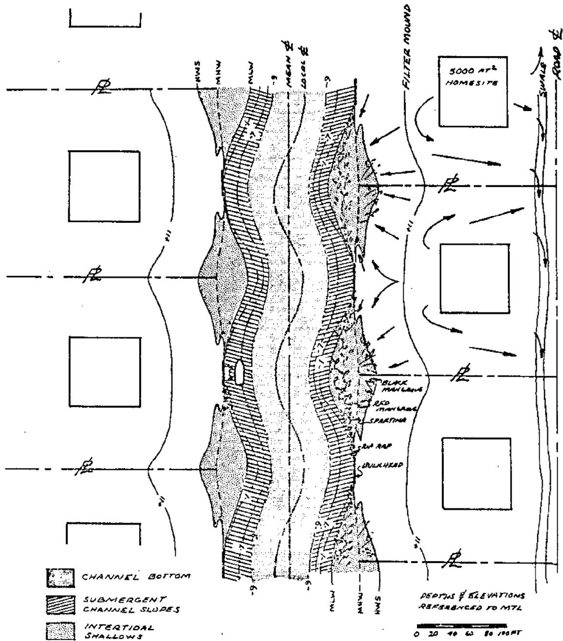
Figure 13.2 - Sinuous Bank Design for 57 Acres Project. (Source: Snyder, R. M., 1976, p. 77).
