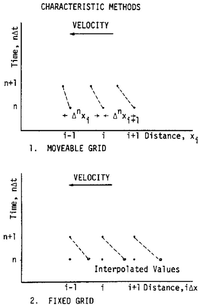
Figure 3.11 - Schematic Representation of Convective Steps of Method-of-Characteristics Methods.
