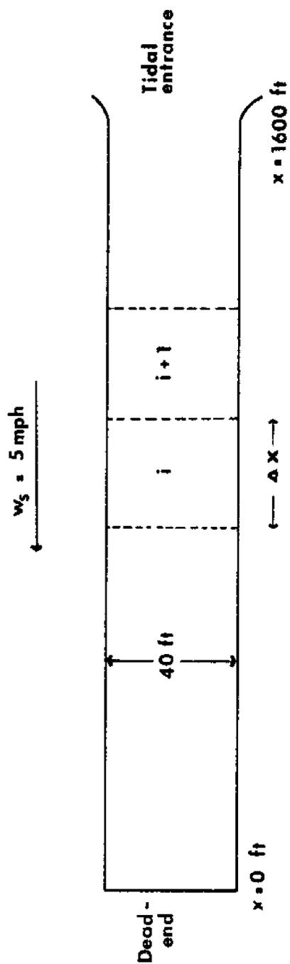
Figure 7.1 - Schematic Canal for Three-Dimensional Model Tests.
