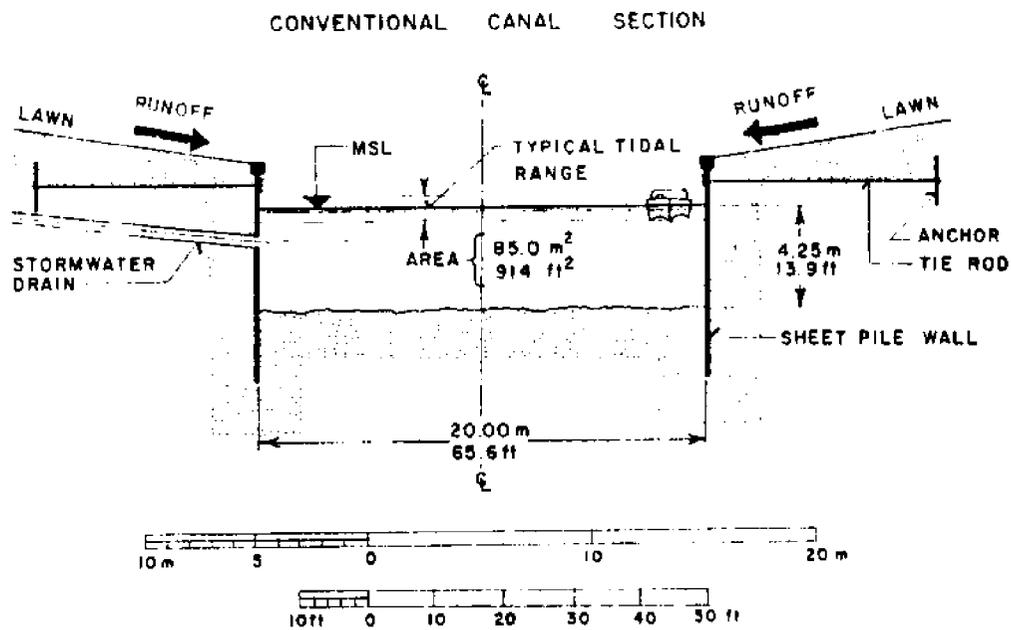
Figure 2.3 - Typical Cross-Section of Conventional Residential Canal
