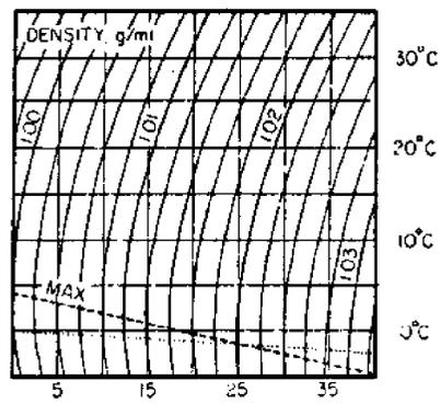
Figure 2.22 - Relationship of Density of Seawater (g/ml) to Salinity (ppt) and temperature ( $^{\circ}\text{C}$ ). (Source: Chow, 1964, p. 2-5)
