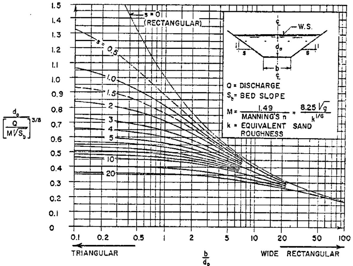
Figure 13.6 - Design Chart for Trapezoidal Channels.
