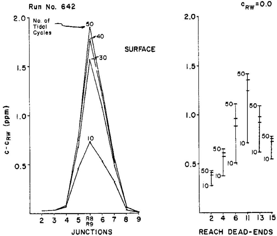
Figure 13.26a - Values of Surface Concentrations for East Wind, at Junctions and Dead-ends at High Tide After Fifty Tidal Cycles, System D.
