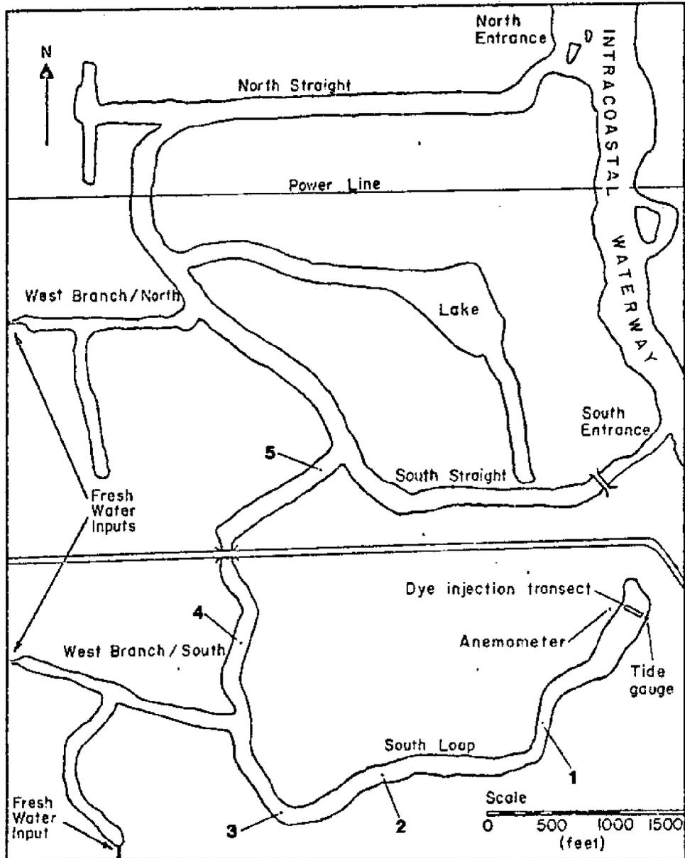
Figure 2.26 - 57 Acres Site Plan Showing Location of Electromagnetic Current Meters for October 1977 Velocity, Salinity, and Water Temperature Measurements.
