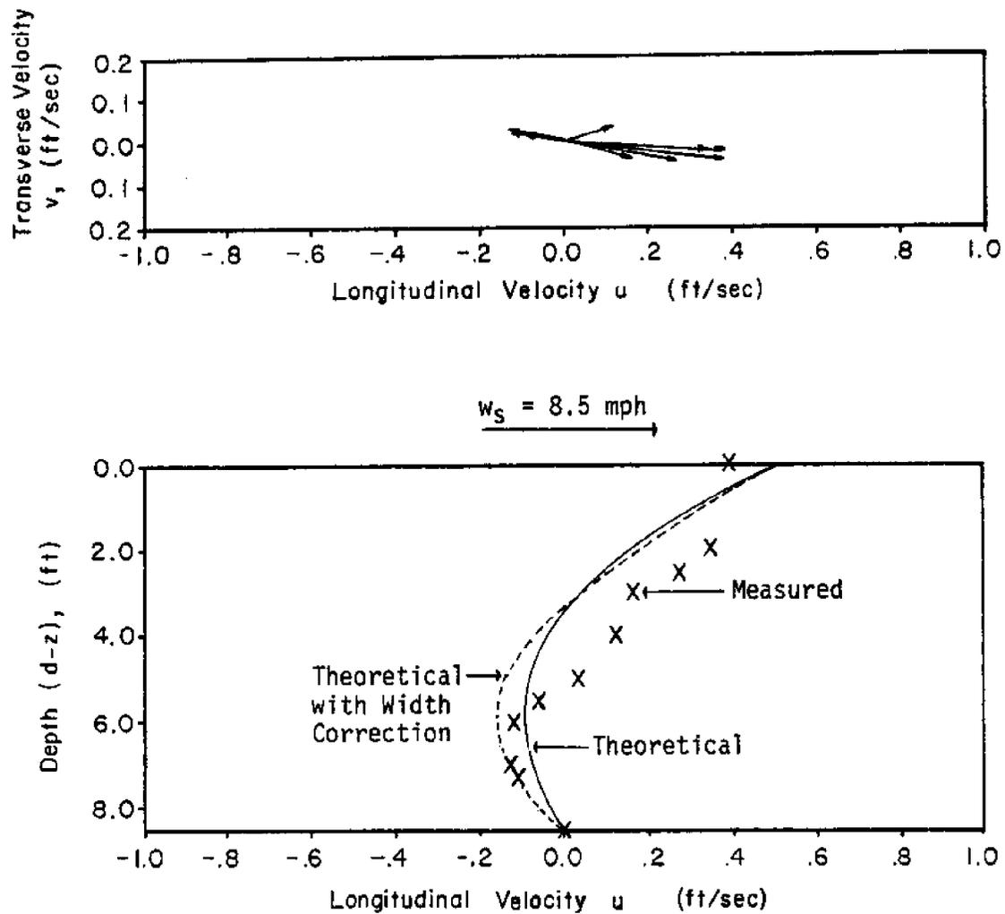
Figure 4.5 - Comparison Between Observed and Theoretical Wind-Induced Vertical Velocity Profiles, With and Without Width Correction ( $N_z = 0.002 \text{ ft}^2/\text{sec}$ ) - 57 Acres.
