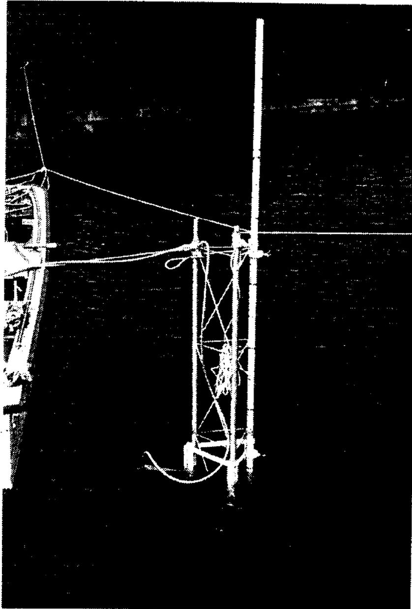
Figure 12.4 - Velocity Meter Tower Set-Up in Canal.
