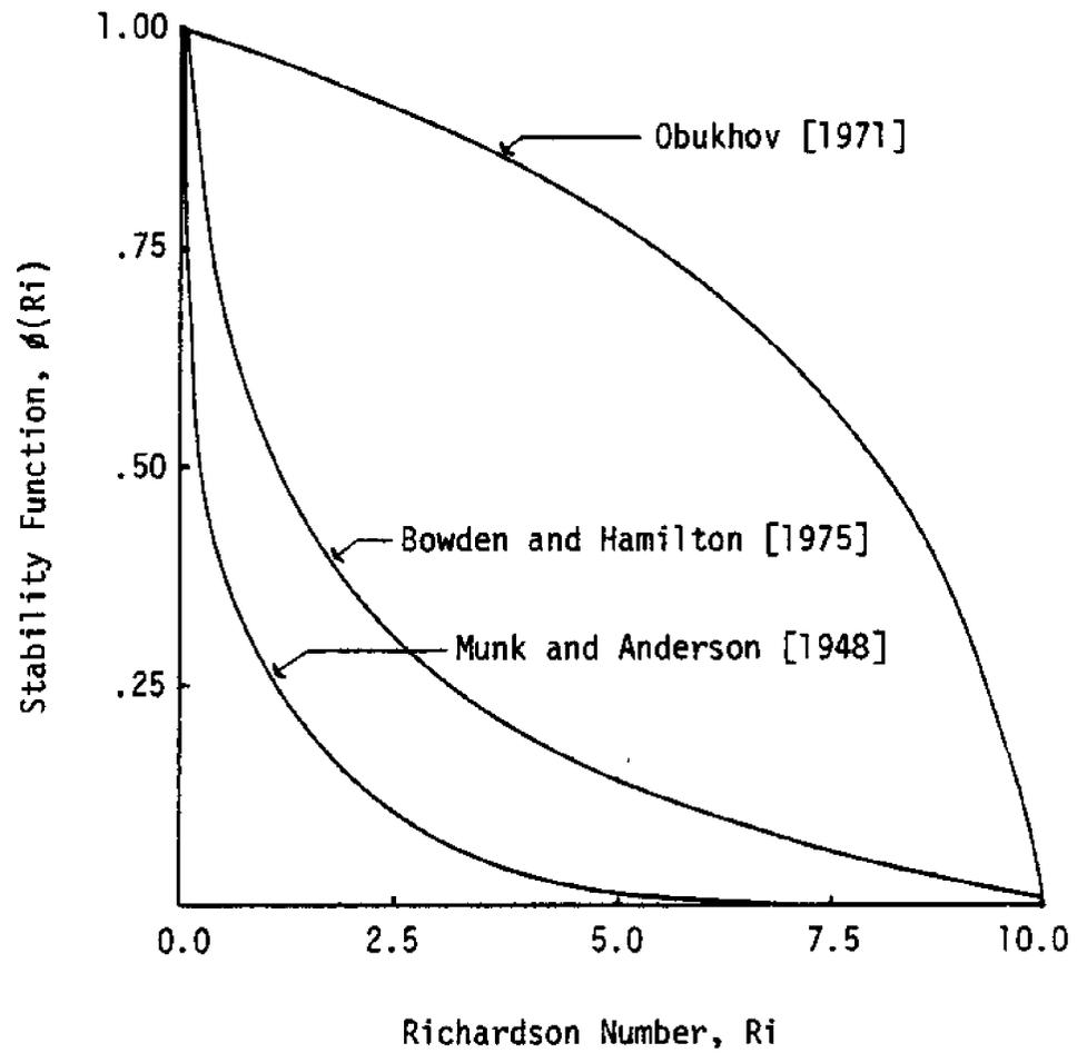
Figure 5.2 - Comparison of Saltwater Interface Stability Function.
