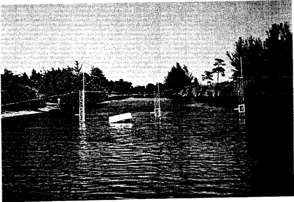
Figure 12.5 - Three Velocity Meter Towers Installed in the Loxahatchee North Canal.
