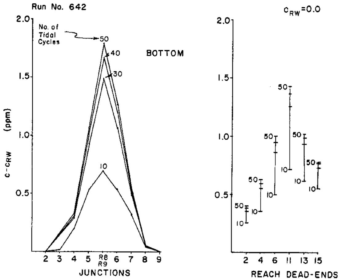
Figure 13.26b - Values of Bottom Concentrations for East Wind, at Junctions and Dead-ends at High Tide After Fifty Tidal Cycles, System D.
