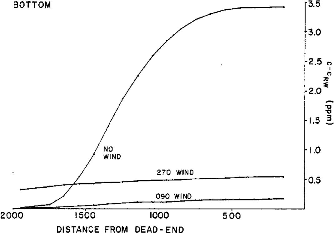
Figure 13.19 - Values of Surface and Bottom Concentrations for Three Wind Conditions in Reach Number 3 at High Tide After Forty-eight Tidal Cycles, System B.
