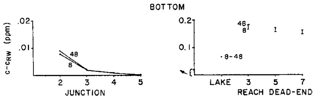
Figure 13.21 - Values of Surface and Bottom Concentrations for East Wind at Junctions and Dead-ends at High Tide After Forty-eight Tidal Cycles, System B.
