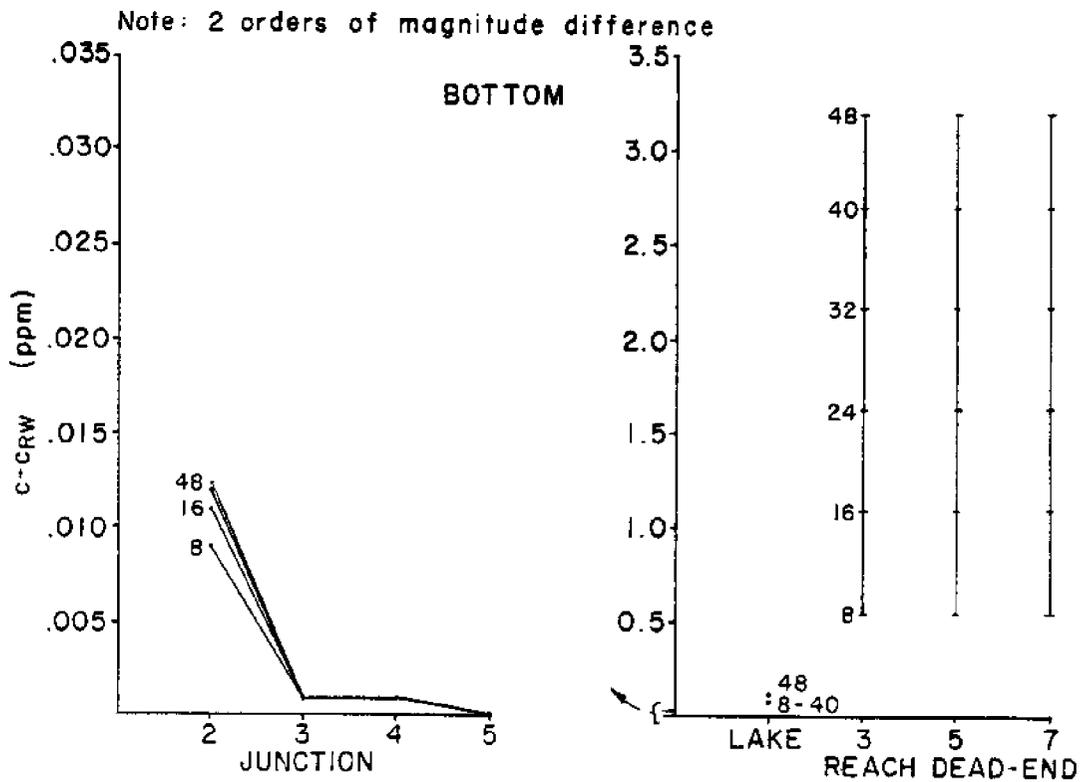
Figure 13.18 - Values of Surface and Bottom Concentrations for No Wind at Junctions and Dead-ends at High Tide After Forty-eight Tidal Cycles, System B.
