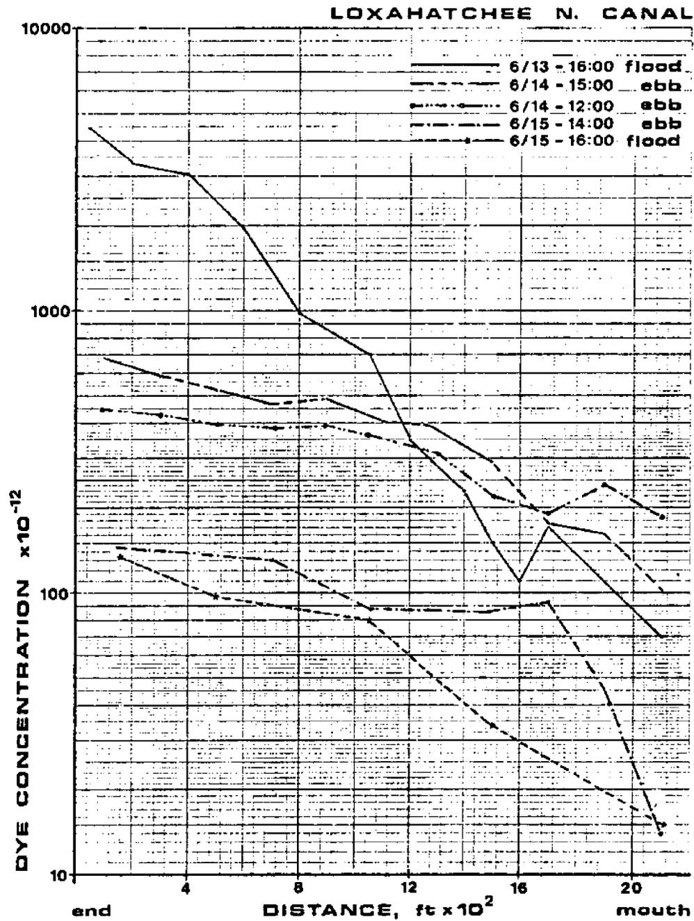
Figure 12.14 - Example of Vertically-Averaged Dye Concentration Profiles.
