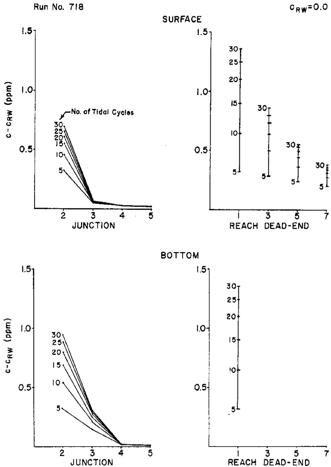
Figure 13:15 - Values of Surface and Bottom Concentration for East Wind, at Junctions and Dead-ends at High Tide After Thirty Tidal Cycles, System A.
