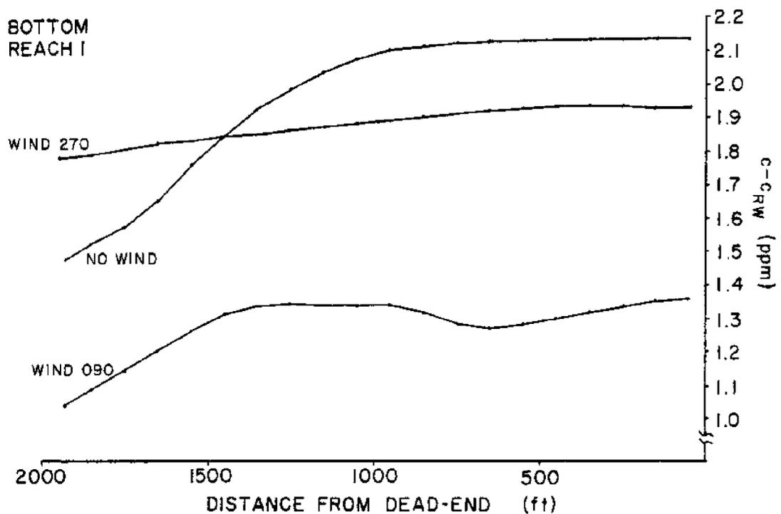
Figure 13.14 - Values of Surface and Bottom Concentrations for Three Wind Conditions in Reach Number 1 at High Tide After Thirty Tidal Cycles, System A.
