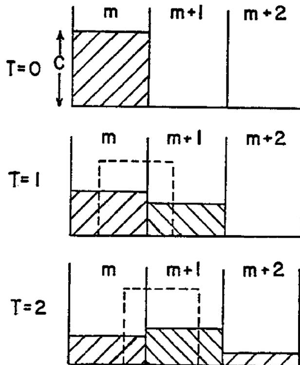
Figure 3.9 - Schematic Representation of Effect of Numerical Dispersion.
