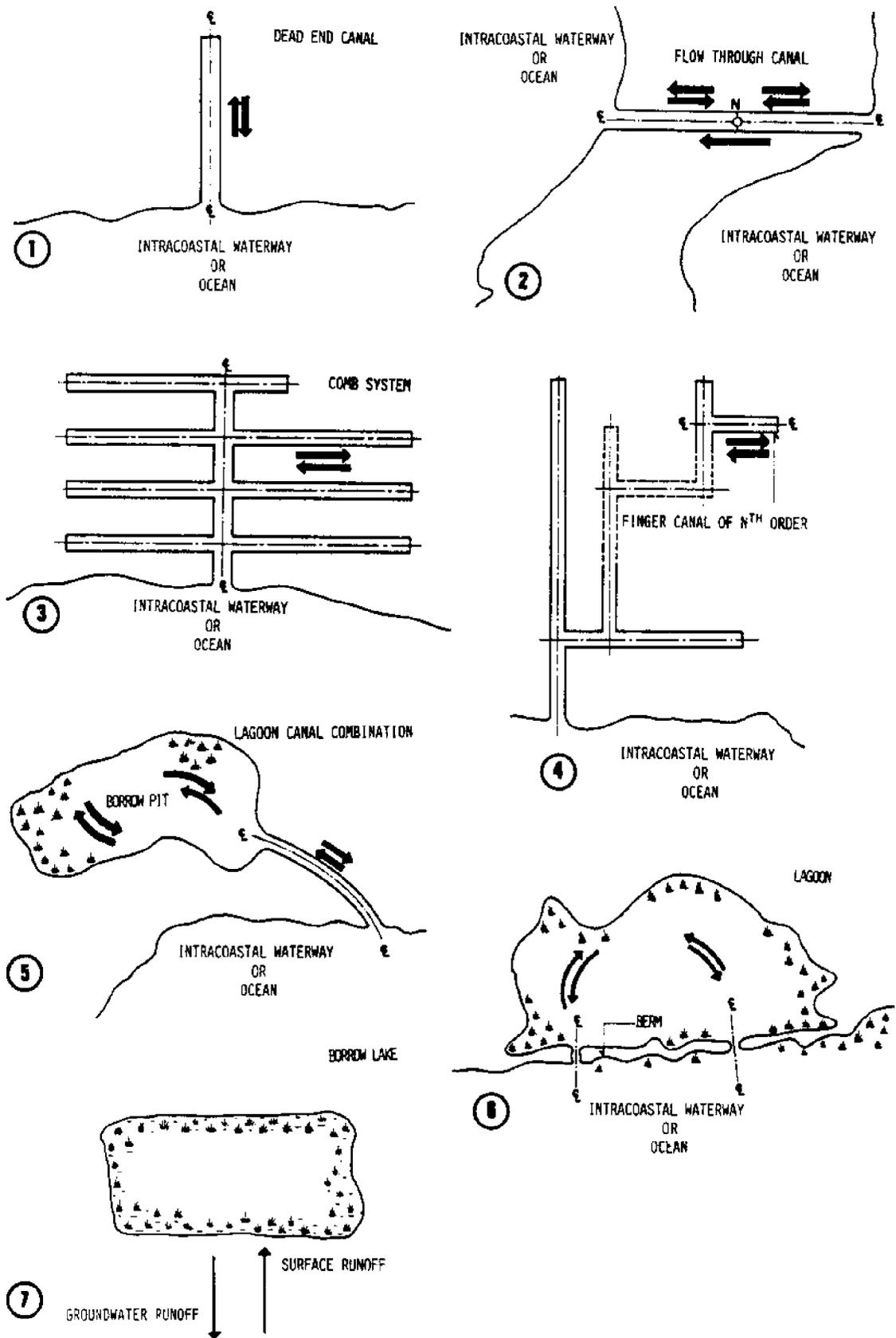
Figure 2.2 - A Geometric Classification for Types of Canals.
