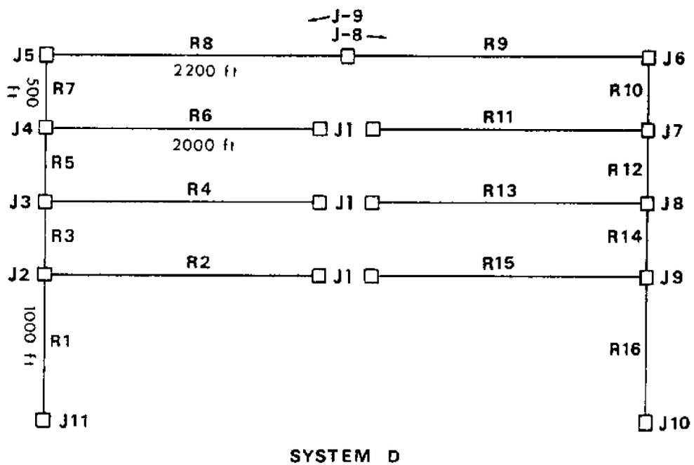
Figure 13.24 - Layout and Dimensions of System D.
