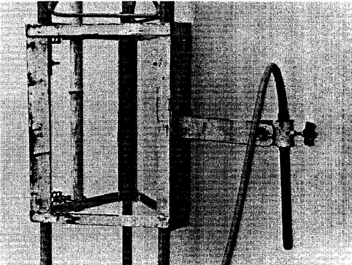
Figure 12.3b - Detail of Probe Holder Carriage on Velocity Meter Tower,
