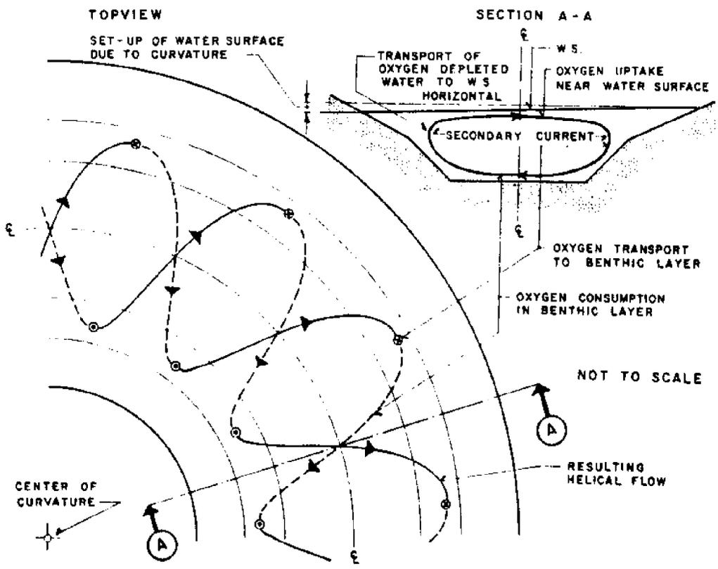
Figure 4.6 - Schematic Drawing of Helical Current Induced by a Bend.
