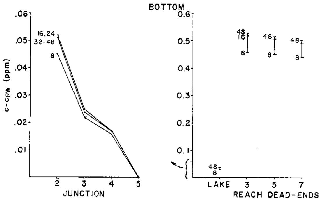
Figure 13.20 - Values of Surface and Bottom Concentrations for West Wind at Junctions and Dead-ends at High Tide After Forty-eight Tidal Cycles, System B.
