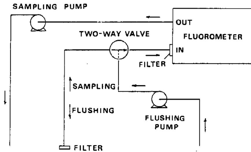
Figure 12.7 - Diagram of Continuous Flow Dye Sampling System.
