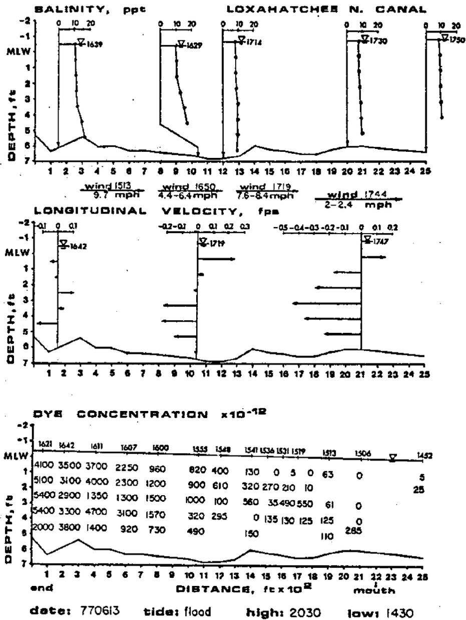
Figure 12.12 - Example of Plotted Salinity, Velocity, and Dye Concentration Profiles.
