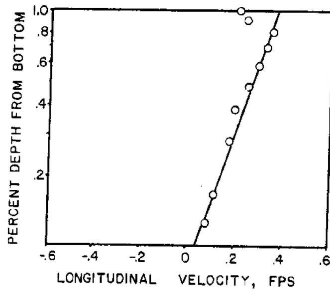
Figure 3.7 - Typical Logarithmic Velocity Profile.
