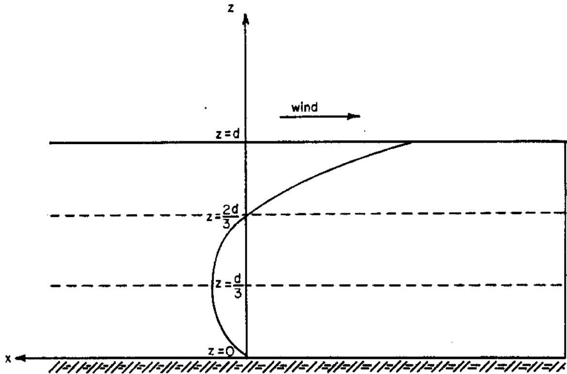
Figure 4.4 - Theoretical Wind-Induced Vertical Velocity Profile.
