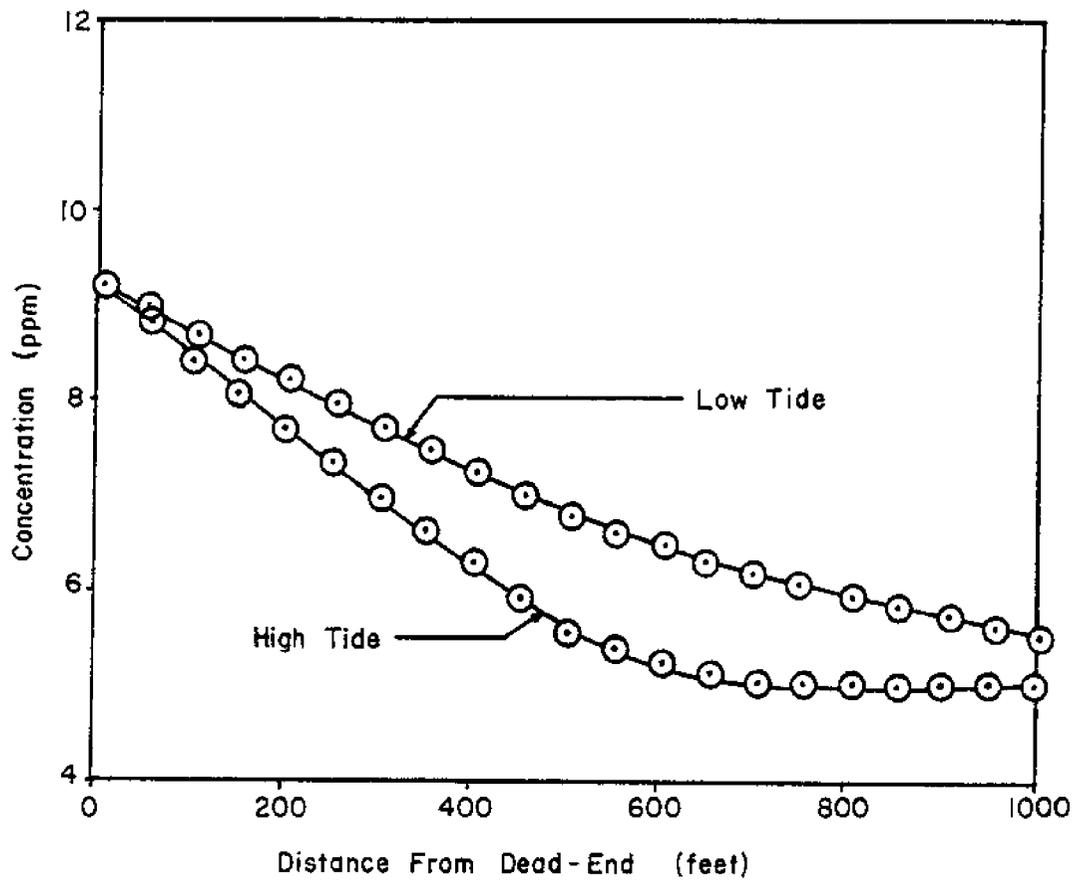
Figure 3.26 - Concentration Profiles for Second Test Canal Network - Method of Second Moments.
