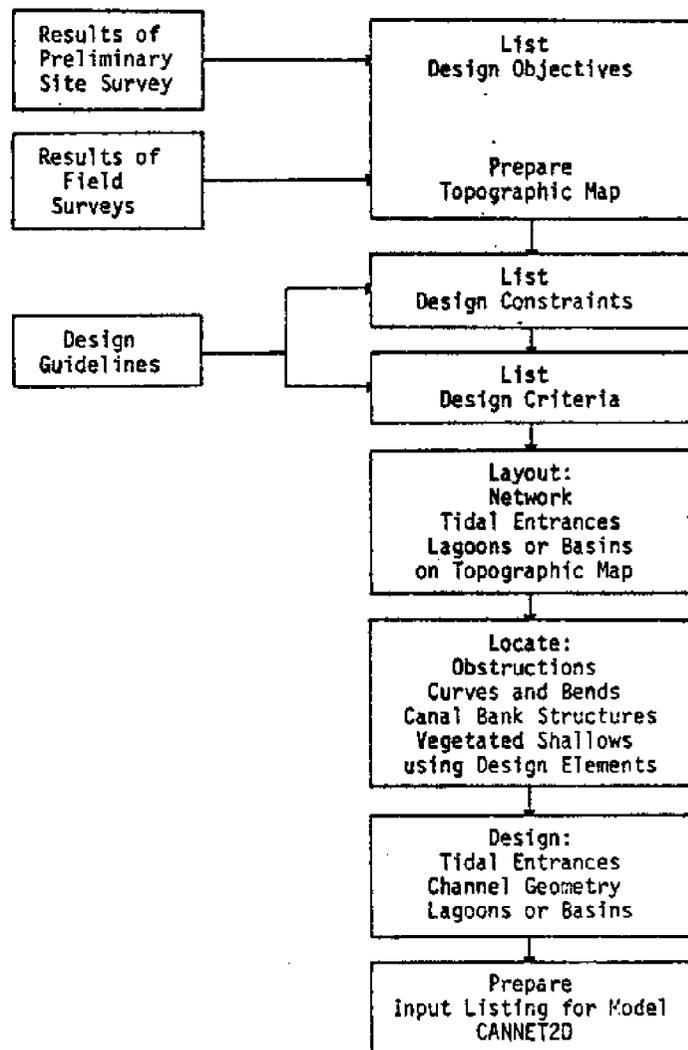
Figure 13.1 - Steps in Formulating a Trial Canal Design.
