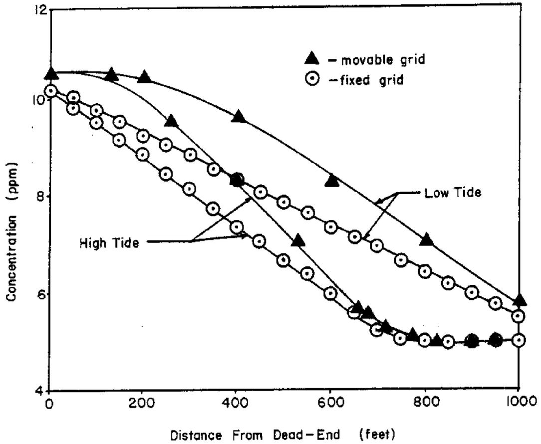
Figure 3.12 - Comparison of Concentration Profiles for Fixed Grids and Movable Grid Method-of-Characteristics.
