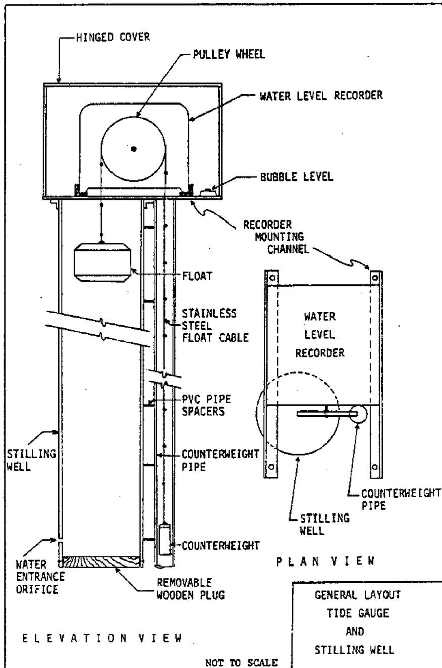
Figure 12.2 - Typical Stilling Well and Water Level Recorder Box for the Tide Measurements.
