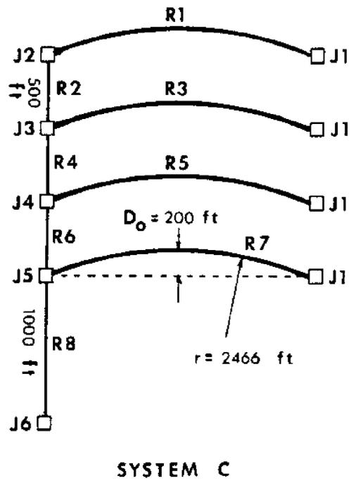
Figure 13.22 - Layout and Dimensions of System C.
