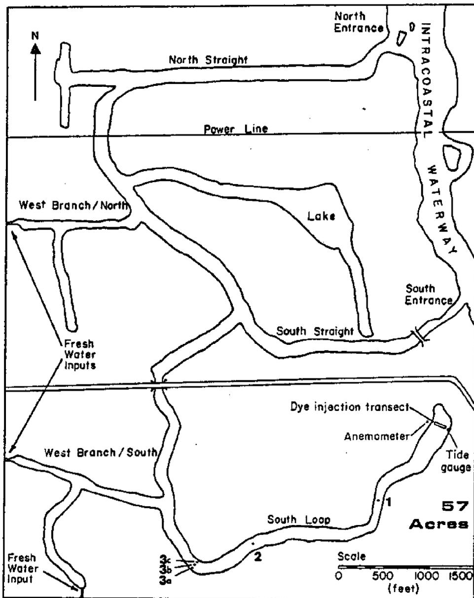
Figure 2.27 - 57 Acres Site Plan Showing Location of Electromagnetic Current Meters for October 1977 Dye Dispersion Measurements.
