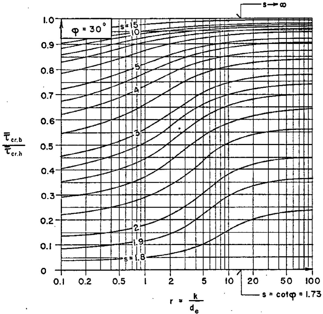
Figure 13.5 - Critical Shear Stress Ratio  $\bar{\tau}_{cr.b}/\bar{\tau}_{cr.h}$  as a Function of Correction Factor,  $r$ , and Inverse Bank Slope,  $s$ .
