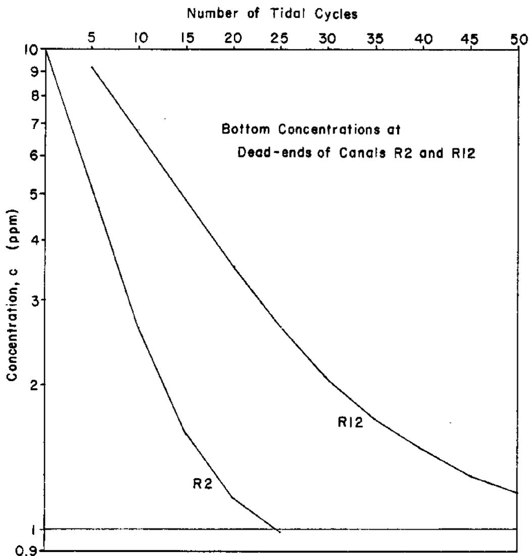
Figure 14.17 - Semilogarithmic Plot of Laterally-averaged Bottom Concentration at the Dead-ends of Canals R2 and R12 versus Number of Tidal Cycles for 4-ft-deep Alternate Canal Network After Thirty and Fifty Tidal Cycles, With Lake Surface Area of 30 percent of Network Surface Area and With a Steady Wind of 5 mph From the East (Run No. 633).
