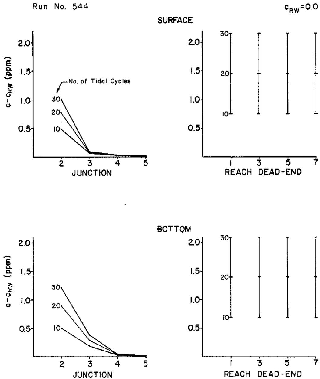
Figure 13.12 - Values of Surface and Bottom Concentrations for No Wind at Junctions and Dead-Ends at High Tide After Thirty Tidal Cycles, System A.
