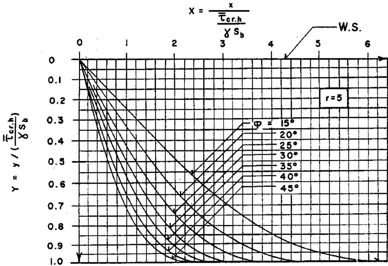
Figure 13.7 - Stable Bank Profile, Mild Slope, Cohesionless Material,  $r = 5$ .
