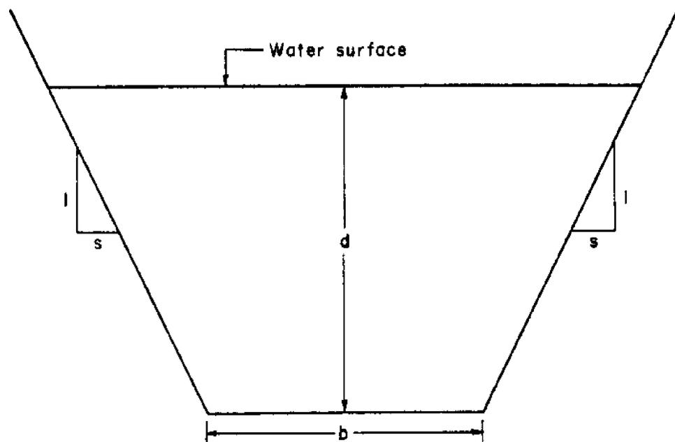
Figure 3.2 - Schematic Drawing of Trapezoidal Cross-Section.
