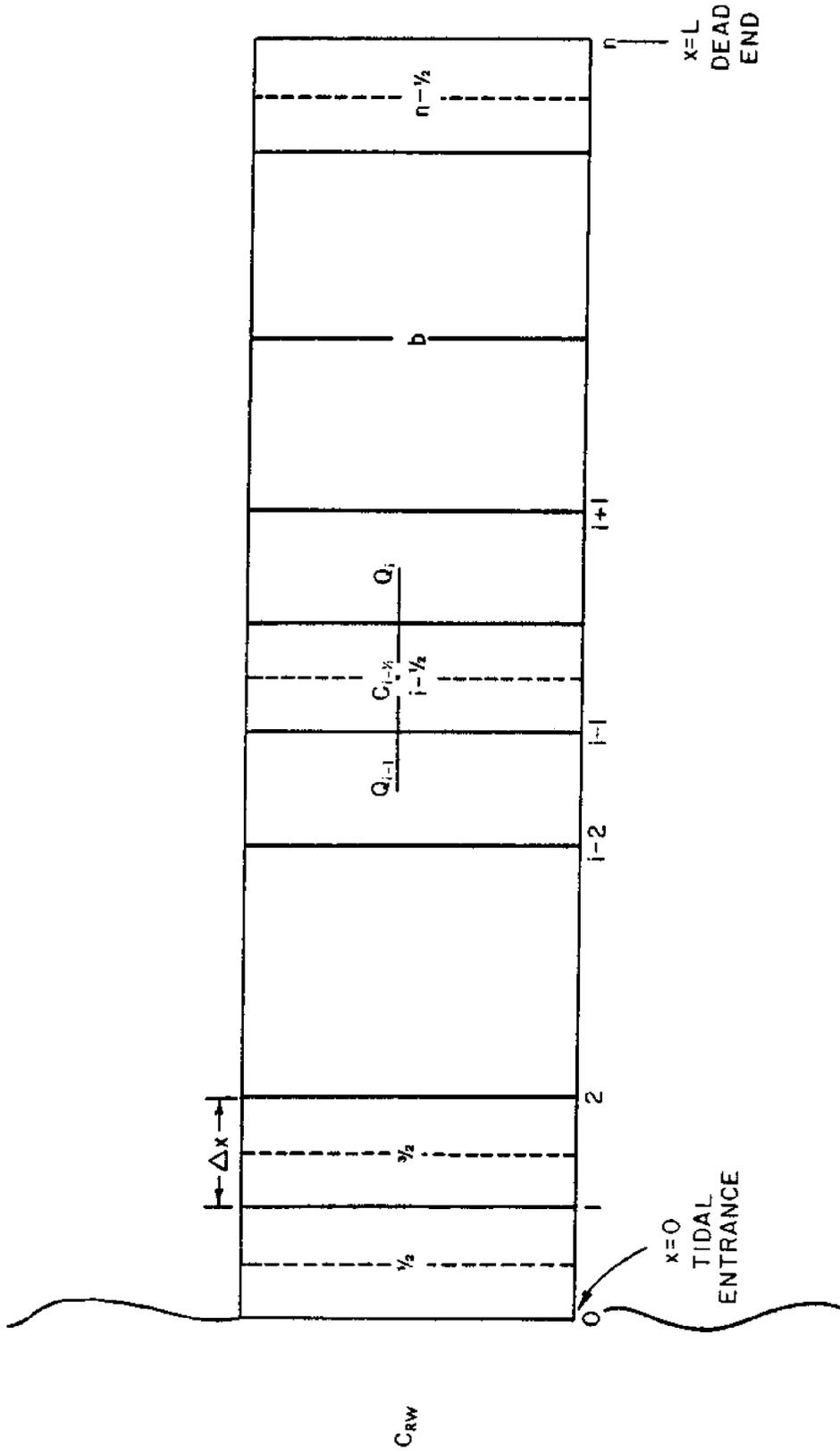
Figure 3.18 - Schematic Representation of Second Upwind Difference Method.
