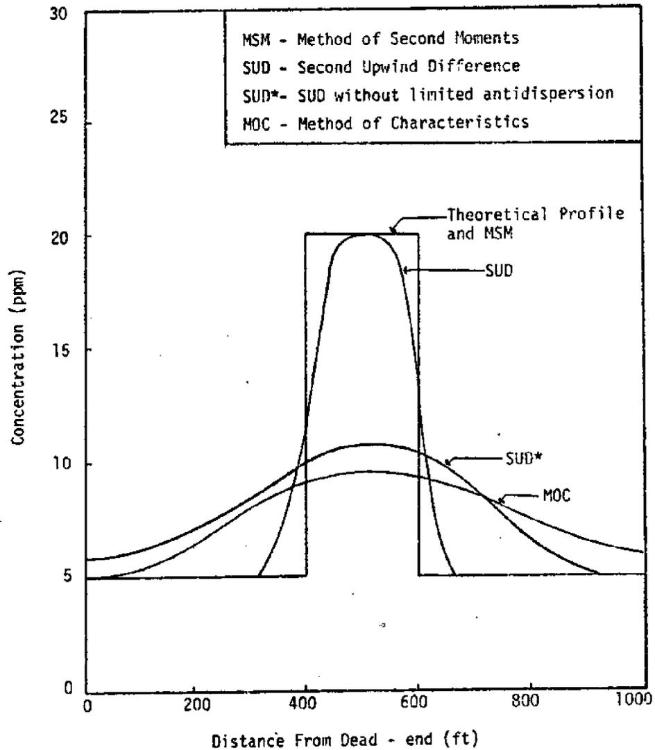
Figure 3.23 - Comparison of Techniques' Accuracy in Modeling Pure Convection.
