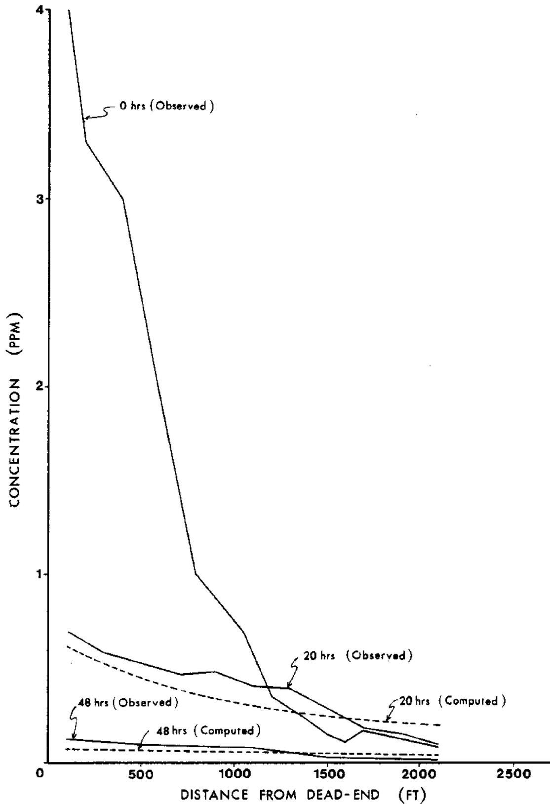
Figure 8.7 - Comparison Between Observed and Computed Concentration for Loxahatchee River North Canal, June, 1977.
