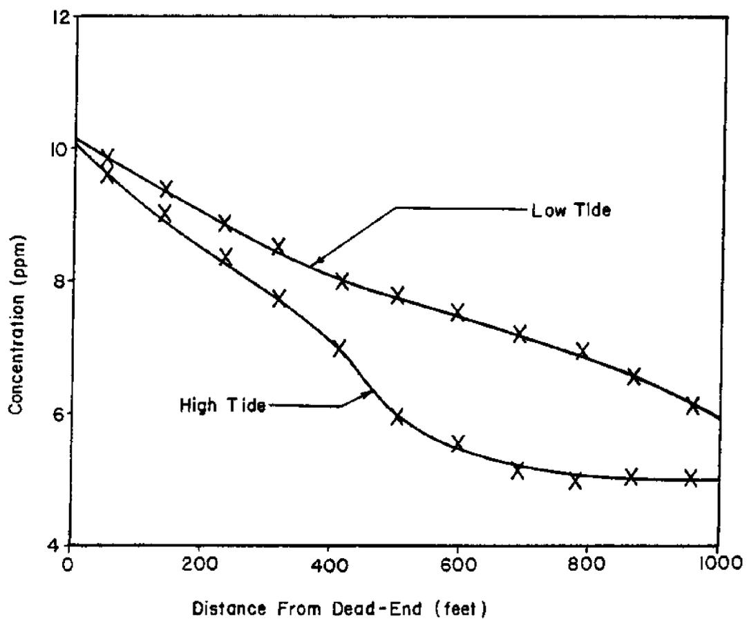
Figure 3.25 - Concentration Profiles for Second Test Canal Network - Second Upwind Difference Method.
