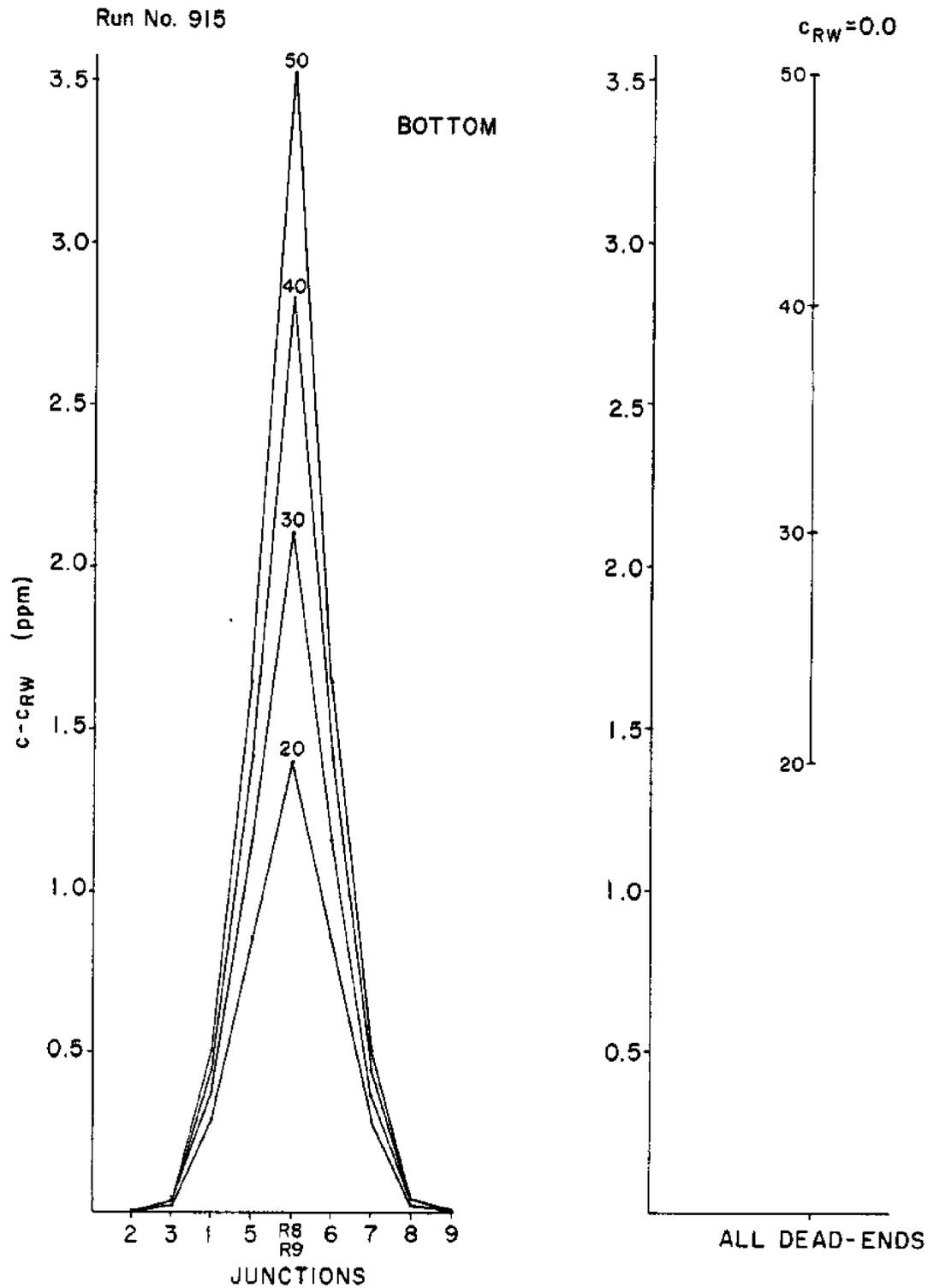
Figure 13.25b - Values of Bottom Concentrations for No Wind at Junctions and Dead-ends at High Tide After Fifty Tidal Cycles, System D.
