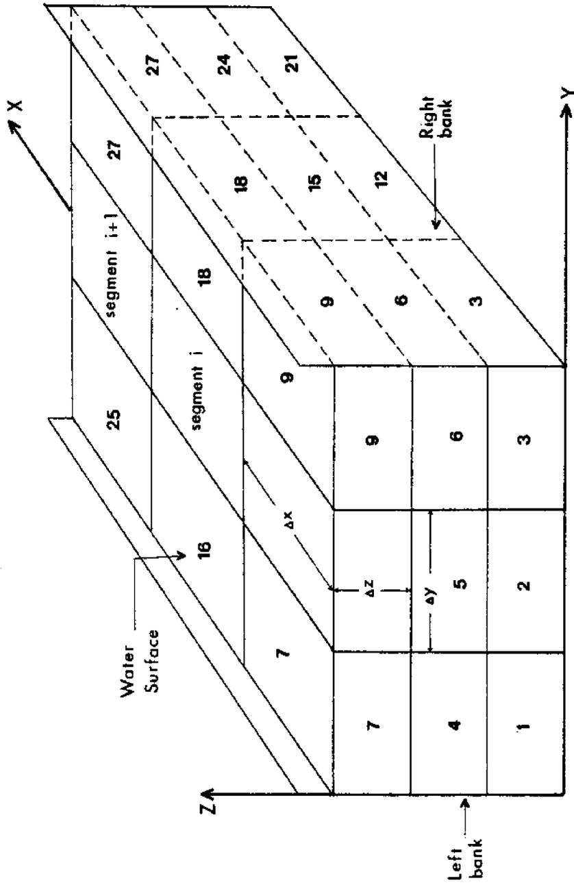
Figure 6.3 - Cell Structure in Reach.
