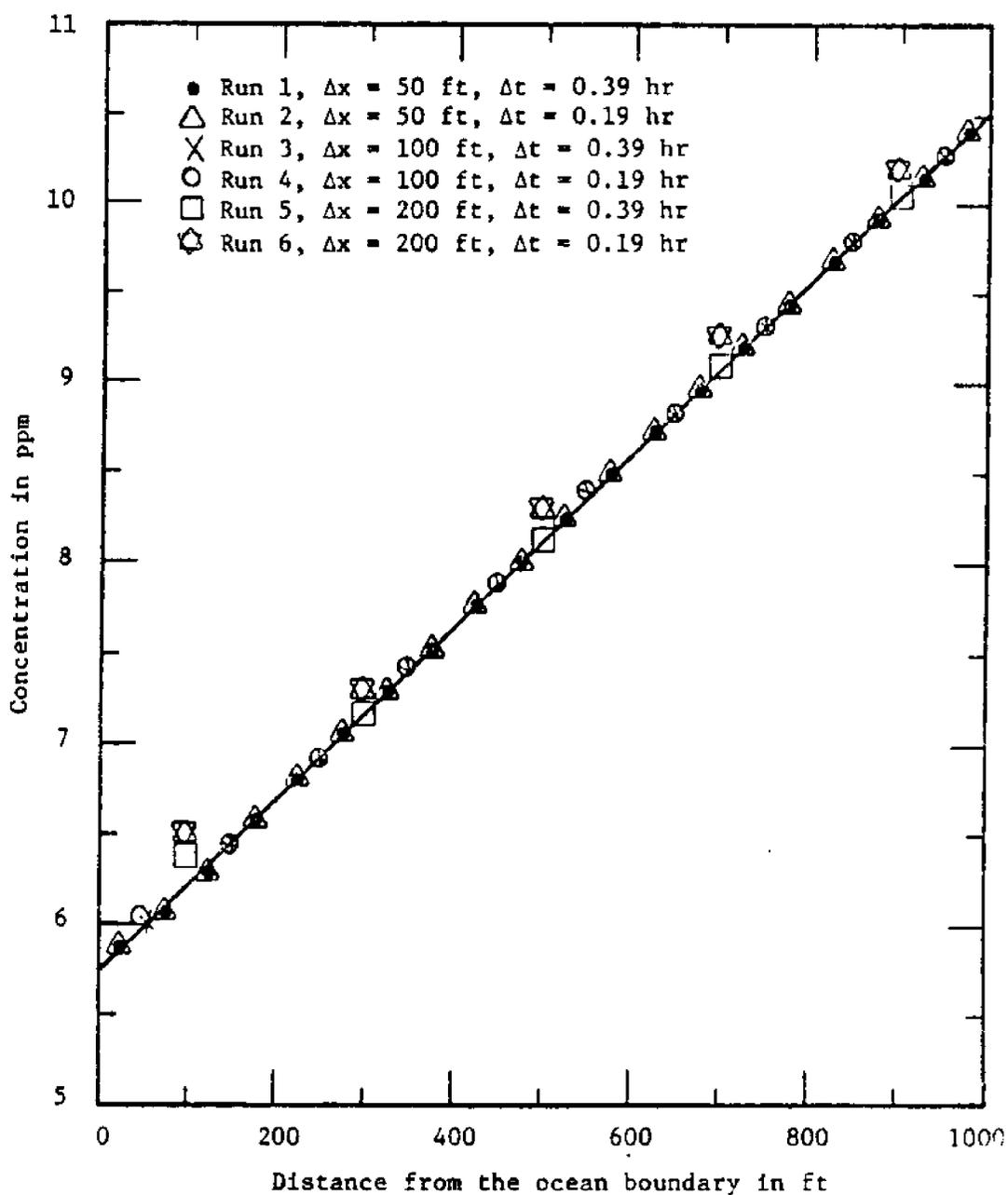
Figure 3.19 - Low Tide Concentration Profiles for Various  $\Delta x$  and  $\Delta t$  - Second Upwind Difference Method.
