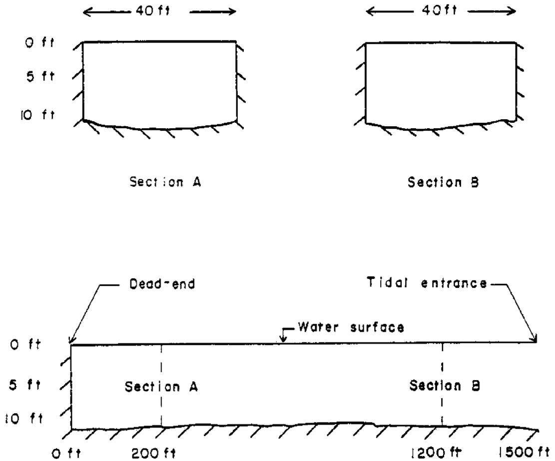
Figure 8.2 - Typical Longitudinal Sections and Cross-Sections, Big Pine Key Canal III, Florida [EPA, May, 1975].
