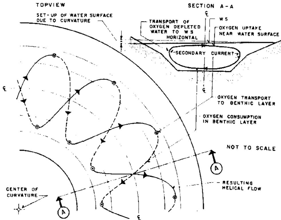
Figure 2.14 - Secondary Current and Resulting Helical Flow in Canal Bend.
