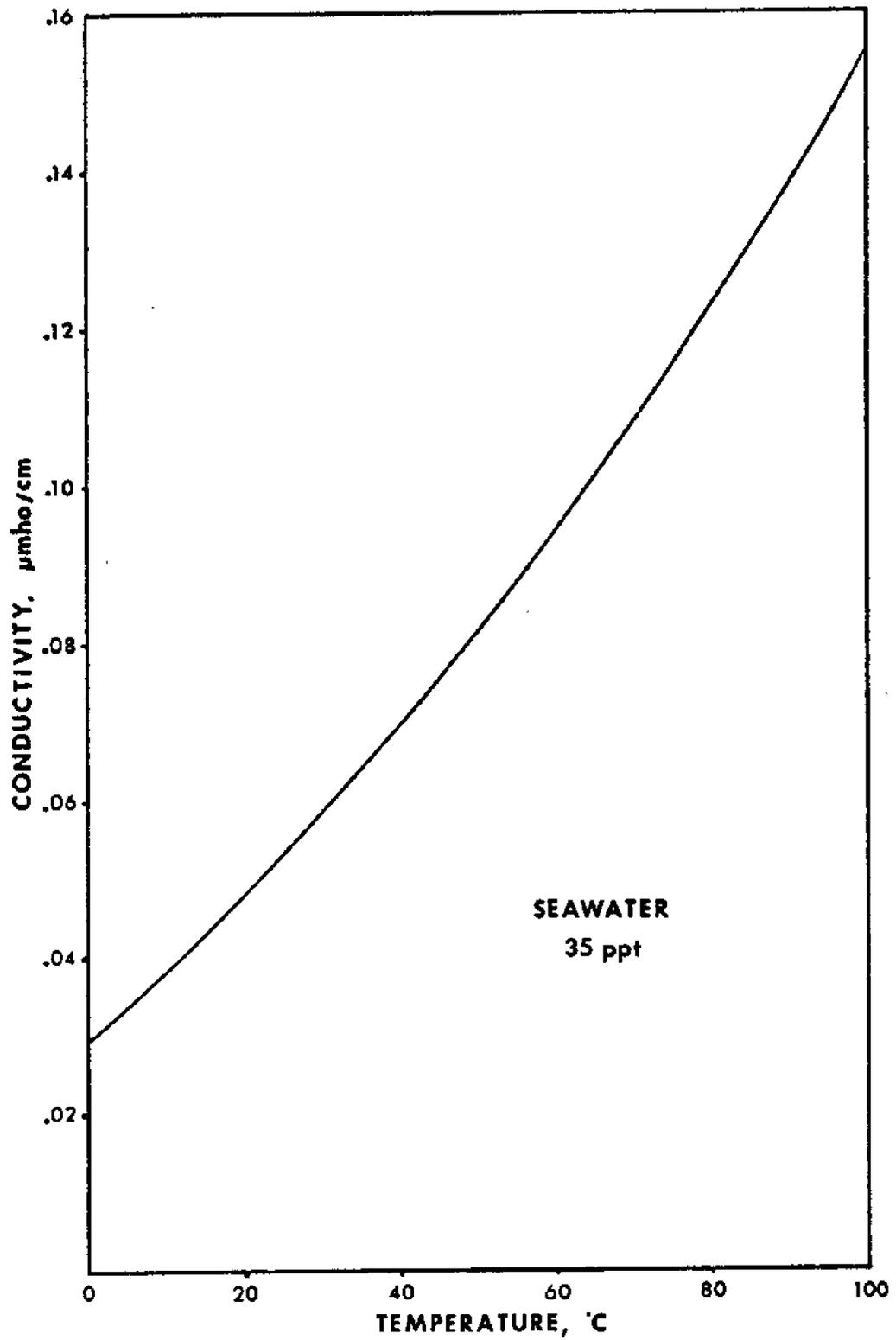
Figure 12.6 - Electrical Conductivity of Seawater as a Function of Temperature (Source: Higgins, L. L., 1962, p. 2.6).
