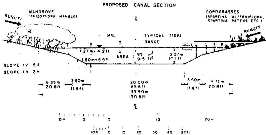
Figure 2.4 - Proposed Canal-Section With Same Area as the Conventional Canal Section Shown in Figure 2.3 (Source: Christensen and Snyder, 1978, p. 5).
