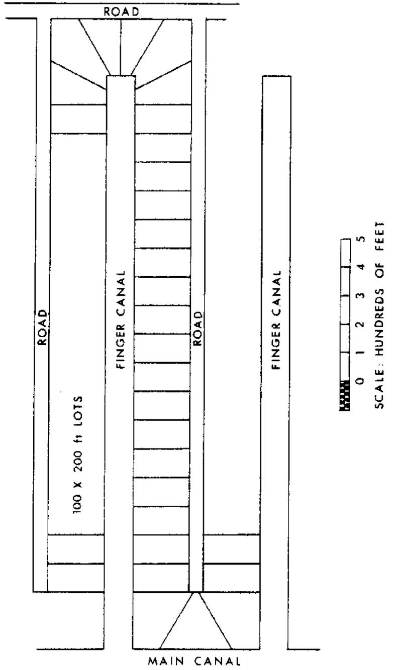
Figure 13.9 - Test Canal and Lot Dimensions.
