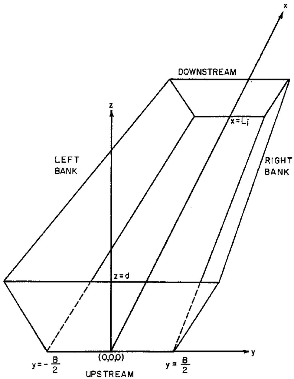
Figure 4.2 - Definition of Coordinate System.
