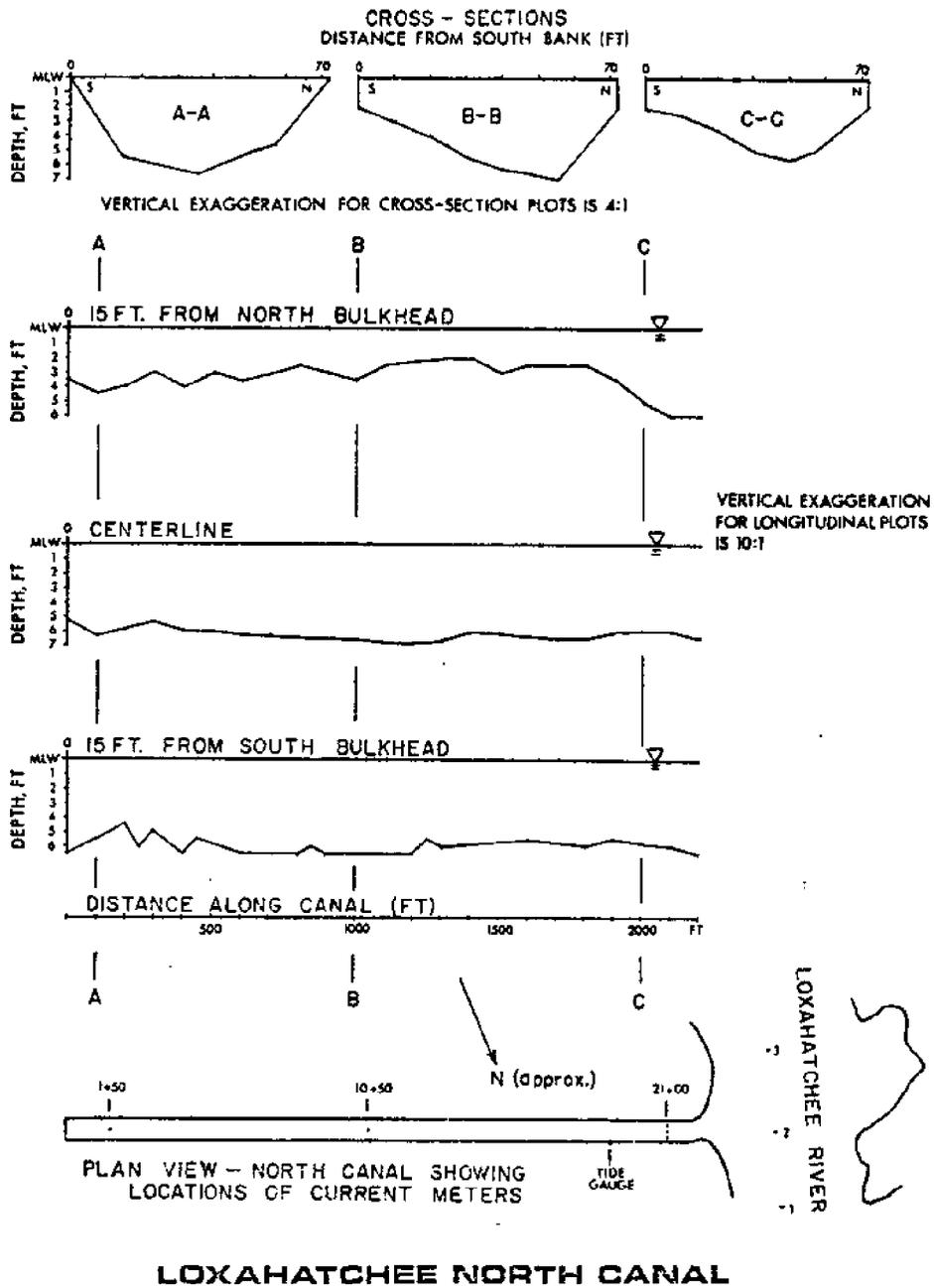
Figure 2.12 - Cross-Sections and Plan View of Loxahatchee North Canal, June 1977.
