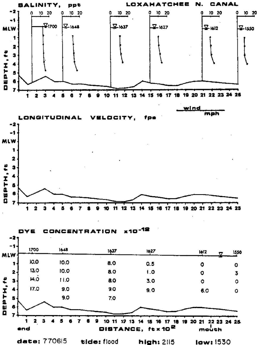
Figure 2.24 - Vertical Salinity Profiles, Loxahatchee North Canal, Showing Slight Density Gradient
