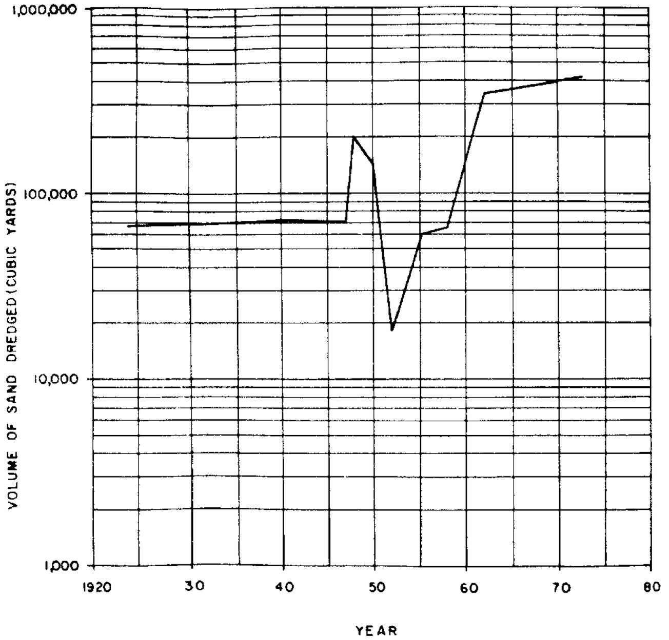
Fig. 4.9 Volume of Sand Dredged from Sebastian Inlet as a Function of Years.
