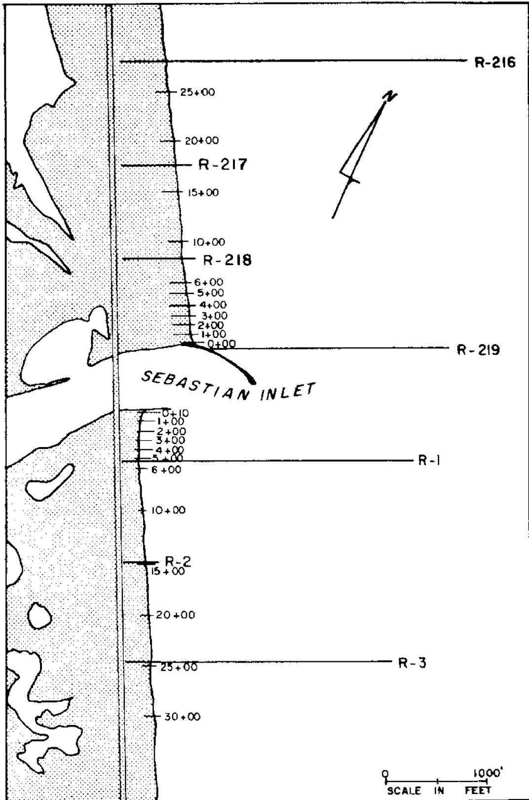
Fig. 5.4 Locations and Lengths of Setback Line Profiles near Sebastian Inlet. Also Shown are Locations of Profiles by Beindorf and Associates of Vero Beach. The Latter Profiles have been obtained once a Year Since 1967.
