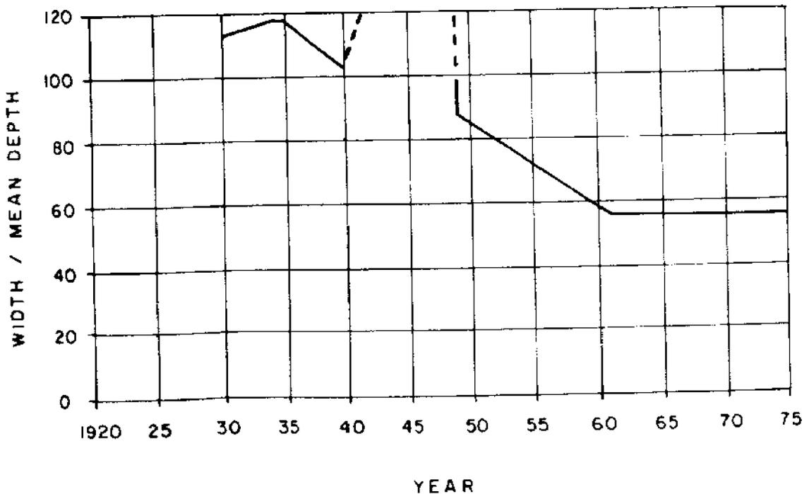
Fig. 5.2 Ratio of Width to Depth (below MLW) at the Throat Section of Sebastian Inlet Plotted against Time in Years.
