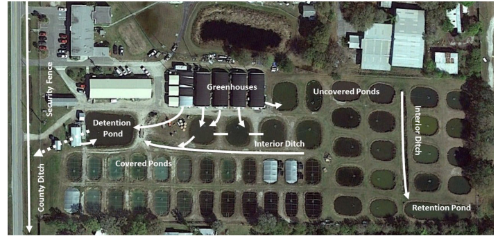
Figure 1. Representative fish farm layout. Water flow direction is indicated by arrows. Effluent from buildings and greenhouses flows into an interior ditch that empties into a detention pond. The detention pond discharges to the county ditch, the only surface water connection between the farm and the outside environment. Ponds are periodically dewatered by pumping into one of the interior ditches. The facility has security fencing, locked gates, and security lighting.
