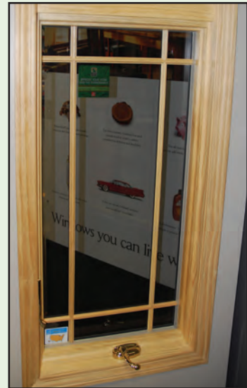
Figure 4-11: This attractive window can be fitted with energy-efficient glass, impact-resistant glass, or both. The impact resistant glass consists of a laminate or film sandwiched between two glass panes. The frames are reinforced and the hinges have extra fasteners to withstand high wind events. During a wind event, debris may crack the glass, but the laminate will hold the window pane together in the frame and prevent breaching of the wind- and rain-resistant envelope. After the storm, the glass will need to be replaced.
