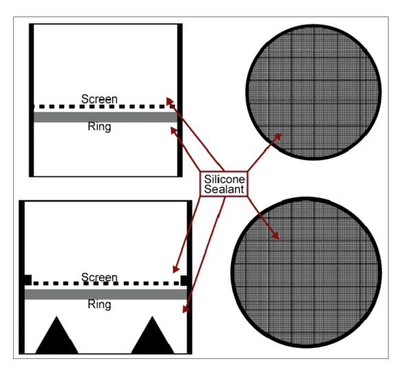
Figure 12. Stacked sieves schematic.
