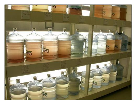
Figure 7. Carboy algae culture. Lights are maintained on an 18 h on / 6 h off cycle.
