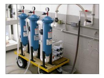
Figure 4. Filter set and ultraviolet sterilizer.
