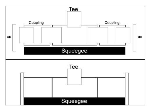
Figure 10. Squeegee longitudinal section schematic.
