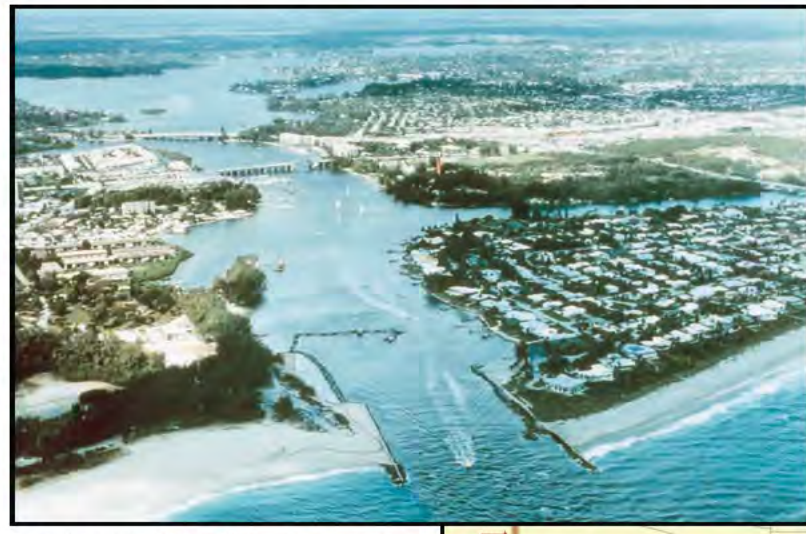
In the foreground of this 1997 aerial photograph, a dredge pumps material from the "sand trap" in Jupiter Inlet and deposits it on the beach south of the inlet. To the west, beyond the bridges, are the Loxahatchee River Central Embayment and the river's North and Northwest Forks. Photo credit: National Oceanographic & Atmospheric Administration Photo Library (Mrs. Marge Beaver, photographer)
