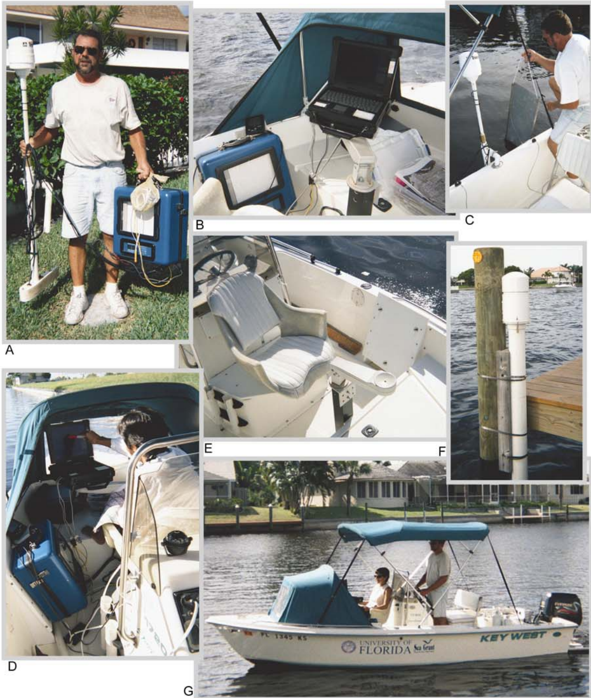
A. Bathy 500-MF Sounder, Transducer, and DGPS Antenna B. Data Collector's Work Station C. Bar Check D. Data Collector During Soundings
