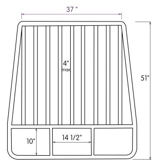
FIGURE 2: Modified Flounder TED Outside fram 1 1/2" OD AL pipe Horizontal bar 1 1/4" OD AL pipe Vertical bars 1 inch OD AL pipe
