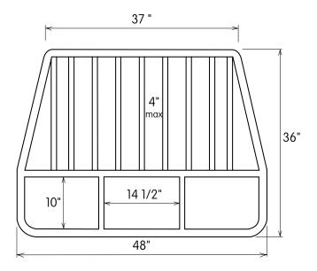
FIGURE 3: Modified Flounder TED short version Outer frame 1 1/2" OD AL pipe Horizontal bar 1 1/4" OD AL pipe Vertical bars 1 inch OD Al pipe
