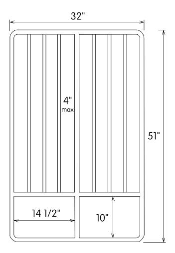
FIGURE 1: Flounder TED original configuration Outer Frame and Grid Bars Minimum Size: 1 1/4" outside diameter (OD) aluminum (AL) pipe with 1/8" wall thickness GRID DESIGN MODIFICATION OF THE FLOUNDER TED
