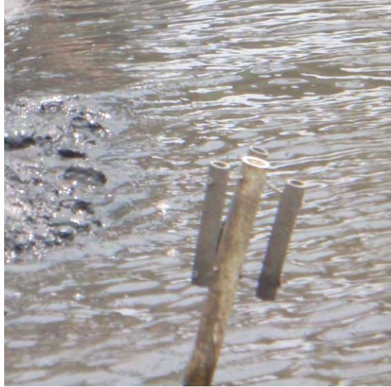
Figure 34. Spat collector used monitor oyster spat at living shoreline site prior to construction, Little St. Simons Island, GA.
