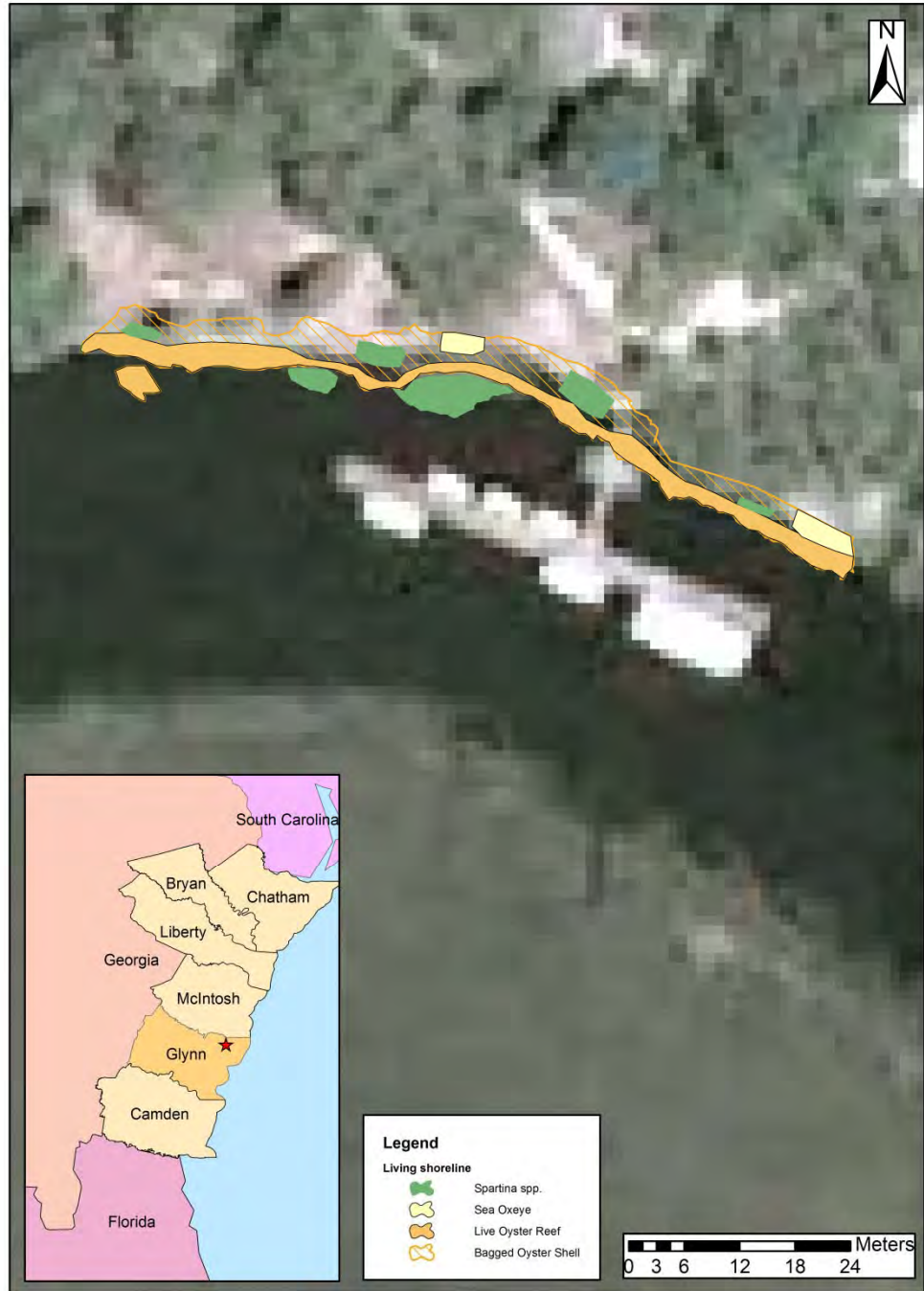
Figure 14. Location of Spartina , sea oxeye, bagged oyster shell, and live oysters at the living shoreline after its construction, Little St. Simons Island, GA.
