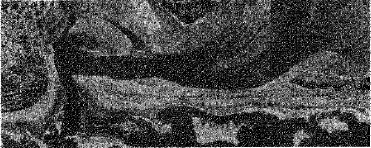
Fig. 3. Aerial photo mosaic of the northern half of Siletz Spit, taken on Feb. 5, 1976, showing erosion embayments on the ocean beach due to rip currents carrying sand offshore.
