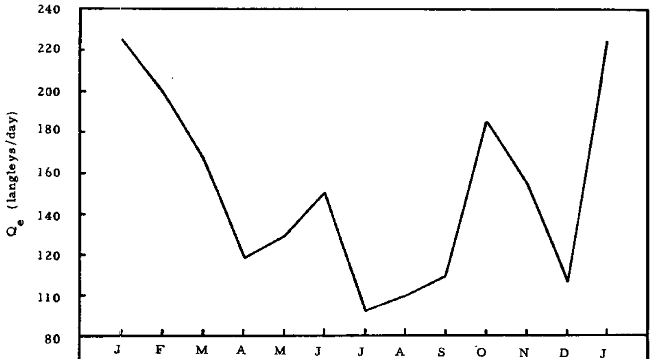
Figure 7-5. Monthly mean values of evaporative flux for the area from the Oregon coastline to 60 nautical miles offshore. In summer the evaporative heat loss is greatly suppressed from its winter maximum due to cooling effect of coastal upwelling. (modified from Lane, 1).
