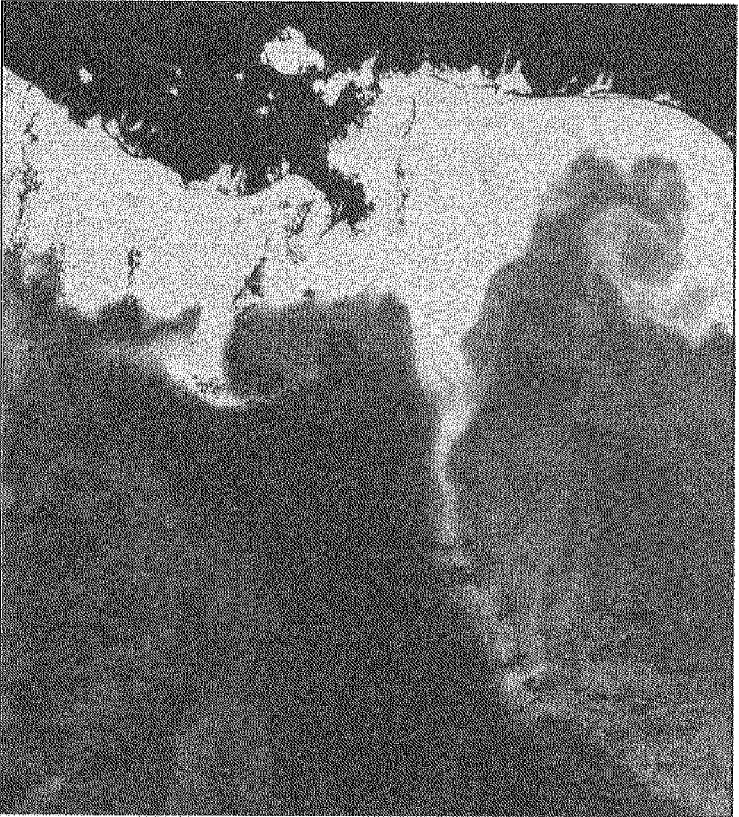
Figure 2. CZCS subscene off the Mississippi Delta from Orbit 4830, October 8, 1979, with dark areas corresponding to low pigment concentrations (chlorophyll a and phaeopigment). The darkened feature is an intrusion of the Gulf of Mexico Loop Current into coastal areas with the entrainment of high pigment concentrations (white) 100–200 km offshore.
