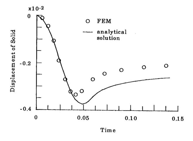
Fig. 4.12 Variation of Displacement of Solid at Surface with Time (Triangular Impulse Loading)
