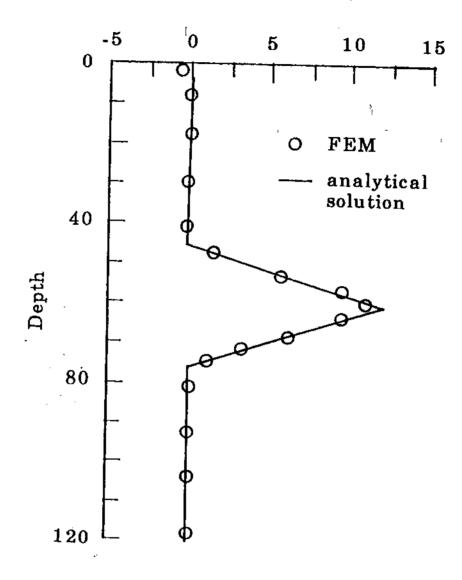
Fig. 4.17 Variation of Excess Pore Pressure with Depth at £ = 0.12 (Triangular Impulse Loading)
