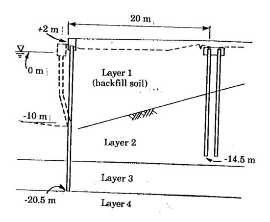
Fig. 5.1 Anchored Bulkhead of Oohama No. 2 Wharf
