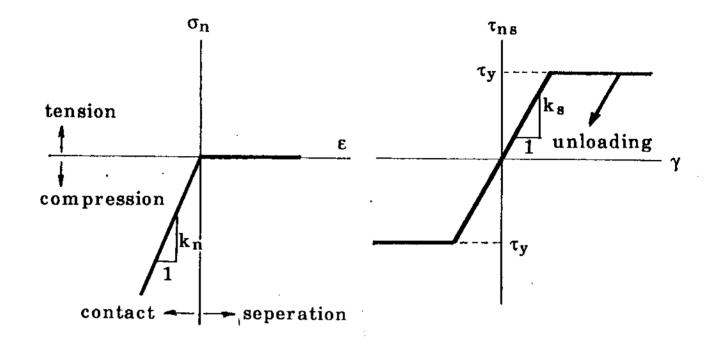
Fig. 2.2 Stress-Strain Relationship at Soil-Wall Interface
