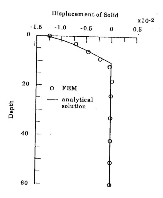
Fig. 4.10 Variation of Displacement of Solid with depth at t=0.06 (Step Function Loading)
