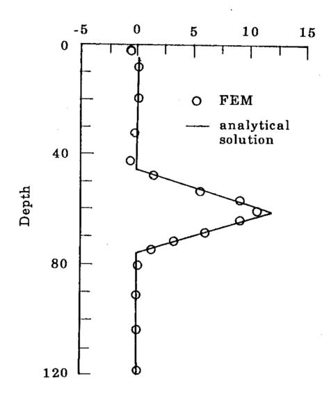
Fig. 4.16 Variation of Total Stress with Depth at t = 0.12 (Triangular Impulse Loading)
