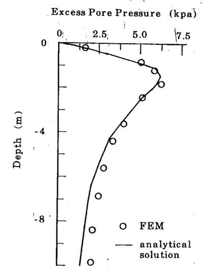
Fig. 4.5 Variation of Excess Pore Pressure with Depth beneath the Loaded Area at T=0.1
