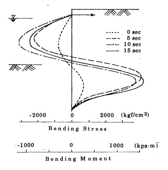
Fig. 5.10 Bending Moment Stresses Induced in Sheet Pile at Various Times
