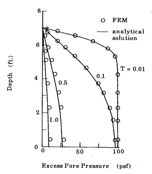
Fig. 4.3 Variations of Excess Pore Pressure with Depth at Various Times (Static 1-D problem)
