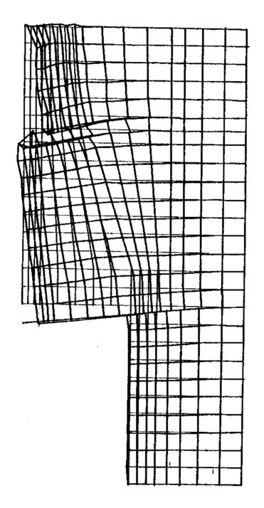
Fig. 5.8 Computed Displacements at 15 Seconds of Earthquake Shaking
