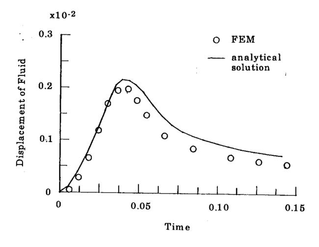
Fig. 4.13 Variation of Displacement of Fluid at Surface with Time (Triangular Impulse Loading)
