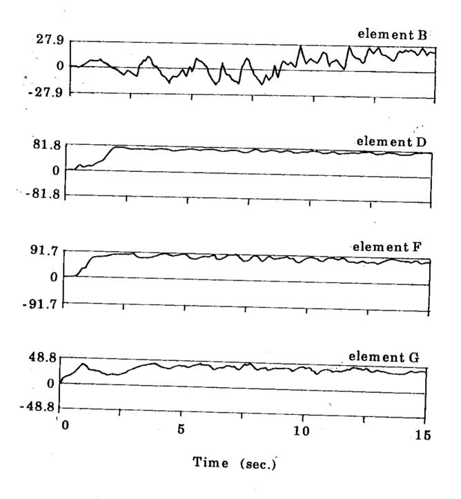
Fig. 5.7 Excess Pore Pressure Time Histories at Various Locations
