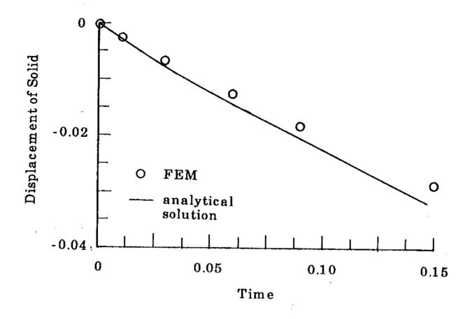
Fig. 4.8 Variation of Displacement of Solid at Surface with Time (Step Function Loading)
