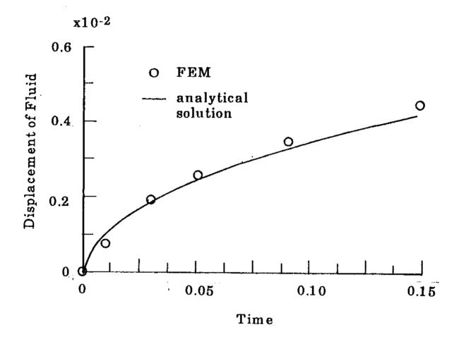
Fig. 4.9 Variation of Displacement of Fluid at Surface with Time (Step Function Loading)
