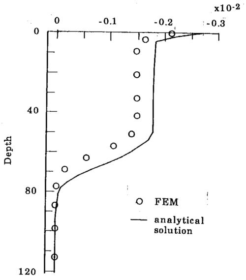
Fig. 4. 14 Variation of Displacement of Solid with Depth at t=0.12 (Triangular Impulse Loading)
