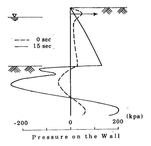
Fig. 5.11 Pressure Acting on Sheet Pile before and at 15 Seconds of Earthquake Shaking
