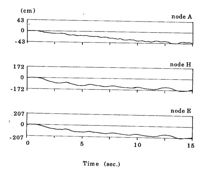
Fig. 5.4 Horizontal Displacement Time Histories at Various Locations
