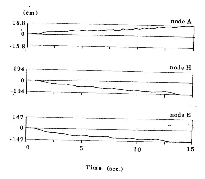
Fig. 5.5 Vertical Displacement Time Histories at Various Locations
