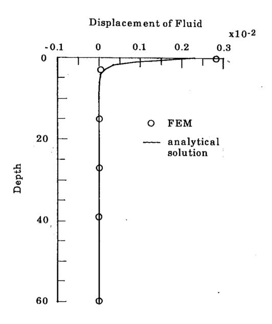
Fig. 4.11 Variation of Displacement of Fluid with Depth at t=0.06 (Step Function Loading)
