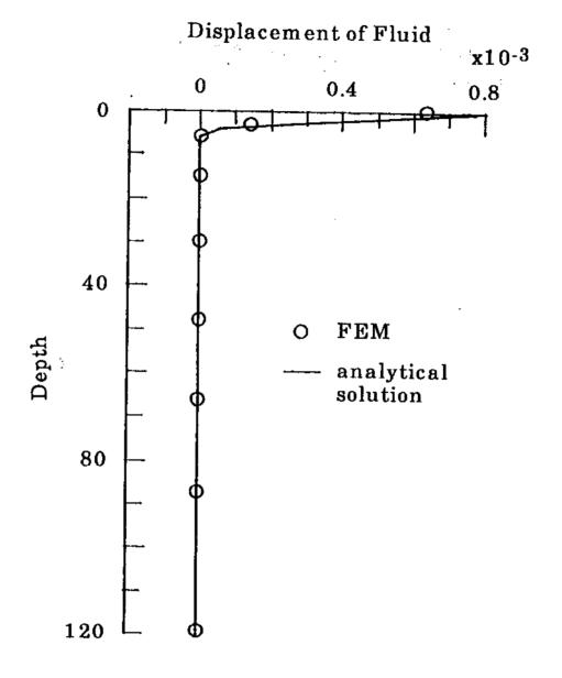
Fig. 4.15 Variation of Displacement of Fluid with Depth at t=0.12 (Triangular Impulse Loading)
