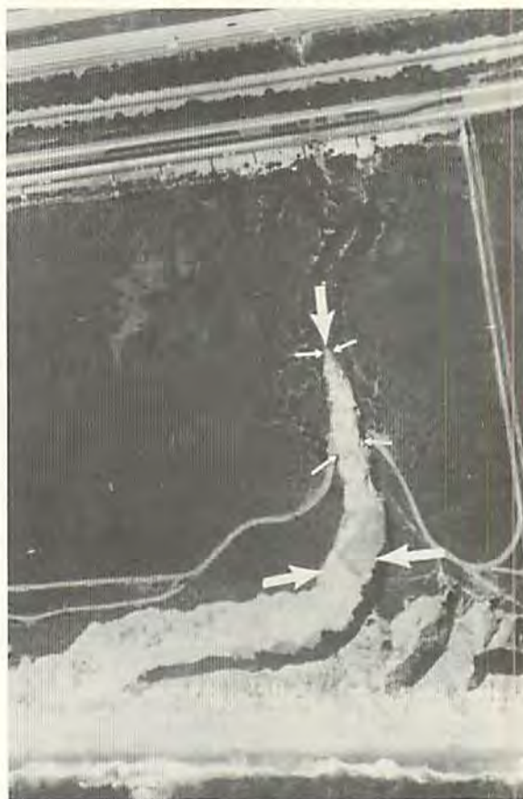
Figure 6. Same area in March 1980. Vertical photo of erosion along the canyon head and subsequent canyon wall collapse. The area located between the large arrows eroded headward approximately 460 feet between January 1968 and March 1980. The area between the small arrows eroded approximately 235 feet on February 20, 1980. (Photo: U.S. Navy)
