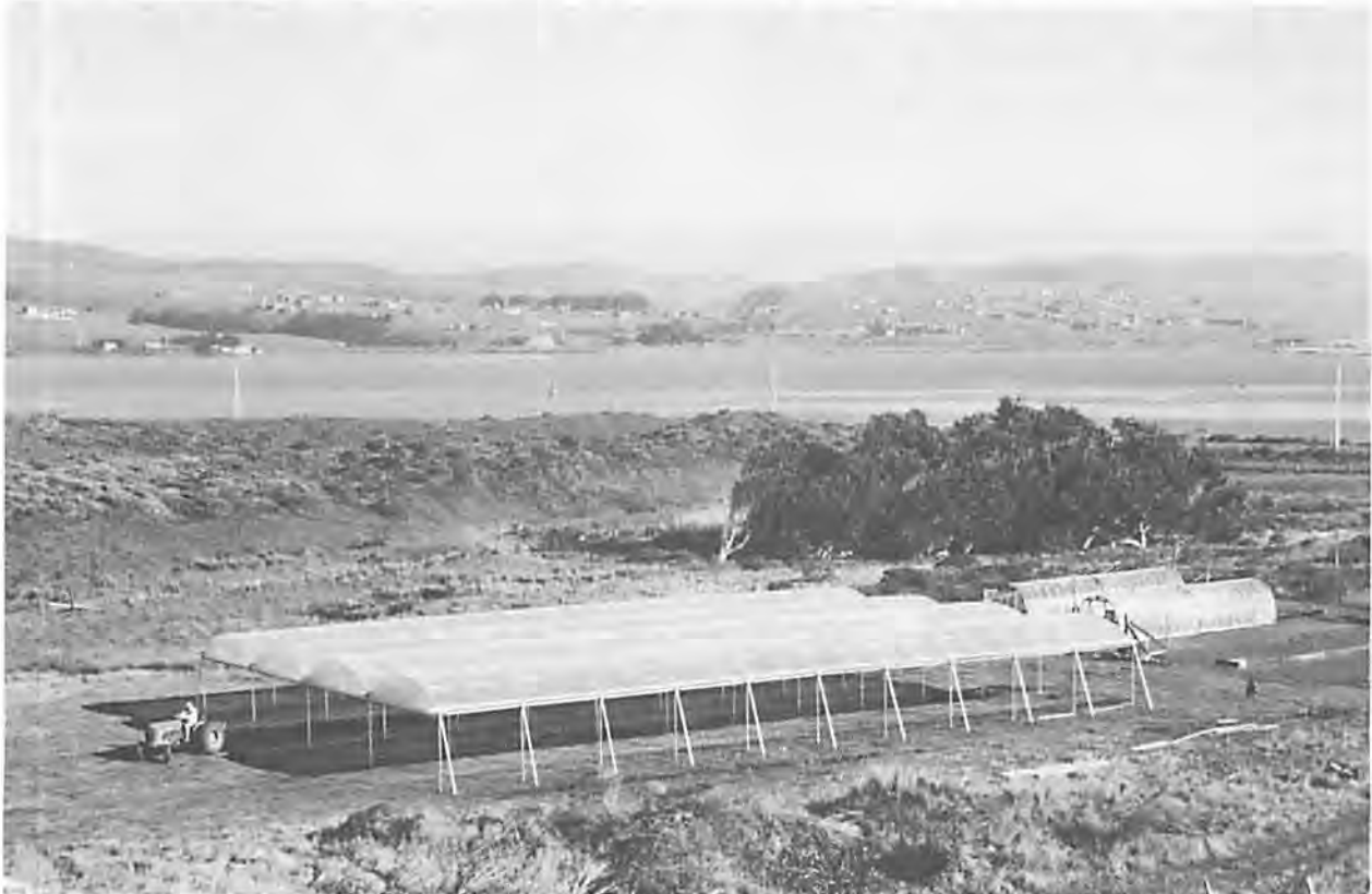
Figure 1. Canopy over an area of stabilized dune sand at the University of California Bodega Marine Laboratory. The canopy covers a 24 x 30 m experimental site for experiments on irrigation of barley and wheat with seawater and dilutions of it. It protects the saline treatments from dilution by rainwater. Partial assistance with the erection of the canopy by International Plant Research Institute, Inc. is acknowledged.
