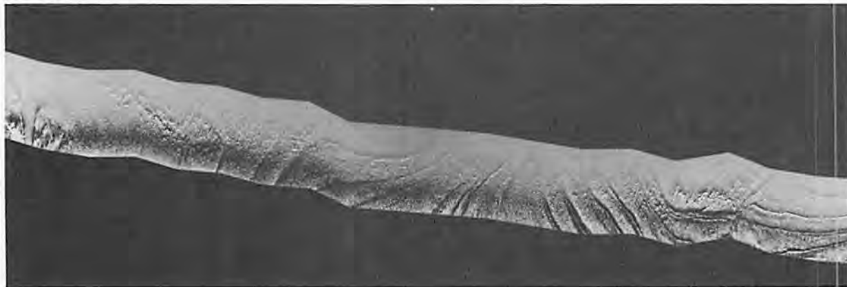
Figure 5. Latest digital sonar sub-image from Anacapa Passage. These data were tape recorded differently from those shown in figure 3. The image includes corrections for both slant range and speed changes. Although the image example has not had a contrast stretch, the improved data quality collected on this November 1979 cruise is evident. This image is western half of a starboard, north-looking run. It is located in approximately the west-central portion of Anacapa Passage, a region of complex folding. Scale: 1:16700. Southwest corner of grid: 34.57 N lat, 31.13 W long.
