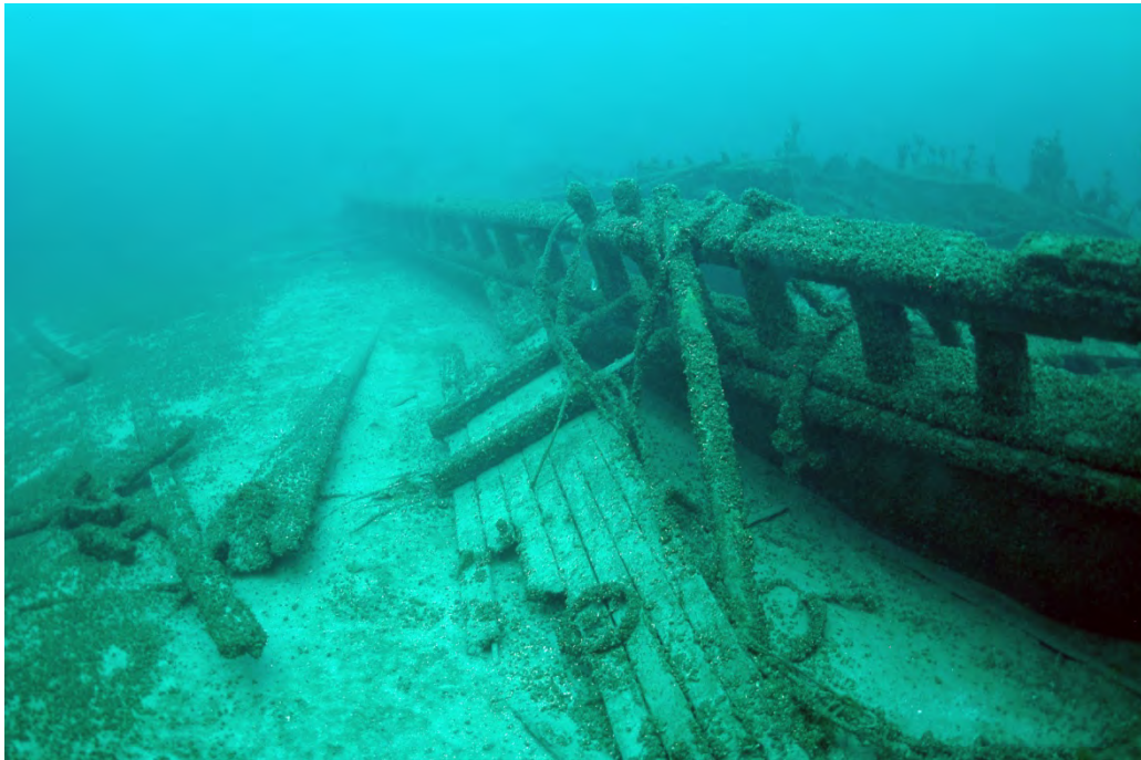
Figure 22. Outside the starboard bow, looking aft. The bulwarks, rubbing strake, and fore chainplates are visible. An inverted section of deck and gaff lie on the lakebed.
