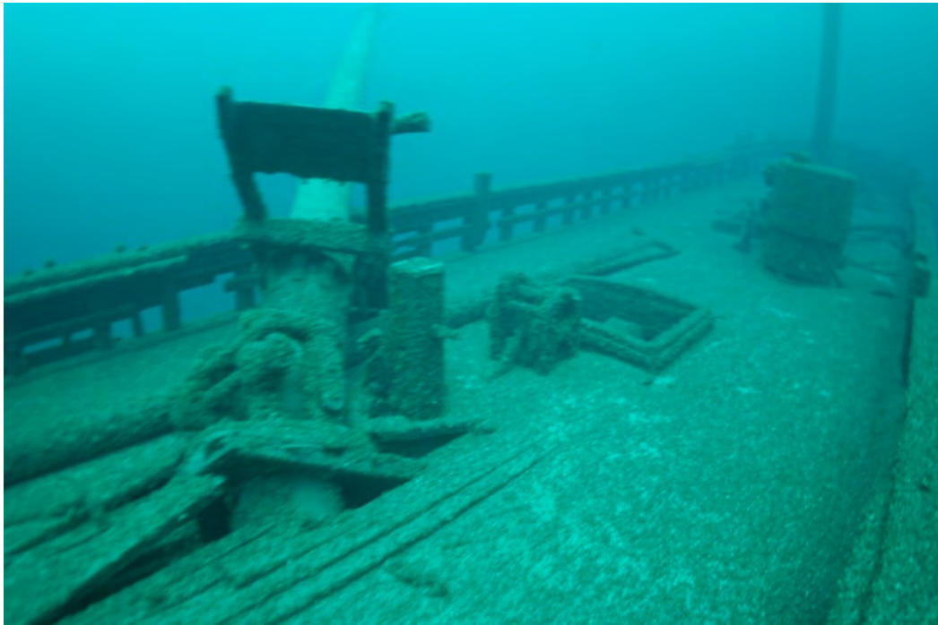
Figure 29. The weather deck, looking forward from near the starboard quarter. The centerboard winch is visible forward of the toppled mast, as well as the donkey boiler forward of the second cargo hatch.
