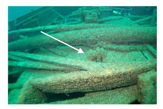
Figure 18. Pulley for aft centerboard chain (denoted by arrow). Note distance to centerboard winch farther aft on deck. Aft cargo hatch is visible at bottom of photo.
