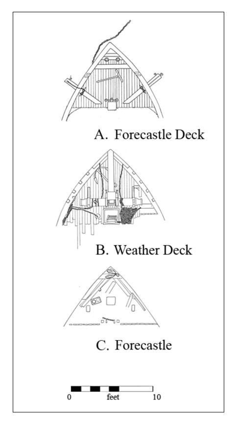
Figure 10. Plan view of deck levels at the bow.
