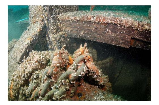
Figure 12. Starboard side of windlass with turns of the anchor chain loosened and tied to allow the windlass to revolve without working the starboard anchor chain. Note the remnants of line protruding from the upper chain links.
