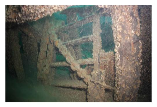
Figure 14. Forecastle ladder, looking aft from the forecastle. Some of the starboard anchor chain spills down the scuttle. The vertical timber on the right is the deck pipe leading to the chain locker.
