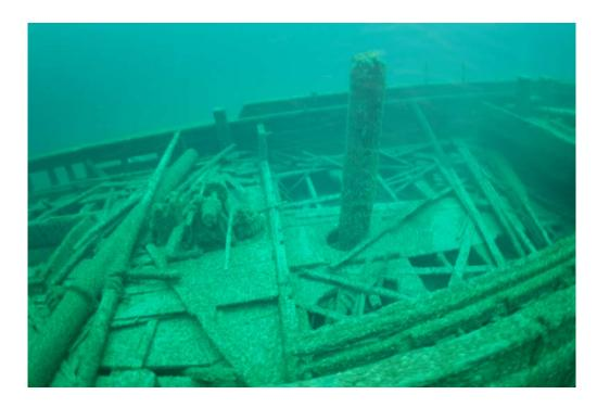
Figure 19. The cabin's former location is visible near the stern. The mizzenmast broke above the cabin roof, and the base of the mast remains in the hull. The bilge pump, centerboard winch, and boom are visible forward of the cabin.
