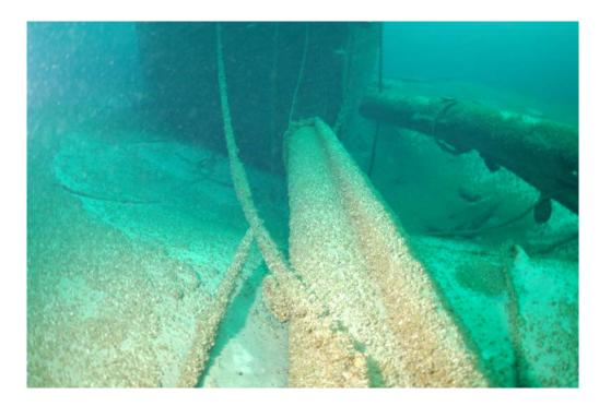
Figure 8. The bowsprit hounding and jib boom lies on the lakebed at the *Rouse Simmons*' bow. A chain bowsprit guy remains attached to the starboard bow. The eye for the inner bobstay is visible beneath the bowsprit guy. Note the large depression in the lakebed around the bow.
