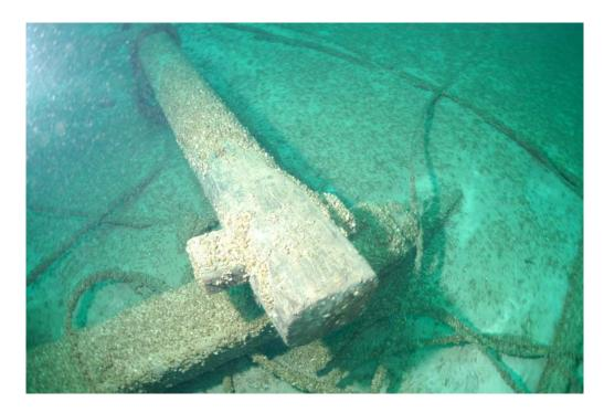
Figure 26. The base of the fore topmast with intact fid. The mast cap visible at the top of the image, which fit onto the tenon at the masthead beneath the topmast.
