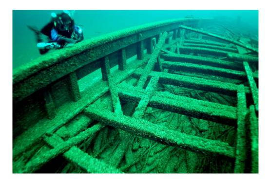
Figure 33. Salt channels carved into the top of each deck beam.
