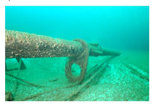
Figure 27. The foremast cap is intact on the fore topmast. The topsail saddle is visible above the mast cap. Topmast shrouds are visible beneath the topmast.
