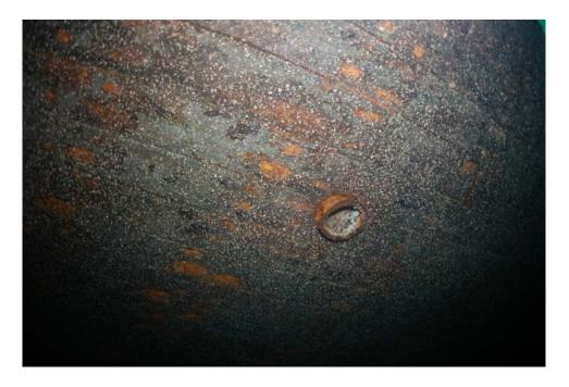
Figure 21. Through-hull fitting beneath the cabin's starboard quarter. Blue hull paint is visible on much of the planking.
