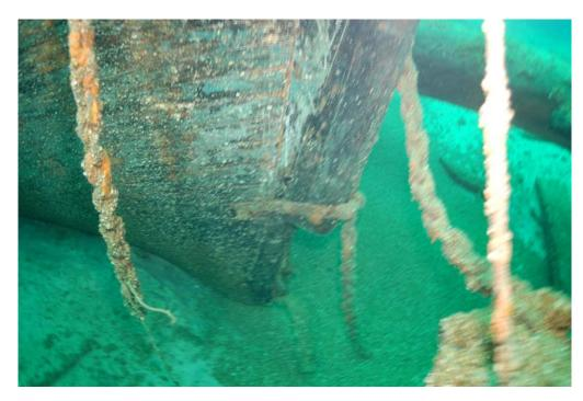
Figure 7. Bow with missing gripe. Iron reinforcing band, encrusted with mussels, is visible hanging below the bobstay plate. Large patches of blue and green hull paint are visible on the stem and outer hull planks.
