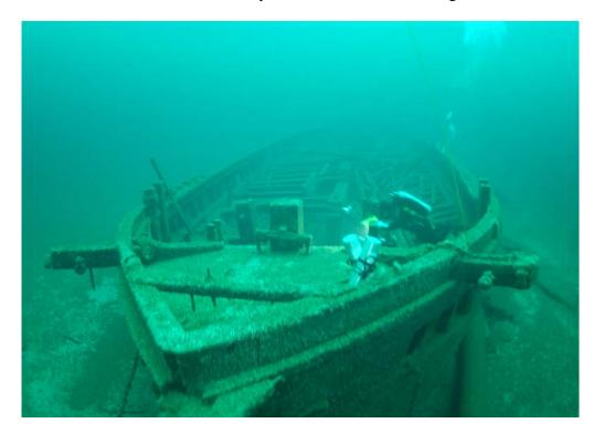
Figure 9. Forecastle deck with pin rack, catheads, samson post, and cross head visible.
