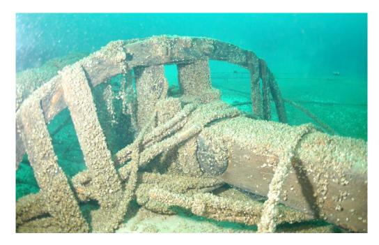
Figure 25. Foremast with top, trestle trees, bolsters, and battens, viewed from above. Note shroud eyes still attached to mast.
