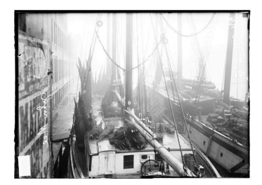
Figure 34. The *George Wrenn*, moored outboard, was used by Captain Schuenemann prior to the *Rouse Simmons* and included a deck house forward of the cabin (Chicago Historical Society DN-0006954f).
