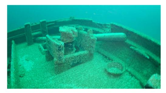
Figure 22. Wheel box and rudder stock. The lazarette hatch is visible between the rudder and the starboard bitts.
