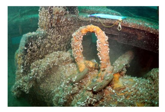
Figure 13. Port side of windlass with norman pin. Note notch in forecastle deck beam. An identical notch is also cut into the beam on the starboard side (see Figure 12).
