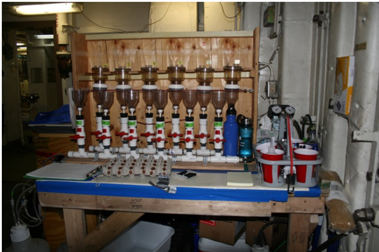
Fig. 1. Onboard laboratory setup for collection and filtering of Arctic seawater samples. Discrete sampling remains critical to understanding ocean chemistry. Photo by J. N. Cross.
