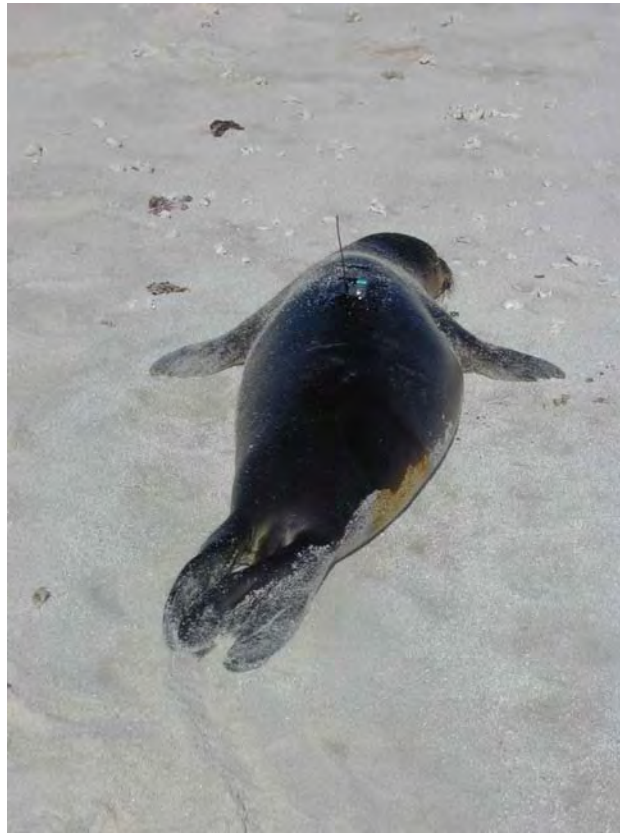
Figure 5. Small SLDR (20,000 transmission capability) glued to hair of juvenile Hawaiian monk seal at Kure Atoll (Photo by B. S. Stewart).
