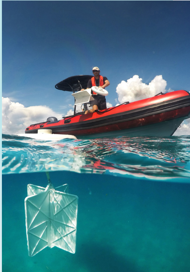
Biodegradable drifters, which float on the water to measure surface currents, wait to be deployed. (CARTHE)
