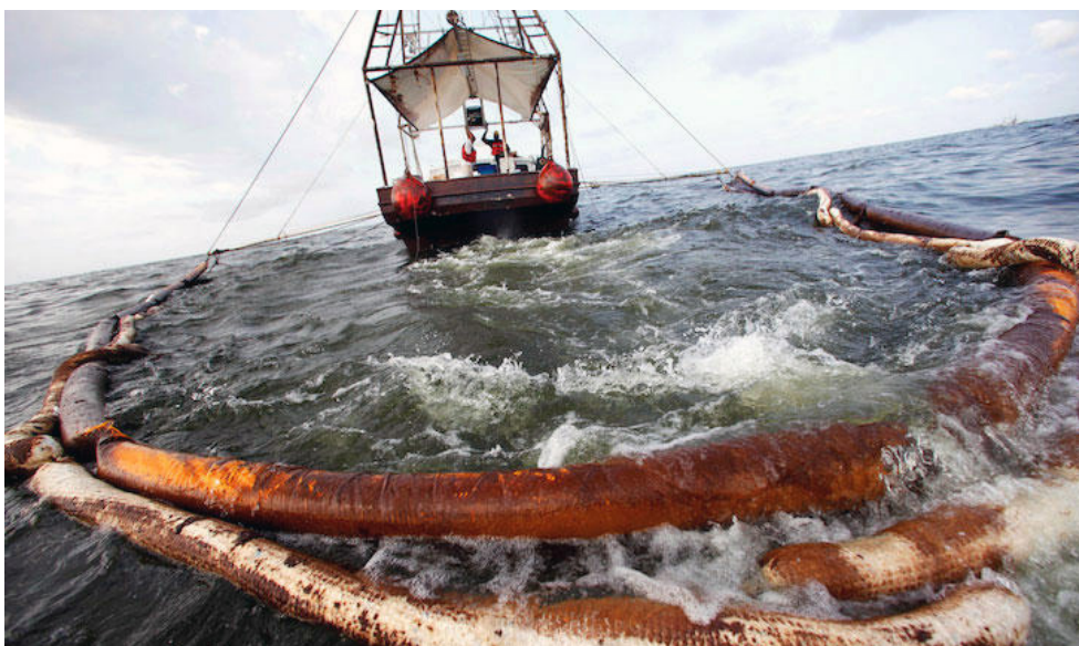
A fishing boat serves as a vessel of opportunity in oil spill response by pulling an oil boom. (National Commission on the BP Deepwater Horizon oil spill)
