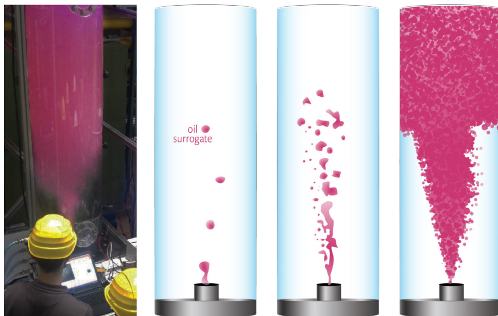
FIGURE 4. To better understand the forces of oil and gas released from the Deepwater Horizon wellhead and how droplets formed and dispersed, scientists generated a variety of scenarios in laboratory experiments using an oil surrogate (droplets dyed pick). (Reprinted from Quigg et al., 2021)
