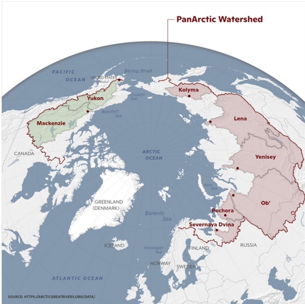
Fig. 1. Watersheds of the eight largest Arctic rivers that are featured in this analysis. Collectively, these rivers cover approximately 70% of the 16.8 million km 2 pan-Arctic watershed (indicated by the red boundary line). The red dots show the locations of the discharge monitoring stations (see Table 2).
