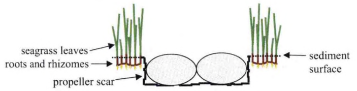
Figure 3. Cross-sectional view of sediment tube deployment into an existing propeller scar.
