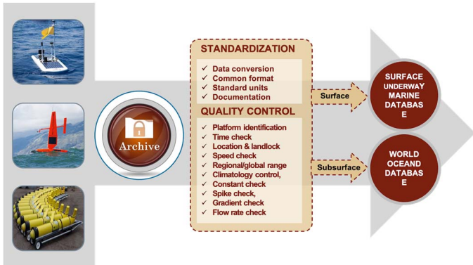
Fig 2. NCEI unmanned maritime system data incorporation workflow.
