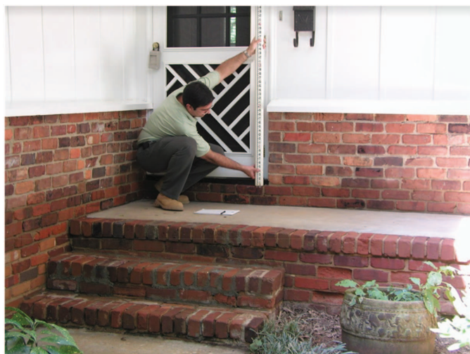
Fig. 7. (Color) Example of flood damage survey for the 2008 flood of record. Damage depths were recorded relative within a structure and are not referenced to a datum. (Image courtesy of Charlotte-Mecklenburg Storm Water Services.)
