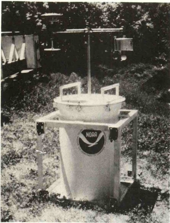
Figure 3. Tatable Tornado Observatory (TOTO) developed by A. J. Bedard, Jr., of the Wave Propagation Laboratory. Sensors located on the cross-arm measure temperature, pressure, wind speed and direction, and corona discharge. The cylindrical container, that forms the stable base of the 400 pound device, houses the electronics, chart recorders and battery. Photo courtesy of Howard Bluestein.
