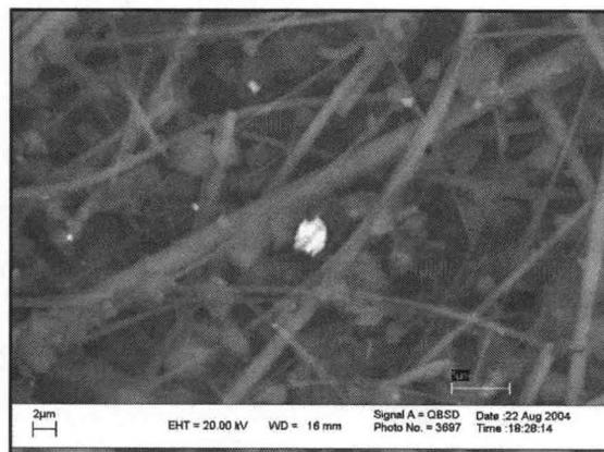
Figure 8. Fe-Cr particle embedded on an E-BAM silica ribbon filter (bright, center).
