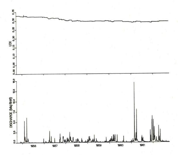
Figure 6.8. LINDRV Results for UZK (Fractional daily upper zone free water withdrawal rate) for Leaf River Data ( $P_0=0.1\%$  initial parameter value,  $v_p=0.2$ ,  $v_u=0.1$ ).
