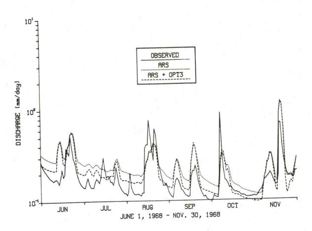
Figure 6.7b. Logarithmic Baseflow Hydrograph for Comparison of ARS and ARS + OPT Parameter Sets.
