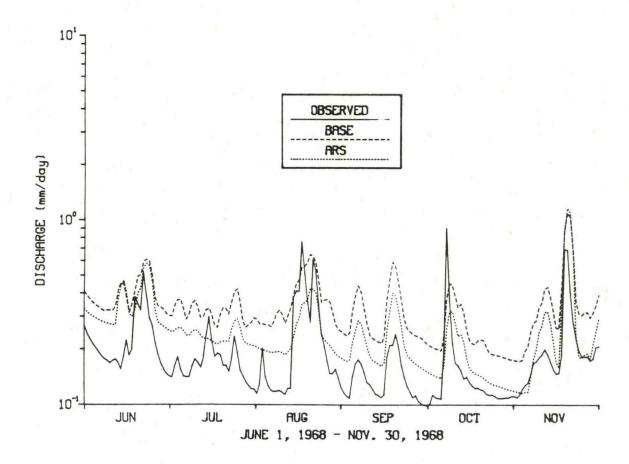
Figure 6.7a. Logarithmic Baseflow Hydrograph for Comparison of Base and ARS Parameter Sets.
