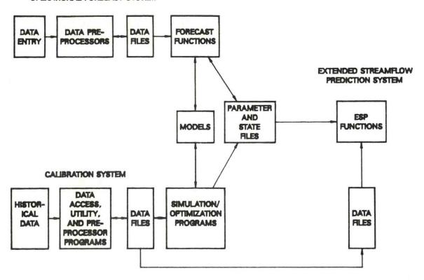
Figure 4.1. Schematic Overview of NWSRFS
