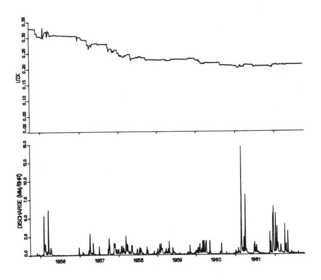
Figure 6.14a. LINDRV Results for 4-parameter Run for Leaf River Data. UZK (Fractional daily upper zone free water withdrawal rate)
