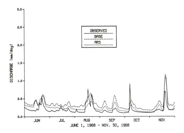
Figure 6.6a. Baseflow Hydrograph for Comparison of Base and ARS Parameter Sets.
