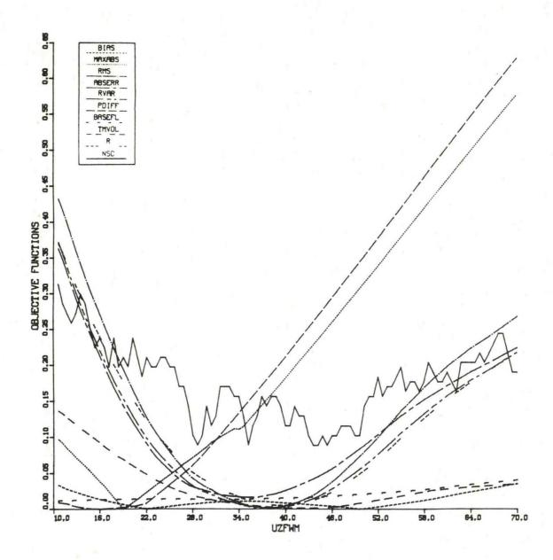
Figure 6.4b. Leaf River Sensitivity Analysis Results for UZFWM (Upper zone free water capacity) following Level II analyses. (Objective function definitions shown in Table 5.2.)
