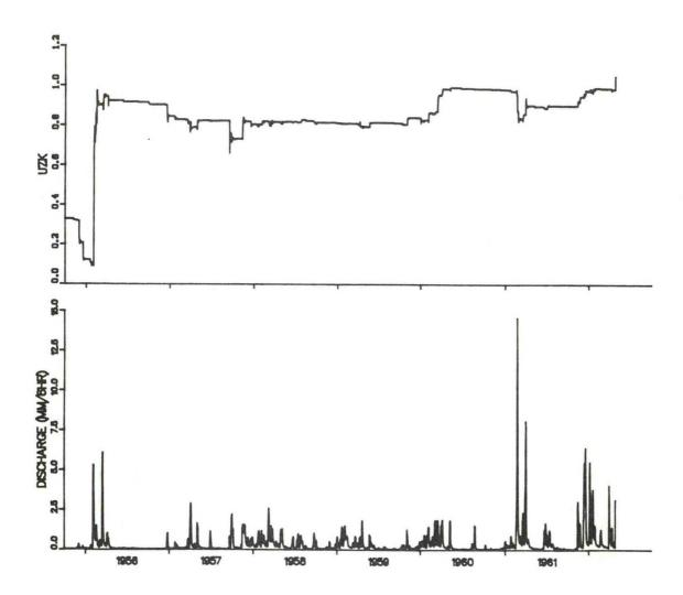
Figure 6.10. LINDRV Results for UZK (Fractional daily upper zone free water withdrawal rate) for Leaf River Data (  $P_0=1\%$  initial parameter value,  $v_r=v_u=0$ ).
