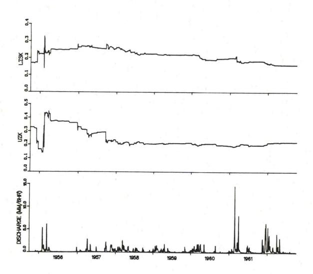
Figure 6.12. LINDRV Results for UZK (Fractional daily upper zone free water withdrawal rate) and LZSK (Fractional daily supplemental withdrawal rate) for Leaf River Data (  $P_0=1\%$  initial parameter value,  $v_r=v_u=0.2$ ).
