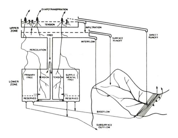
Figure 4.2. Schematic Representation of SAC-SMA Model (from Lawson and Shiau, 1977)
