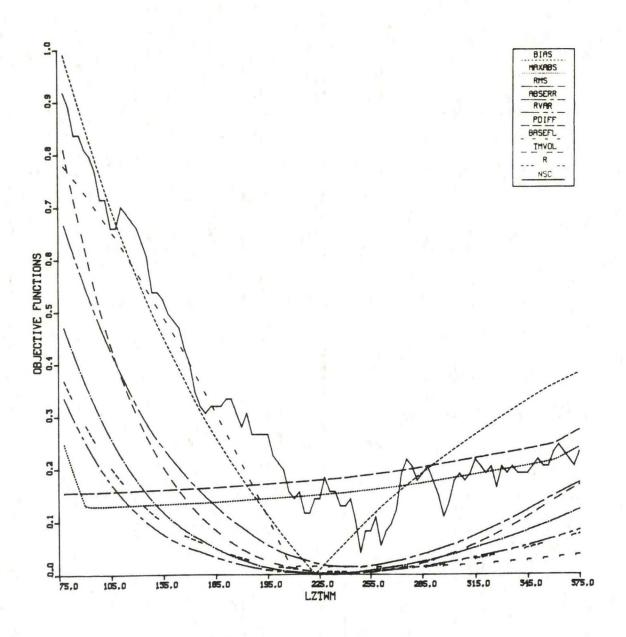
Figure 6.4c. Leaf River Sensitivity Analysis Results for LZTWM (Lower zone tension water capacity) following Level II analyses. (Objective function definitions shown in Table 5.2.)
