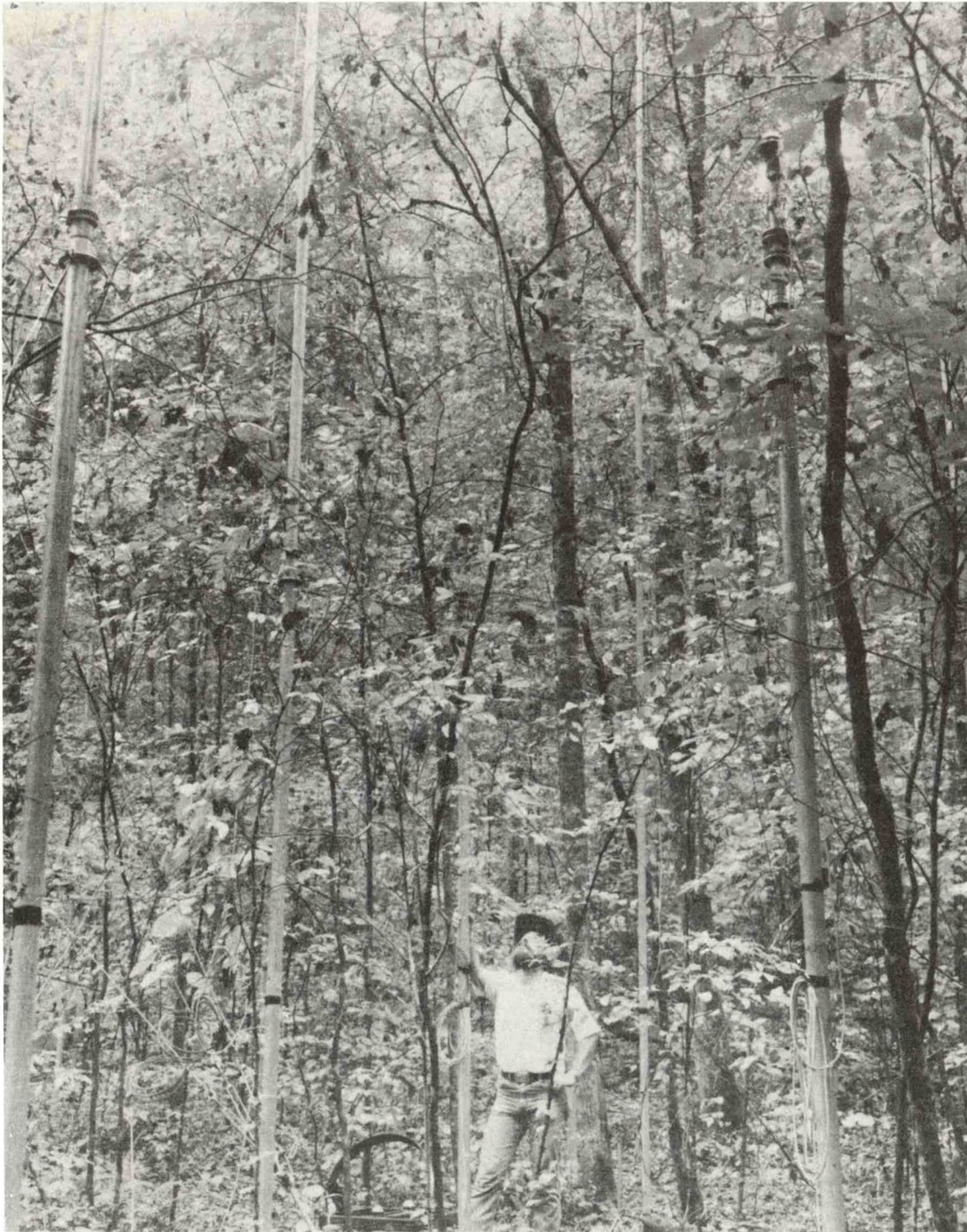
Figure 5: General View of Liriodendron Forest in Summer Showing Telescoping Masts Used to Elevate Solarimeters to 3 and 16 Meter Levels.
