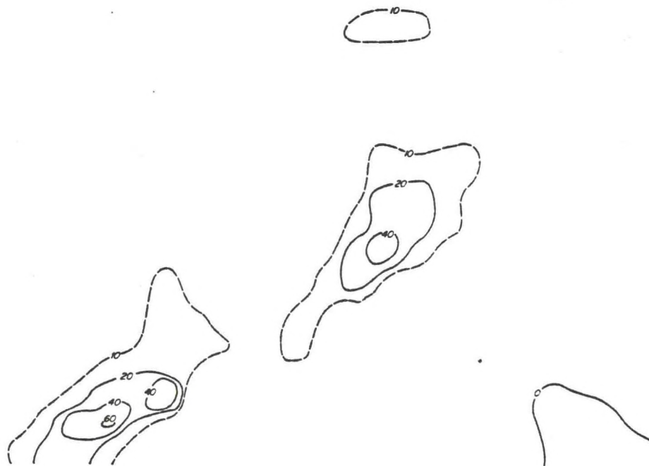
8. Isopleths of calculated \text{SO}_2 concentrations ( \mu\text{g}/\text{m}^3 ) in grid vertical level-3 for October 3, 1974.
