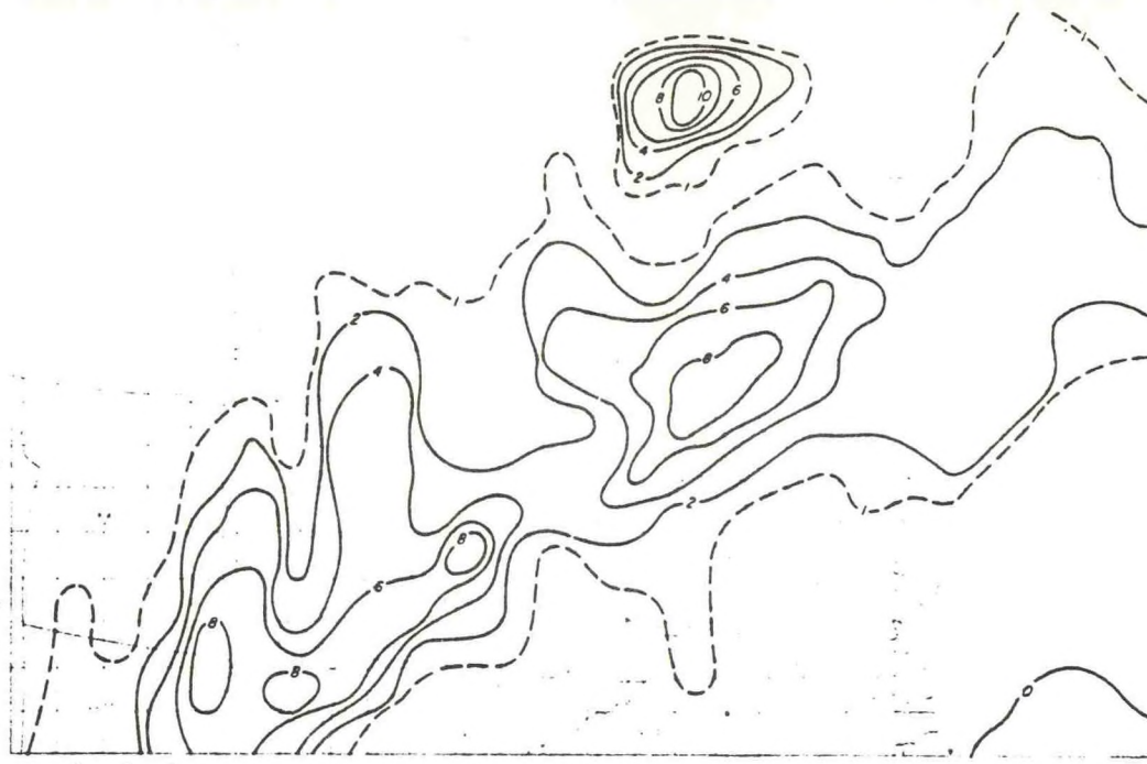
3. Isopleths of calculated \text{SO}_4 concentrations ( \mu\text{g}/\text{m}^3 ) in grid vertical level-1 for October 3, 1974.
