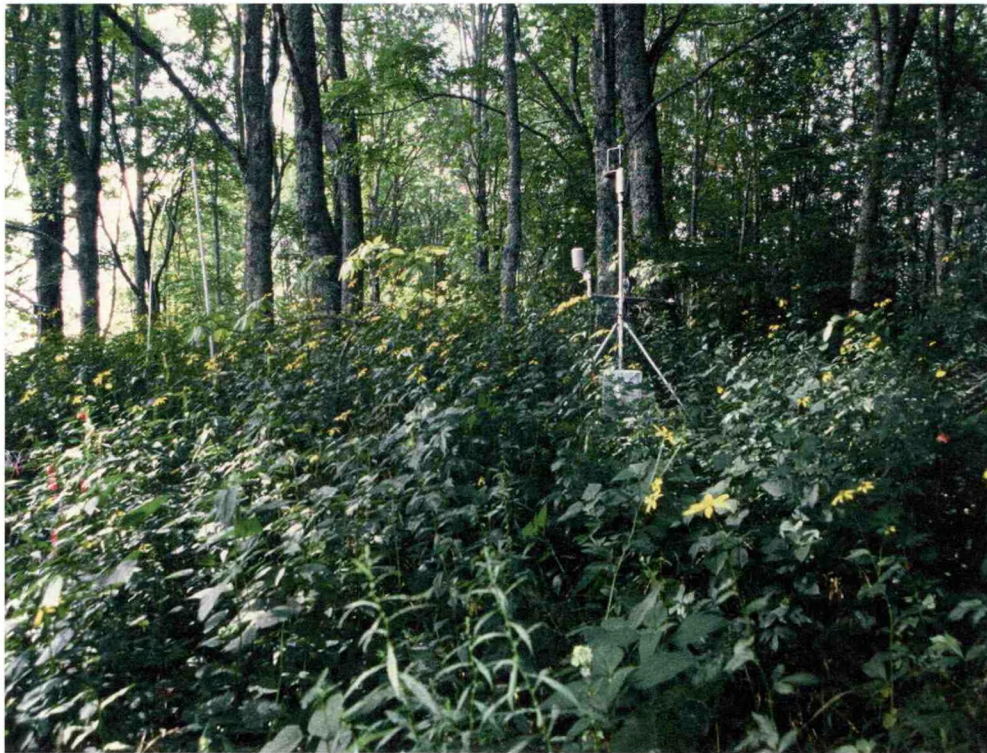
Figure 2. Installation of the meteorological tripod and sonic anemometer at the site inside the forest canopy.
