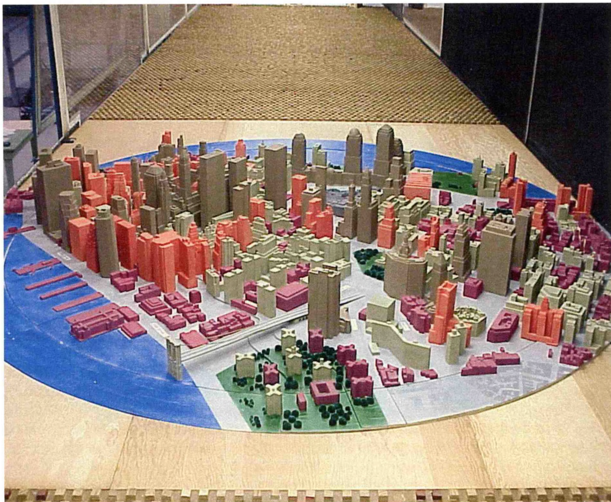
Figure 5. A 1:600 scale model of Lower Manhattan as it appears on the turntable within the Meteorological Wind Tunnel.
