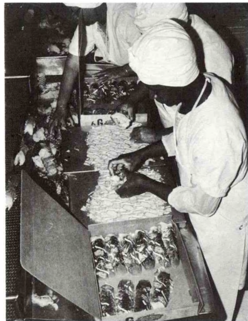
Figure 16.--Tails are wrapped in individual plastic bags and placed in 10-lb (4.54 kg) cartons. (c) Albert J. Stella.
