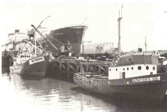
Figure 3.--Landing fish from the San Genaro , an old side trawler, at Montevideo's fishing pier. Note how the freeboard of the Almafuerte , reconstructed in 1973, has been built up. (c) USIS, Montevideo.
