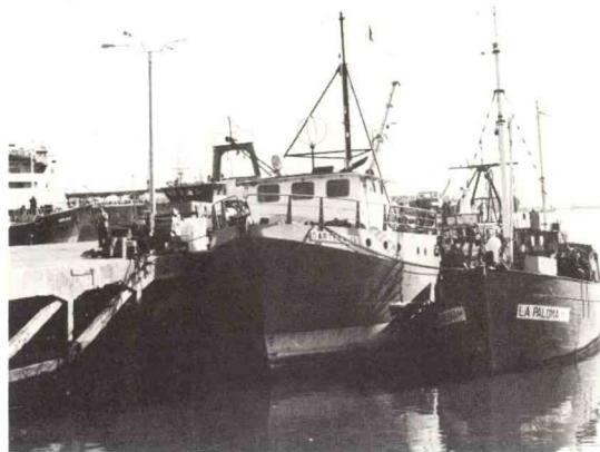
Figure 10.--The Dartesa IV , a new Brazilian built stern trawler, and La Paloma , one of Uruguay's older fishing vessels, tied up at Montevideo's fishing pier. Note how La Paloma's freeboard has been built up. (c) USIS.
