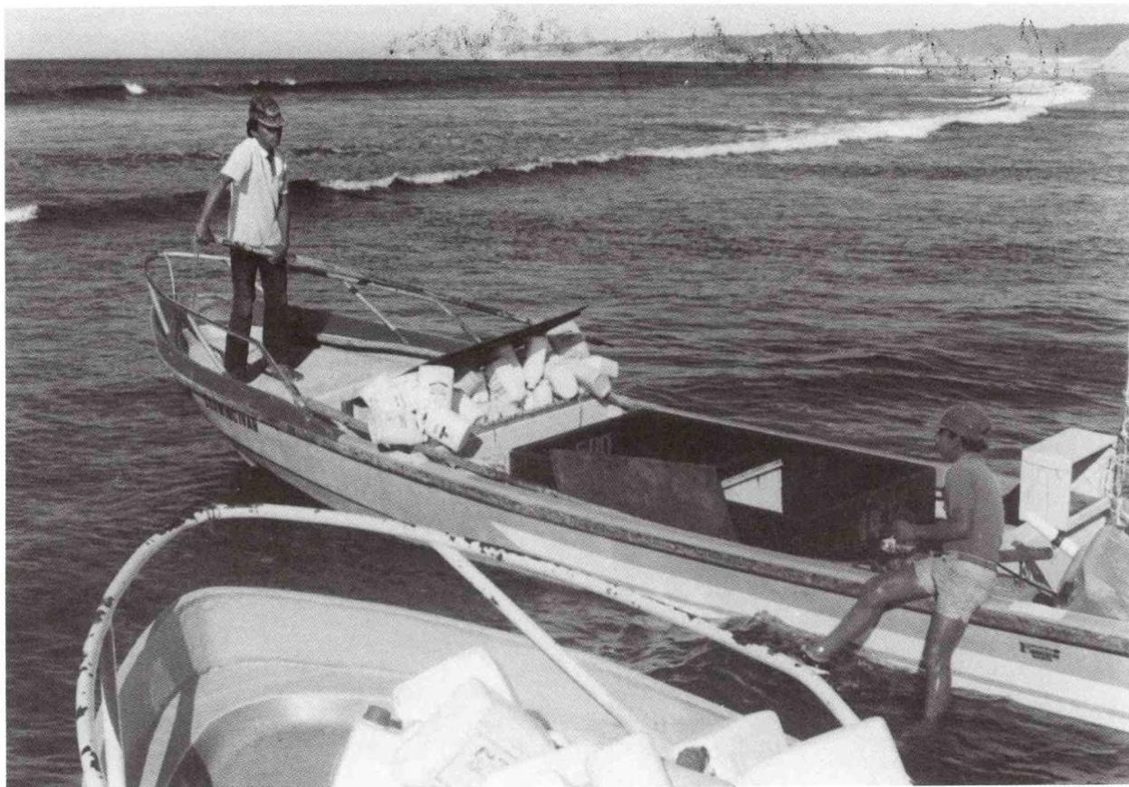
Photo 13.--Typical artisanal fiberglass "panga" or "fibra", which have largely replaced the traditional dugouts. Otto Schwarz
