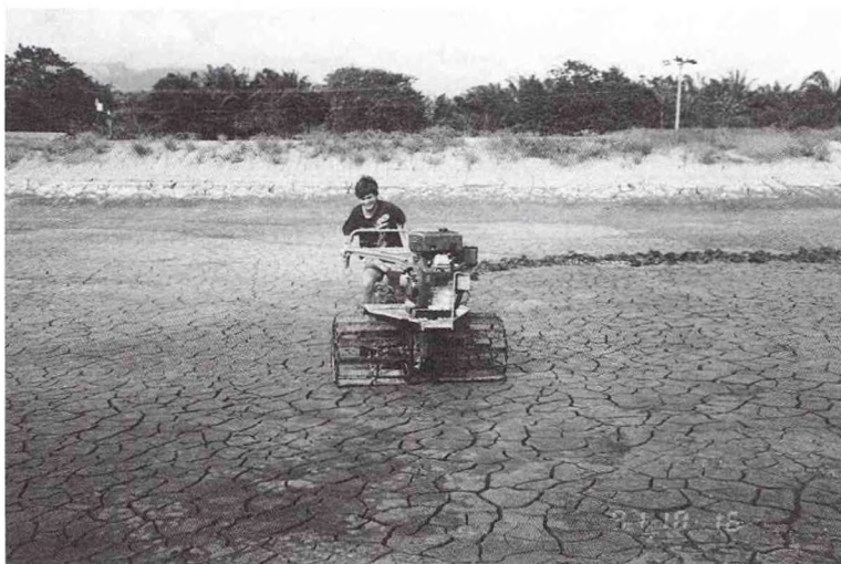
Photo 1. --Costa Rica. Pond bottom maintenance at the Cosechas Marinas farm using a Mud-Wrestler tiller. © C. Lara
