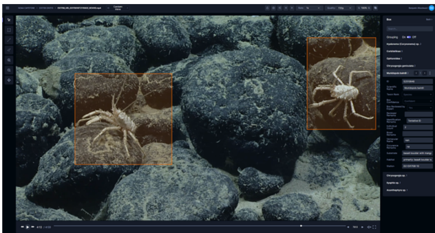
Fig. 4 Video data collected by the NOAA ROV Deep Discoverer during the Musicians Seamount exploration (2017) is displayed in the CVision (Anno)Tator Online tool during an algorithm training exercise. Image courtesy of CVision.
